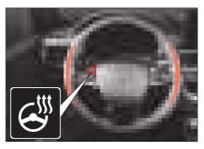
• To activate the steering wheel heater, press the steering wheel heater switch while the engine is running.
