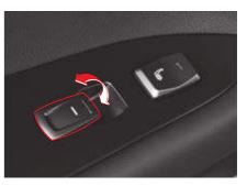
• The window operates only while the Window button is being pressed or pulled.
