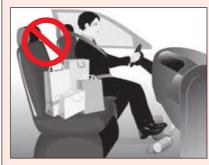
Before driving the vehicle, clean up the area where the brake pedal or the accelerator pedal is operated. If an empty can or an article is present below the pedal, it may obstruct the pedal operation, causing an accident. Be sure to check before driving the vehicle.
