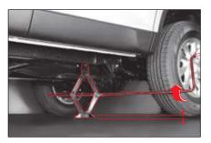
4 Combine the jack, jack extension and the wheel nut wrench as shown in the figure. Raise up the vehicle by rotating the combined wrench clockwise until the tire is off from the ground about 3 cm. 5 Remove the wheel nuts by hands while the vehicle is stationary. Remove all of the wheel nuts.
