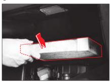
6 Replace it with a new one. Install it with the "AIR FLOW arrow" facing down.
