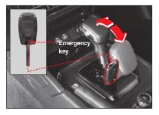
If the gear shift lever cannot be moved from the P (parking) to another position even if the START/ STOP switch is in the ON status and the brake pedal is depressed, move the gear shift lever manually as follows.
