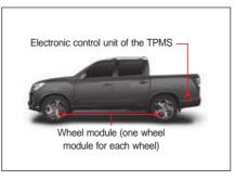
The electronic control unit of the TPMS receives various data including the tire pressure and temperature from the wheel module mounted on each wheel and displays such data on the instrument cluster.
