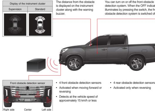
You can turn on or off the front obstacle detection system. When the OFF indicator illuminates by pressing the switch, the front obstacle detection system is switched off.
