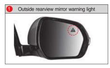
When the outside rearview mirror warning light blinks twice with the START/STOP switch in the ON status or while the engine is running, it indicates that the rear and side warning system is operating normally.
