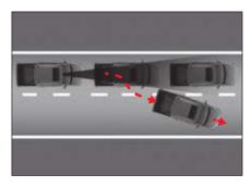
Caution should be taken that if there is a vehicle stopped in front of the vehicle ahead and the vehicle ahead moves out of the lane while your vehicle has been decelerated due to the AEBS operation, the vehicle stopped at the front is not selected as the control target, causing a collision risk.
