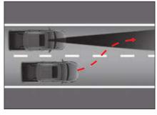
When a vehicle on the next lane changes the lane to the same lane, the vehicle may not be detected until it enters the detection range of the
