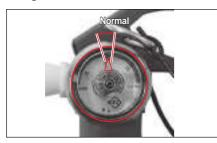
• Check at least once a month if the needle on the pressure gauge of the extinguisher is in the normal range.
