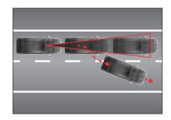
If the front vehicle leaves the lane due to lane change, etc., be careful that there is a risk of collision because the system can not detect another vehicle ahead.
