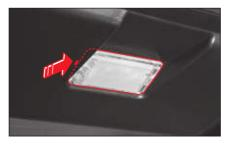
Disconnect the negative battery cable and remove the cover using a flat bladed screwdriver.
