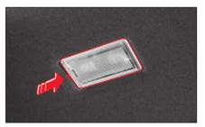
1 Turn the ignition switch OFF, and remove the cover using a flat bladed screwdriver.
