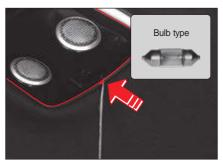
1 Turn the room lamp switch OFF, and remove the cover using a flat bladed screwdriver.
