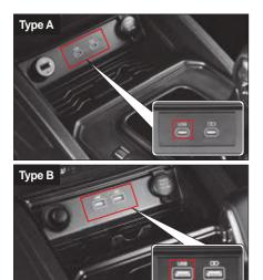
You can charge devices such as a smartphone or tablet PC using the USB charging port.
