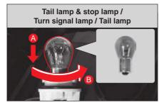
3 Remove the lamp from the removed socket by rotating the lamp in the direction of the arrow (B) while pressing it in the direction of the arrow (A). Rear fog light or Stop lamp
