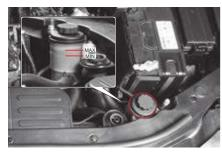
Check the fluid level on a level ground with the engine turned off. The fluid level should be between the MIN and MAX marks on the reservoir cap gauge. If it drops to or below the MIN mark, refill the reservoir with the specified fluid. Only use the specified fluid. The difference between the MIN and MAX marks shows fluctuations of the steering fluid between when it is hot and when it is cold.
