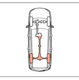
The 2WD (2H) mode is the status for 2WD high speed driving. Use this mode for normal or a high speed driving on a normal road or an expressway.
