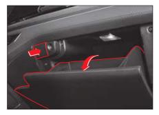
2 Pull the fixing holder on the left side and the right side of the glove box in the arrow direction.
