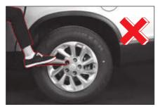
If over tightened, the wheel nuts could be damaged. Do not overtighten the wheel nuts by pressing the wheel nut wrench by foot or using an assist pipe.
