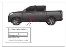
The certification label is attached to the driver's door sill (B pillar).
