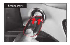
Put the one end of the smart key against the ignition switch and push it while depressing and holding the brake pedal with the gear selector lever in P or N position and. The warning buzzer will stop if it was activated.
