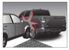
In the event of a side collision, the occupants cannot be protected by the front air bags, so the front air bags may not inflate.
