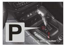
1 Turn the ignition off with brake pedal depressed and gear selector lever in the P position.
