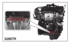
**Gasoline Engine:** The engine number is stamped on the bottom surface of the cylinder block behind the intake manifold.
