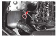
If the vehicle is operated in very dusty or sandy areas, replace more often than at the usual recommended intervals. If it is dirty, shake the element to remove dust. Clean the inside of the air cleaner housing and cover with a damp cloth.
