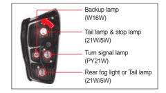
2 Turn the socket counterclockwise to remove the it.
