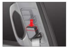
2 Release it at the desired position. The seat belt holder is secured.
