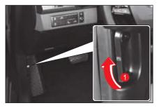
2 With the engine hood lifted slightly, push the engine hood fixing lever (2) in the arrow direction.
