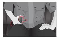
1 Pull out the latch plate at the bight of the seat.
