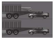
Your attention is always required while driving behind a vehicle carrying cargo longer than the cargo bed or with high ground clearance because the AEBS may not work properly.
