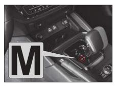
You can shift the gear manually (1st~6th) just as a manual transmission by moving the gear shift lever from the D (driving) position to the M (manual) position.
