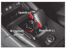
You can shift the gear by pushing or pulling the manual gear shift lever from the M (manual) position.
