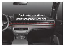
Mood lamps are always activated when any door is open, the ignition is turned on, or switch is turned on, as long as they are set to on.
