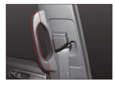
The grip handle is installed at the front of side of rear seats for convenience at the time of getting in and out of the vehicle.
