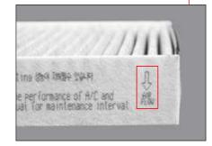
7 After replacing it, install it in the reverse order of A/C filter removal.
