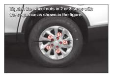
7 Then mount the spare tire and temporarily tighten the wheel nuts until the spare tire wheel is no longer loose.
