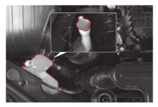
Frequently check the washer fluid level and add the specified product as needed.
