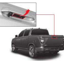
To open the tailgate, pull the lever to unlock the tailgate and lower it slowly with both hands. After loading, raise and close the tailgate.
