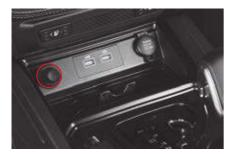
To operate the cigarette lighter, press it in all the way down. When it becomes heated, it automatically pops out and is ready for use.
