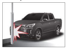
In the event of a collision with a narrow object such as a street light, utility pole or tree, the degree of impact applied to the sensor may not be enough, so the air bag may not inflate.
