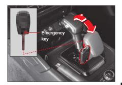
2 Shift the gear selector lever to the N position after pressing the lever lock release button with the brake pedal depressed.
