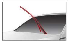
Press the wiper blade retainer (1) and pull the wiper blade out in the arrow direction (2).
