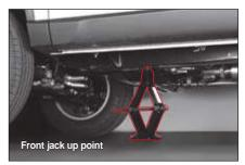
3 Place the jack directly under the jack-up points so that the top of the jack contacts the vehicle at the jack-up point.
