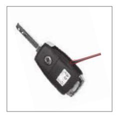
1 Remove the cover at the back side of the smart key using a smallest flat-bladed screwdriver, taking care not to scratch the cover.
