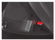
4 Remove the A/C filter cover by pressing the right side of the A/C filter cover.
