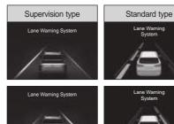
When only one lane line is detected while the vehicle is being driven at 40 km/h or more, the corresponding lane marker on the display turns green.
