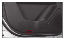
When you open the door, the lamp turns on, and when you close the door, the lamp turns off.
