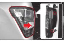
Disconnect the battery (-) terminal and remove the two mounting bolts (10mm) for the rear combination lamp. Pull the lamp assembly in the direction indicated by the arrow in the picture to disconnect the connector and detach the lamp.
