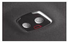
Pressing the center room lamp switch turns on the center room lamp. Pressing the switch again turns off the center room lamp. The center room lamp comes on when the door is opened regardless of the center room lamp switch operation if the door coupled switch is pressed in.
