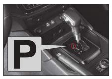
Select this position for parking the vehicle, starting or warming up the engine, or stopping the vehicle for a long period of time.
