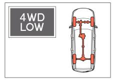
Use the 4WD LOW (4H) mode when the maximum traction power is necessary.
