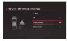
Go to Driving Assist Setting → Blind-Spot Collision Assist → Blind Spot Detection & Collision Assist → Enable Collision Warning in (User Settings) in the instrument cluster and tick the check box.
