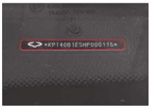
The VIN is stamped on top of the instrument panel.
