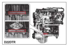
**Diesel Engine:** The engine number is stamped on the bottom surface of the cylinder block behind the exhaust manifold.
