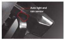
The auto light sensor is integrated with the rain sensor.
