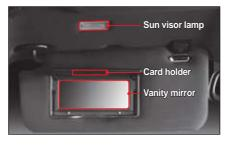
When you pull the sun visor down and open the mirror cover, the lamp turns on.
