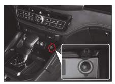
An auxiliary power outlet for extra electrical devices is installed. This power outlet supplies power when the ignition key is in the "ACC" or "ON" position.
