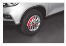
Chock the front and rear of the wheel diagonally opposite to the wheel being changed.
