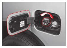
7 Hang the fuel inlet cap on the holder mounted inside the fuel inlet cover.
