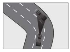
A vehicle on another lane may be detected, affecting the speed. Check the front road and driving conditions and adjust the vehicle speed directly by depressing the brake pedal if necessary.
