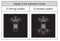
When the obstacle detection sensor is abnormal, "?" is displayed for the relevant sensor. If this message is display on the display of the instrument cluster, have your vehicle checked and serviced at a nearby KG Mobility authorized service center.
