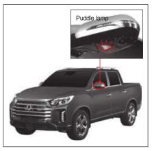
The welcome light is the function that operates the puddle lamp and the door handle lamp (DRL & Low beam: A type only) in order to increase safety and visibility at night.
