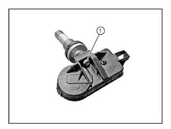
Remove the fixing bolts (1) of the tire pressure sensor with a T10 screwdriver bit to separate the tire pressure sensor from the valve.
