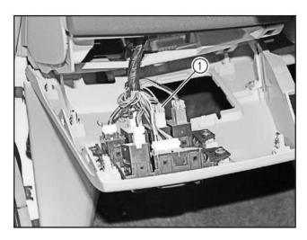
Press the locking clip of connector and disconnect the ESC OFF switch connector (1).
