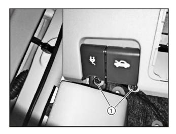
Remove the fixing bolts (1) of the charging hole cover handle and the drive motor compartment handle with a Phillips screwdriver.
