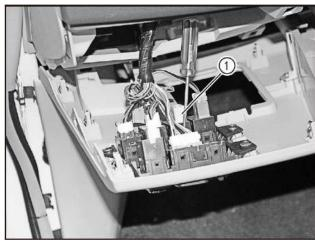
Pry open the locking clips on both ends of the ESC OFF switch with a slotted screwdriver to remove the ESC OFF switch (1).
