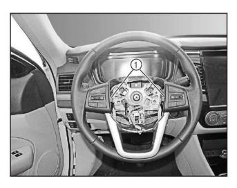
Press the locking clip of steering wheel buttons connector to disconnect the steering wheel button connector (1).
