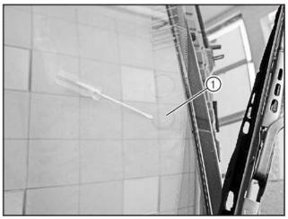
Insert the solar sensor (1) into the instrument panel.
