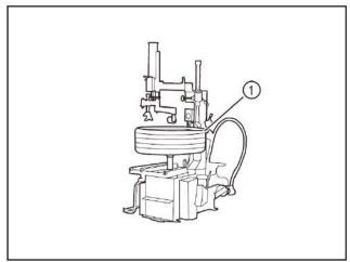
• Refit the tires with a tire changer (1). (Refer to "Removal and Refitting of Battery").
