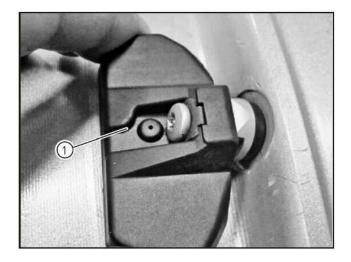
Align the tire pressure sensor (1) with the mounting holes of the valve to refit it in place. By applying pressure (you can hold the sides of the sensor by hands), the gasket on the valve is tightly fitted to the rim mounting plane.
