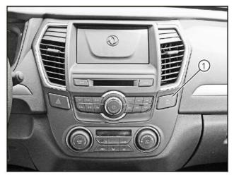
For the model with MP3 radio, Please refer to "Removal and Refitting of Hazard Warning Lamp Switch" for removal and refitting of AVAS switch (1).
