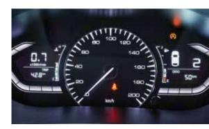
The digital RPM screen provides you with all the vehicle information without letting go of the steering wheel. It indicates fuel consumption pattern, distance to empty, trip meter, gear shift reminder for manual drive and all door open indicator to ensure safety and ease of mind.
