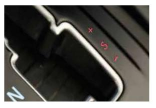
Triptronic sports mode conveniently gives the gear shifting control to the driver.
