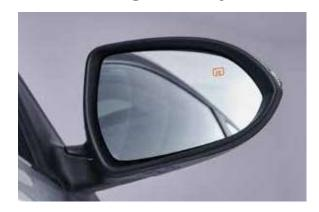
The powered adjustable outside rear view mirrors (ORVM) are equipped with a heater defroster to provide better visibility in rainy and foggy weather.
