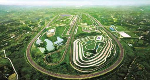
CHANGAN TEST TRACK CHONGQING DIANJIANG DISTRICT Covering an area of over 2,240,000 m², having 12 test tracks, including high speed, brake and performance testing tracks.
