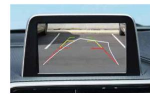
The dynamic reverse guidelines trace the vehicle's trajectory and assist in steering conveniently without colliiding into obstacles.
