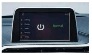
Pakistan's 1st sedan with Tire Pressure Monitoring System (TPMS) offers tire pressure on the driver's screen. The system provides alerts to the driver before the tire deflates to ensure safety of passengers.
