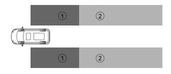
If the turn signal on the corresponding side will be turned on, the lane change assistance system warning lamp will change to flash.
