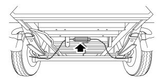
Electrical parking brake (EPB) is in the middle and up of the rear axle of the vehicle. If electrical parking brake (EPB) cannot be released via normal operation, it can be released as per the following methods.
