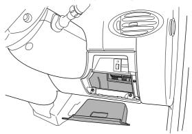
Fuses in main fuse box can be identified with labels printed on the back of fuse box cover.
