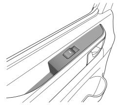
Note: The power windows will only operate when the ignition switch is turned to "ON".
