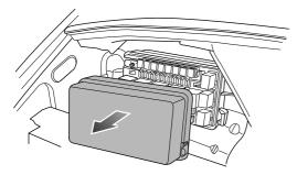
Fuse is accessible just by removing auxiliary fuse box cover. Fuses in auxiliary fuse box can be identified with labels printed on the back of fuse box cover.
