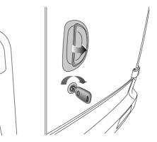
Then pull the spring lock lever on the left hand door to open the left hand tail door.
