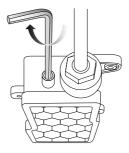
4 Install the hexagon nut (1), and socket head wrench and on-board tool kit will be put away.
