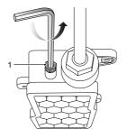
3 Insert the socket head wrench into emergency release port, which will be rotated by clockwise until the vehicle can be pushed from the rear end of the vehicle (in general, the parking can be loosened after 100 circles).
