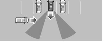
Note: The function of vehicle detection during reversing can be activated only when the speed of target vehicle is 10 to 30 km/h and the speed of your vehicle is less than 10km/h.
