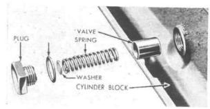
FIG. 31-OIL PRESSURE RELIEF VALVE
