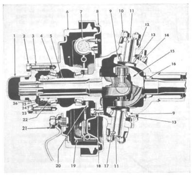
FIG. 236—FRONT STEERING KNUCKLE (With Spicer Universal Joints)
