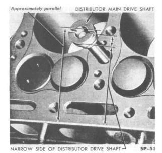
FIG. 93—CORRECT POSITION OF DISTRIBUTOR MAIN DRIVE SHAFT
