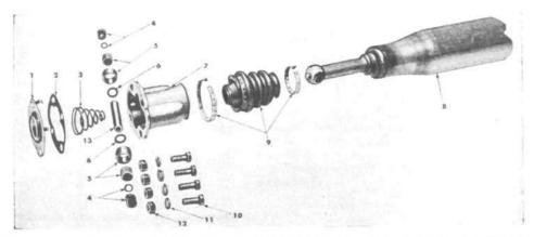
FIG. 220—PROPELLER SHAFT AND UNIVERSAL JOINT—BALL AND TRUNNION TYPE
