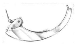
FIG. 305-DOOR HANDLE ADJUSTMENT
