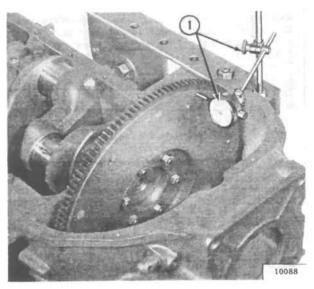
FIG. 79—CHECKING FLYWHEEL RUN-OUT
