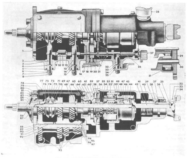
FIG. 202-TRANSMISSION AND OVERDRIVE
