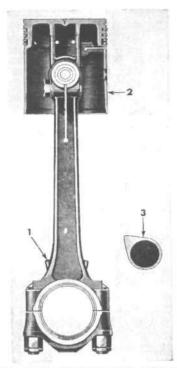
FIG. 119-CONNECTING ROD AND PISTON
