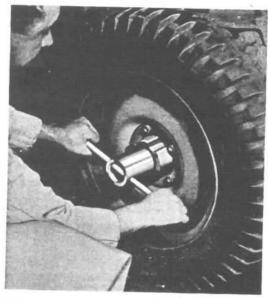
FIG. 229-WHEEL BEARING NUT WRENCH
