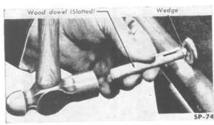
FIG. 32—REMOVING OIL PRESSURE RELIEF VALVE WITH WEDGE
