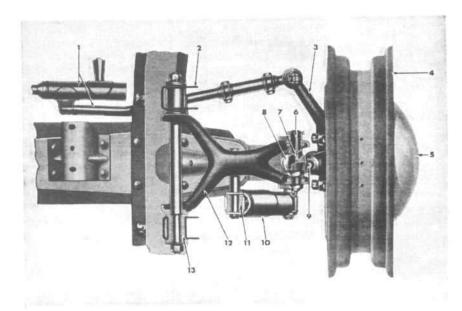
FIG. 237-PLANAR FRONT SUSPENSION-TOP VIEW
