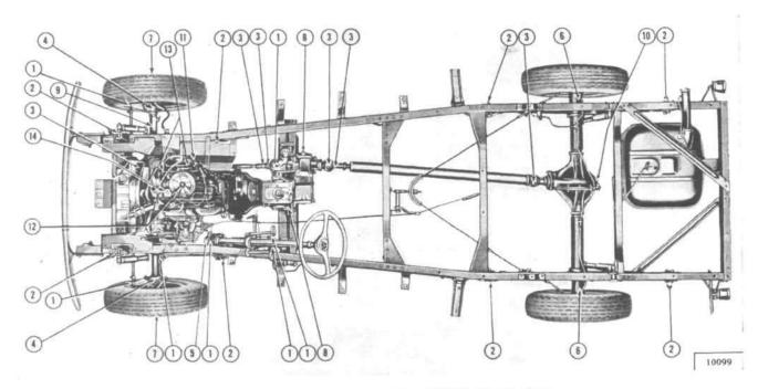
FIG. 6-LUBRICATION CHART - MODEL F4-134 4WD
