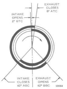
FIG. 89-VALVE TIMING-LATE L6-226 ENGINES
