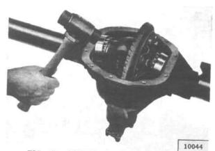
FIG. 264-INSTALLING DIFFERENTIAL
