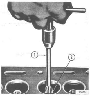
FIG. 68-REAMING VALVE GUIDE
