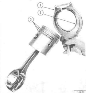
FIG. 43-INSTALLING RINGS ON PISTON
