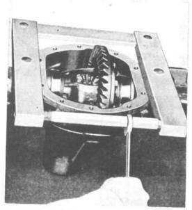
FIG. 244—DIFFERENTIAL CARRIER SPREADER
