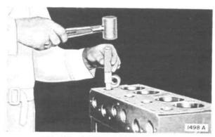
FIG. 101-VALVE GUIDE DRIVER
