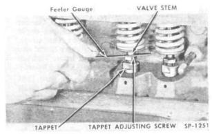
FIG. 95-CHECKING VALVE CLEARANCE
