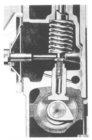
FIG. 94—CAMSHAFT, TAPPET AND VALVE
