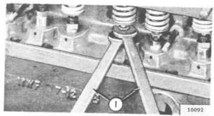
FIG. 96-VALVE TAPPET ADJUSTMENT
