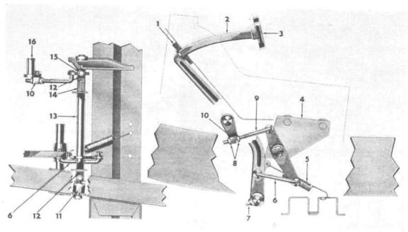
FIG. 172-CLUTCH CONTROL-L6-226 MODELS
