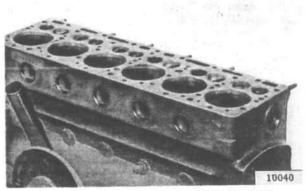
FIG. 80-CORE HOLE EXPANSION PLUGS
