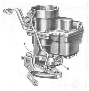
FIG. 131—CARBURETOR FAST IDLE
