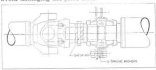
FIG. 315-SPICER PROPELLER SHAFT
