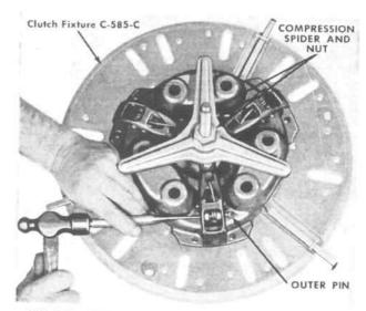
FIG. 178—DISASSEMBLING ROCKFORD CLUTCH
