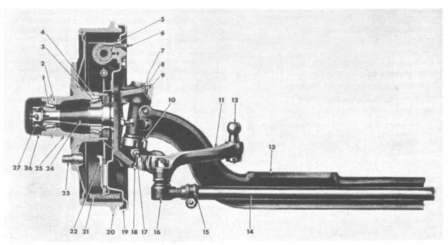
FIG. 226-FRONT AXLE-2-WHEEL-DRIVE MODELS
