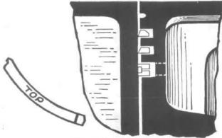
FIG. 115-PISTON RING INSTALLATION
