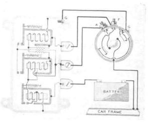
FIG. 168—GENERATOR WIRING DIAGRAM
