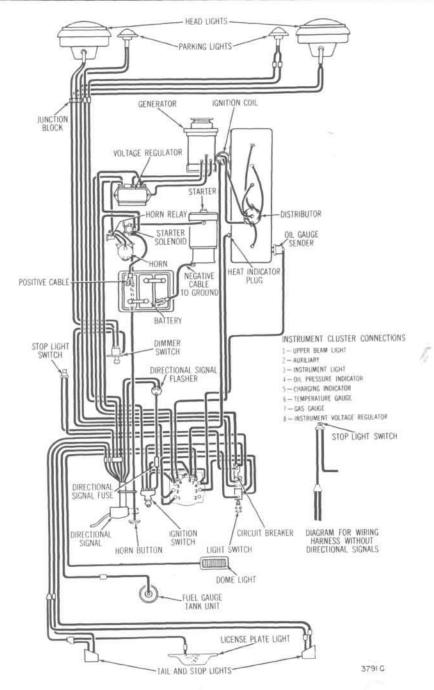
FIG. 156-WIRING DIAGRAM-L6-226 4x4 AND 4x2
