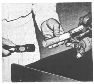
FIG. 214-SHIFT ROD OIL SEAL INSTALLER
