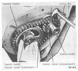
FIG. 26-REMOVING TIMING CHAIN AND GEARS
