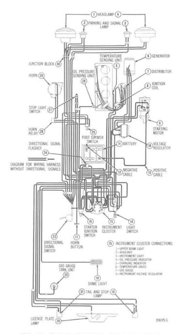
FIG. 158-WIRING DIAGRAM-F4-134 4x4 AND 4x2
