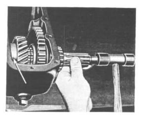
FIG. 210-BEARING CUP REMOVING RING
