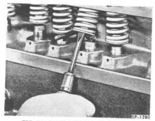
FIG. 24—REMOVING VALVE SPRINGS
