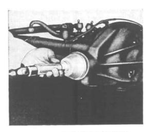
FIG. 267—PINION SHAFT OIL SEAL INSTALLER
