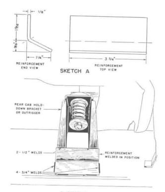
SKETCH B FIG. 311—CAB MOUNTING BRACKET REINFORCEMENT
