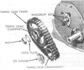
FIG. 84—TIMING GEARS AND CHAIN
