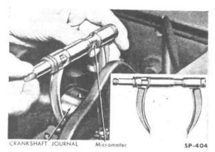
FIG. 44—MEASURING CRANKSHAFT JOURNAL DIAMETER
