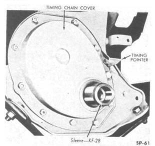
FIG. 86—INSTALLING TIMING CHAIN COVER AND POINTER
