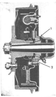
FIG. 294—REAR WHEEL HUB AND BEARING
