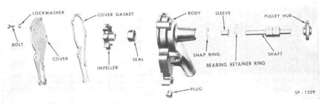
FIG. 153-WATER PUMP-MODEL L6-226
