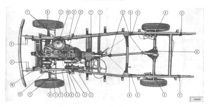
FIG. 5-LUBRICATION CHART - MODEL L6-226 4x2
