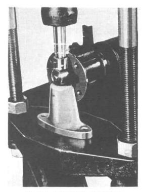
FIG. 223—UNIVERSAL JOINT PIN REMOVER AND REPLACER
