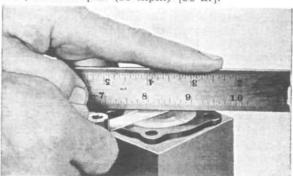
FIG. 123—CHECKING OIL PUMP COVER
