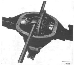
FIG. 245—REMOVING DIFFERENTIAL
