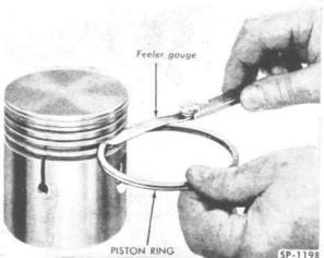
FIG. 42—CHECKING PISTON RING SIDE CLEARANCE
