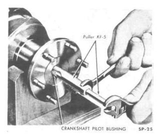
FIG. 45—REMOVING CRANKSHAFT PILOT BUSHING
