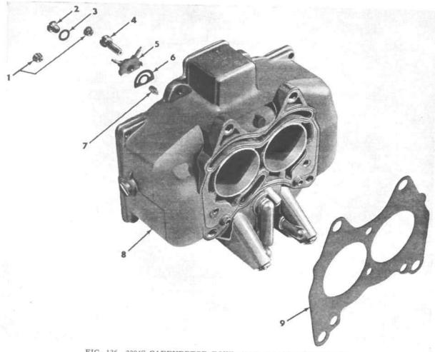
FIG. 136-2204S CARBURETOR BOWL AND ATTACHING PARTS
