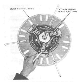
FIG. 176-DISASSEMBLING AUBURN CLUTCH
