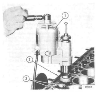
FIG. 60-REFACING VALVE SEATS
