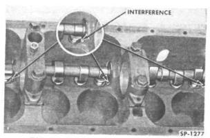
FIG. 85—CAMSHAFT JOURNAL AND TAPPET INTERFERENCE
