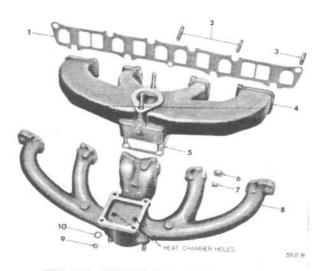
FIG. 143—MODEL L6-226 INTAKE AND EXHAUST MANIFOLD (Single-throat Carburetor)
