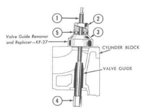
FIG. 66—REMOVING VALVE GUIDE FROM CYLINDER BLOCK
