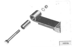
FIG. 299—SPRING PIVOT BOLT
