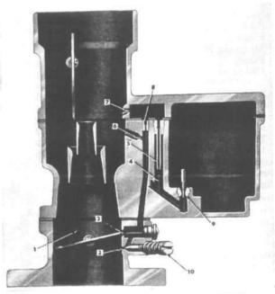
FIG. 129-THE LOW SPEED CIRCUIT
