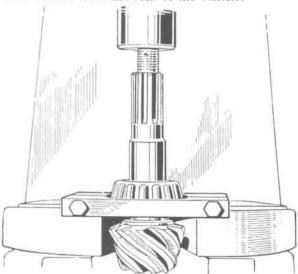
FIG. 252—REMOVING PINION BEARING
