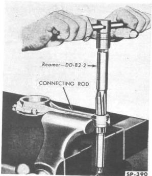
FIG. 39—REAMING CONNECTING ROD BUSHING
