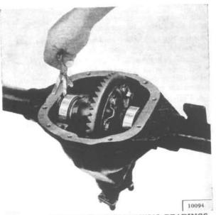
FIG. 262—CHECKING DIFFERENTIAL BEARINGS
