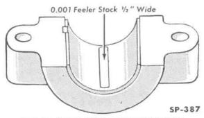
FIG. 50—SHIM STOCK IN POSITION ON MAIN BEARING
