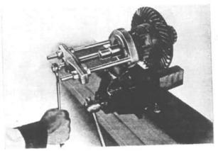
FIG. 268—DIFFERENTIAL BEARING PULLER
