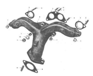
FIG. 142-MODEL F4-134 EXHAUST MANIFOLD
