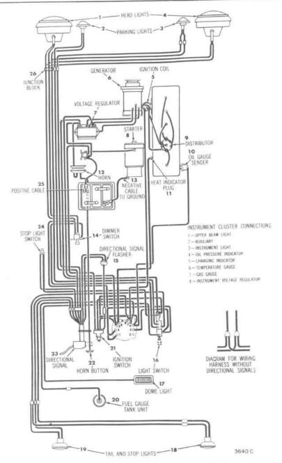
FIG. 155-WIRING DIAGRAM-L6-226 4WD
