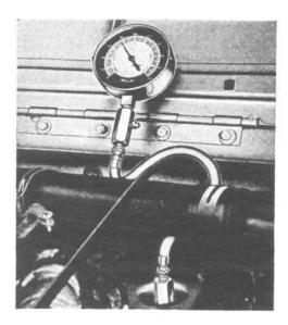
FIG. 18-COMPRESSION AND VACUUM GAUGE
