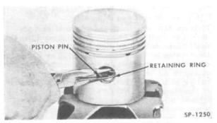
FIG. 36—REMOVING PISTON PIN RETAINING RINGS
