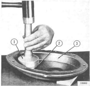
FIG. 57—INSTALLING TIMING CHAIN COVER OIL SEAL
