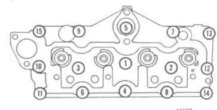
FIG. 104 —CYLINDER HEAD BOLT TIGHTENING SEQUENCE
