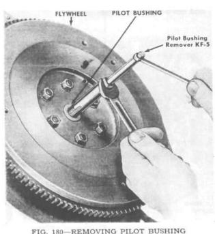
FIG. 180-REMOVING PILOT BUSHING FROM FLYWHEEL
