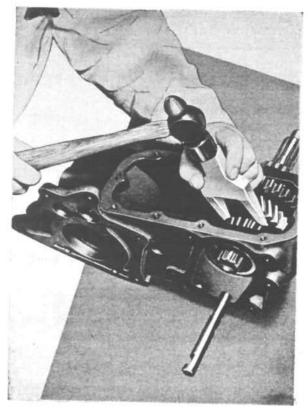
FIG. 209—BEARING CONE REMOVING WEDGE
