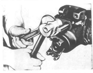
FIG. 212-SHIFT ROD OIL SEAL PULLER
