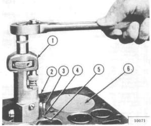
FIG. 20—REMOVING RIDGE FROM CYLINDER BORE
