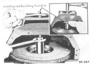
FIG. 187—INSTALLING AND BURNISHING CRANKSHAFT PILOT BUSHING
