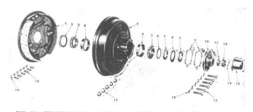
FIG. 291—FRONT WHEEL ATTACHING PARTS—4-WHEEL-DRIVE VEHICLES
