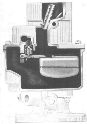
FIG. 127-THE FLOAT CIRCUIT
