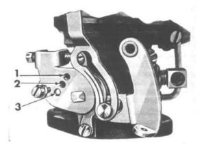
FIG. 317-THROTTLE BELL CRANK
