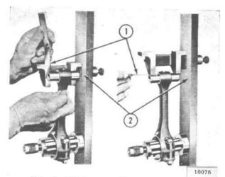
FIG. 40—CHECKING CONNECTING ROD ALIGNMENT
