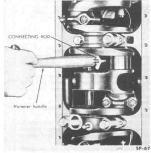
FIG. 21—REMOVING PISTON AND CONNECTING ROD ASSEMBLY
