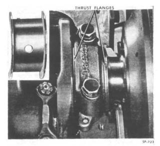
FIG. 51-REAR MAIN BEARING INSTALLATION
