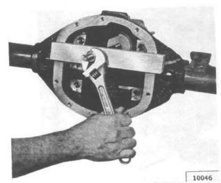
FIG. 249—PULLING PINION SHAFT REAR BEARING CUP
