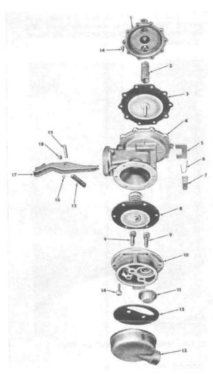
FIG. 140-FUEL AND VACUUM PUMP-L6-226 MODELS
