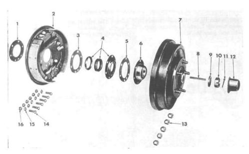
FIG. 293-REAR WHEEL ATTACHING PARTS
