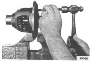
FIG. 246-REMOVING LOCK PIN
