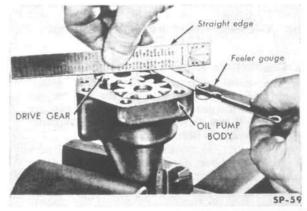
FIG. 76—CHECKING GEAR TO COVER CLEARANCE
