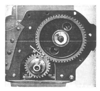
FIG. 108-TIMING GEARS
