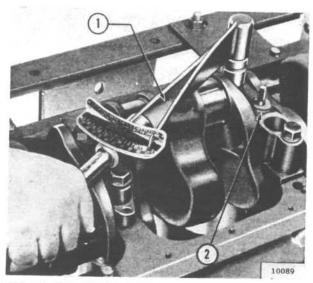
FIG. 81—TIGHTENING MAIN BEARING CAP BOLTS
