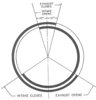
FIG. 88-VALVE TIMING-EARLY L6-226 ENGINES
