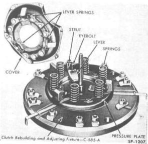
FIG. 183—SIX SPRING CLUTCH COVER PLATE REMOVED
