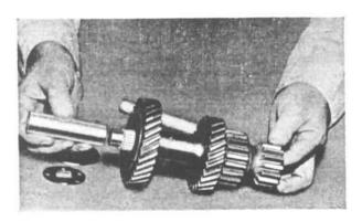
FIG. 191—COUNTERSHAFT GEAR BEARING ARBOR
