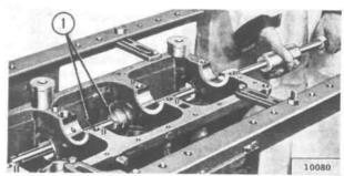
FIG. 54—REMOVING CAMSHAFT BEARINGS 1—Camshaft Bearing Remover and Replacer
