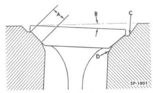
FIG. 64-PROPERLY REFACED VALVE SEAT
