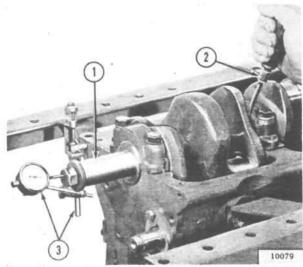
FIG. 52-CHECKING CRANKSHAFT END-PLAY
