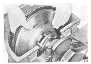
FIG. 82-INSTALLING FLYWHEEL ON CRANKSHAFT
