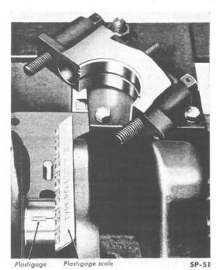
FIG. 49—CHECKING MAIN BEARING CLEARANCE WITH PLASTIGAGE
