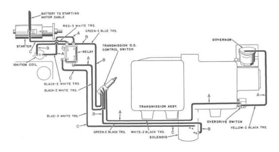
FIG. 198—COLOR-CODED WIRING DIAGRAM—OVERDRIVE
