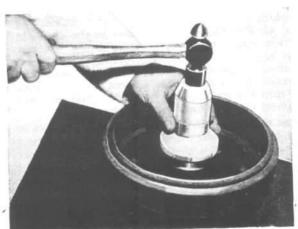
FIG. 290-WHEEL HUB OIL SEAL DRIVER
