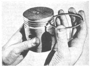
FIG. 117—COMPRESSION RING FITTING
