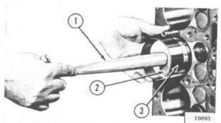
FIG. 87—INSTALLING PISTON AND CONNECTING ROD ASSEMBLY
