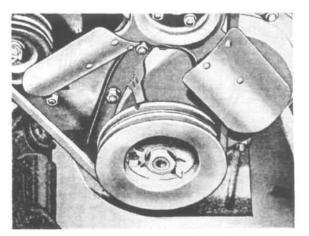
FIG. 13-F4-134 ENGINE TIMING MARKS
