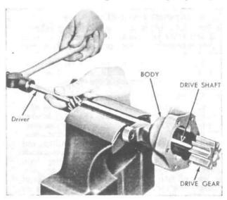
FIG. 74—REMOVING OIL PUMP DRIVE SHAFT AND GEAR
