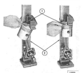
FIG. 41—CHECKING PISTON AND CONNECTING ROD ALIGNMENT
