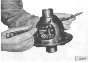
FIG. 259—CHECKING SIDE GEAR CLEARANCE
