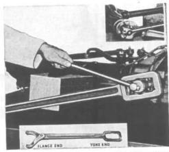
FIG. 247—FLANGE HOLDING WRENCH
