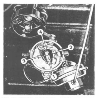
FIG. 163-FIRING POSITIONS - FOUR CYLINDER
