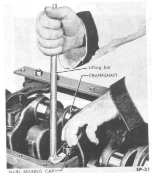
FIG. 28-REMOVING MAIN BEARING CAP
