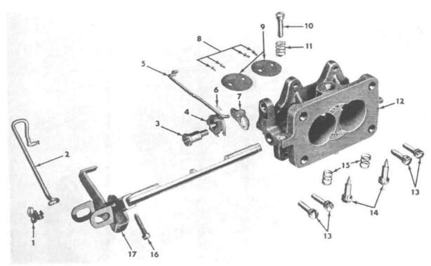
FIG. 137-2204S BODY FLANGE AND ATTACHING PARTS
