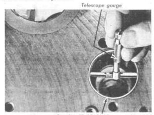
CAMSHAFT BEARING SP-1201 FIG. 53—CHECKING CAMSHAFT BEARING INSIDE DIAMETER
