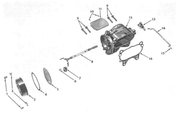
FIG. 138-2204S CARBURETOR AIR HORN AND ATTACHING PARTS
