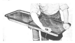
FIG. 308-WINDSHIELD GLASS INSTALLATION
