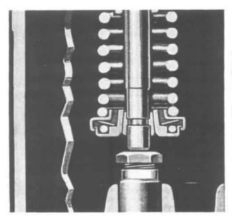
FIG. 11-VALVE WITH BEARING TYPE ROTATOR
