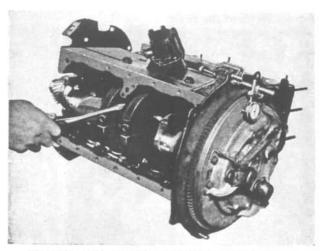
FIG. 107—GAUGING CRANKSHAFT END PLAY
