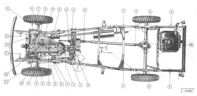
FIG. 3-LUBRICATION CHART-MODEL L6-226 4WD
