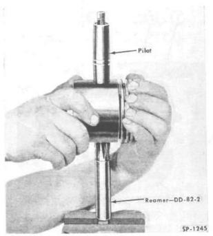
FIG. 38-REAMING PISTON PIN BORE
