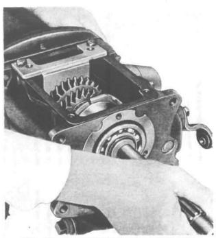
FIG. 196-MAINSHAFT RETAINING PLATE
