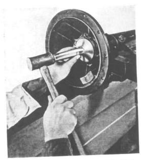
FIG. 272—DIFFERENTIAL BEARING CUP DRIVER
