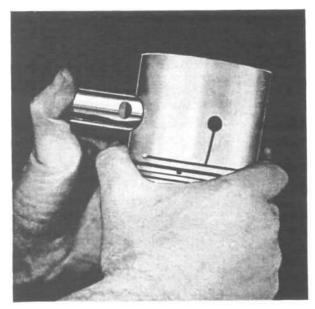
FIG. 118-PISTON PIN FITTING
