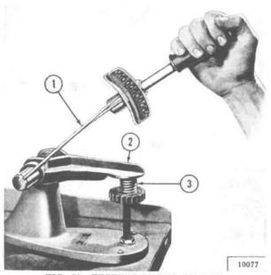
FIG. 58—TESTING VALVE SPRING
