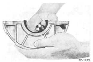
FIG. 72—INSTALLING OIL SEAL IN CRANKSHAFT REAR FILLER BLOCK
