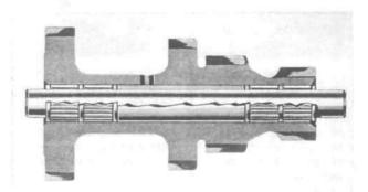
FIG. 192 - COUNTERSHAFT GEAR BEARINGS
