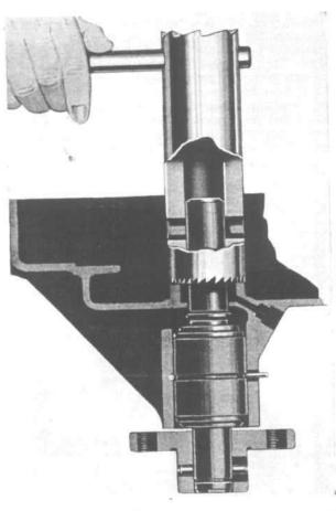
FIG. 152-WATER PUMP HOUSING SEAT REFACER
