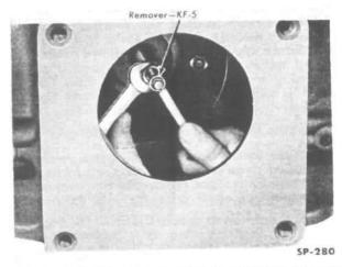
FIG. 186-REMOVING CRANKSHAFT PILOT BUSHING
