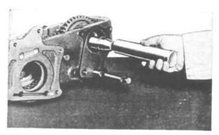
FIG. 216—OUTPUT SHAFT SNAP RING INSTALLER
