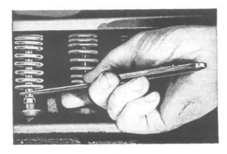
FIG. 103-VALVE TAPPETS AND SPRINGS
