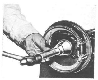
FIG. 218-OUTPUT SHAFT OIL SEAL DRIVER
