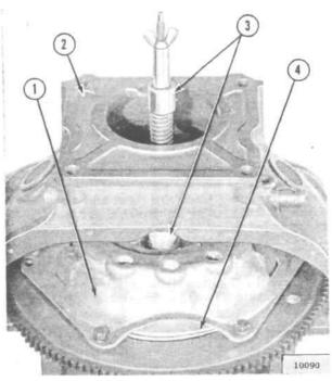
FIG. 83-INSTALLING CLUTCH ON FLYWHEEL
