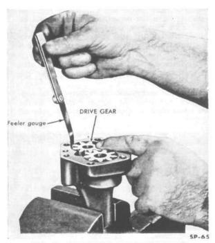
FIG. 75—CHECKING GEAR TOOTH TO BODY CLEARANCE
