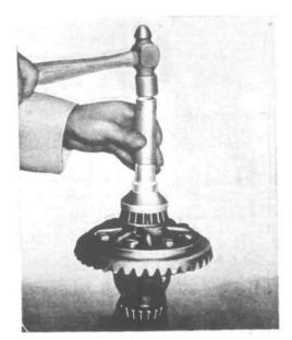
FIG. 261-DIFFERENTIAL BEARING DRIVER
