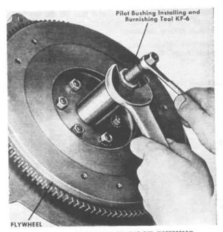
FIG. 181—INSTALLING PILOT BUSHING TO FLYWHEEL
