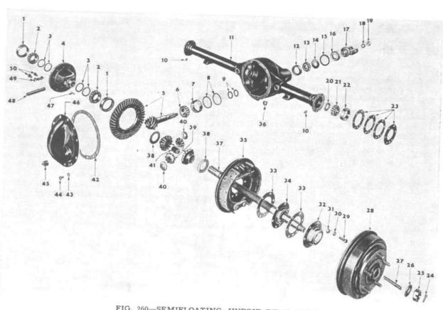
FIG. 260—SEMIFLOATING, HYPOID REAR AXLE
