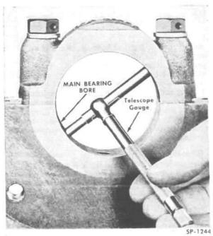
FIG. 48-MEASURING MAIN BEARING BORES
