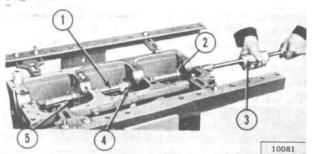
FIG. 55—INSTALLING CAMSHAFT BEARINGS
