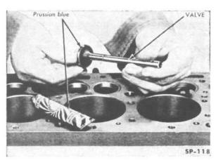
FIG. 65—CHECKING FIT OF VALVE IN VALVE SEAT
