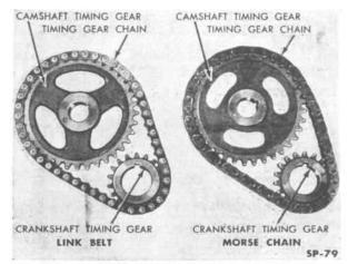
FIG. 56—TWO TYPES OF TIMING CHAINS AND GEARS
