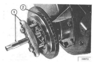
FIG. 25-REMOVING VIBRATION DAMPER
