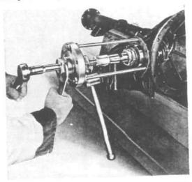
FIG. 273—PINION AND BEARING REMOVER AND REPLACER
