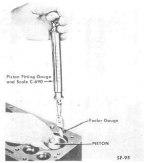
FIG. 37—FITTING PISTON IN CYLINDER BORE
