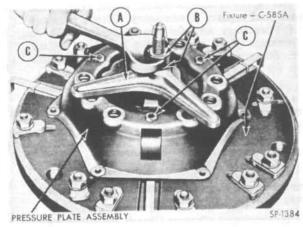
FIG. 182—DISASSEMBLING SIX SPRING CLUTCH
