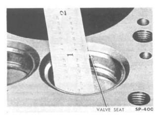
FIG. 61-CHECKING VALVE SEAT WIDTH
