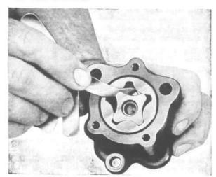
FIG. 121-CHECKING OIL PUMP ROTORS
