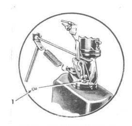
FIG. 318-THROTTLE BELL CRANK
