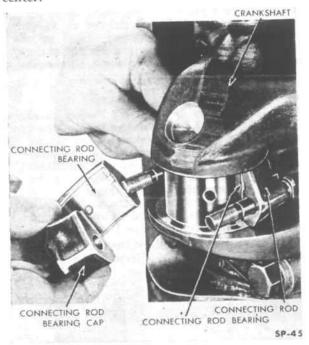
FIG. 90—INSTALLING CONNECTING ROD BEARING CAP
