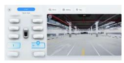
Tap the "Start" button on the Intelligent Parking Assist interface, the vehicle will start to enter the parking space.
