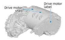
The drive motor model and code are presented on the drive motor shell and the drive motor label.
