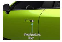
Pull up the door handle and insert the mechanical key into the lock hole:
