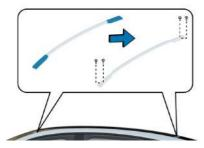
The roof rack interface can be used to install optional roof rack. If using a roof rack, follow the instructions and safety warnings provided in this section and the instruction manual of the roof rack.
