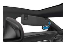
When the sun visor is flipped down, pull it out from the movable bracket along the arrow direction to block the sunlight shining through the side windows.
