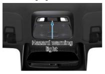
Press the hazard warning light switch on the front reading lights to turn on the hazard warning lights. Then all turn signal lights will flash. Press again to turn it off.
