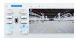
When the Intelligent Parking Assist detects available parking spaces, and the vehicle is stopped safely, the driver can choose the target parking space and tap "Start" for Intelligent Parking Assist.
