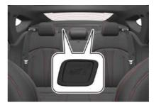
The ISOFIX top tether points are located behind the headrests of rear seats on both sides and can be seen by opening the trim lids.
