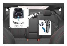
Wrap the tether around the inner headrest position, open the trim lids of the anchor points, attach the hook and loop to the anchor points and tighten the tether.
