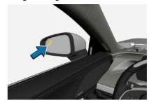
When a target approaches the stationary vehicle, the DOW will illuminate the warning indicator, at which point the driver or the passenger should avoid opening the door and confirm that it is safe to open the door first. If the driver or passenger opens the door on the alarm side at this time, the warning indicator will flash, accompanied by a warning sound and the door ambient light on the corresponding side, to alert the driver or passenger to be careful and be safe.
