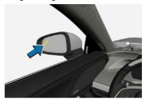
When Blind Spot Security is in the warning state, the driver shall avoid making lane changes, and if the driver turns on the turn signal indicator on the warning side at this time, the blind zone warning light of exterior rear-view mirror on that side will flash to send warning signal.
