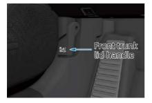
Pull the front trunk lid handle on the lower left side of the dashboard twice in succession, and the front trunk lid will pop up slightly to unlock.
