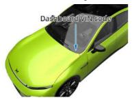
1. Applied to the bottom left side of the dashboard and can be seen through the windshield.
