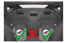
The child safety seats can only be installed in the rear seats on both sides.
