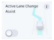
After the vehicle is Ready, the ALC switch defaults to the last operating state. After shifting the gear to P, tap "Vehicle Control → XPILOT → Active Lane Change" to turn on/off ALC.
