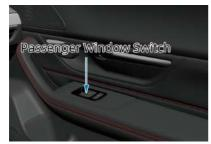
The left rear door, right front door and right rear door are equipped with a passenger window switch with 2 levels of operation:
