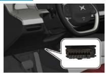
The OBD interface is located on the lower left rear of the dashboard and allows you to read the electronic VIN number and other information through an original diagnostic device or an official authorized diagnostic device.
