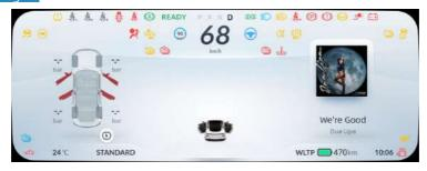
Some indicator lights will come on when the vehicle is powered on and go off after system self-inspection. Some indicator lights are on to indicate the current status of the vehicle system functions, not for system faults.
