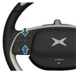
To change the set speed when ACC is activated, press the up/down button in the area left of the steering wheel until the desired set speed is displayed and then release.
