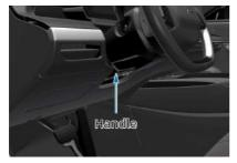
The steering wheel handle is in the locked position by factory default.
