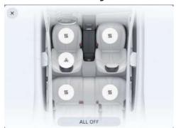
Tap the \$\iiii \text{ button to turn on the heating for the corresponding seat, and the heating intensity will change by one level with each click of the button.
