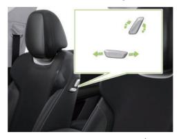
Boss button is equipped on the upper left side of the front passenger seat backrest, which is convenient for the rear seat passengers to adjust the front passenger seat.
