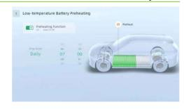
Tap "■→Low-temperature Battery Preheating", or directly open the XPENG App to turn on the low-temperature battery preheating function, and set the preheating time.
