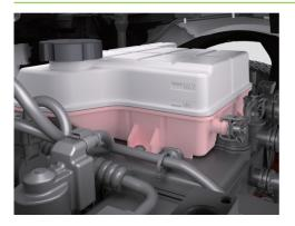
Check the level mark on the side of the coolant reservoir:
