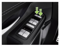
The door lock switch is located at the driver-side door armrest:
