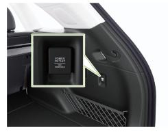
12V Power Supply Port: Maximum supported power is 180W.
