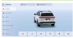
Tap "♠→Controls" in turn on CID, or tap the suspension area on the 3D vehicle model to set the air suspension functions.
