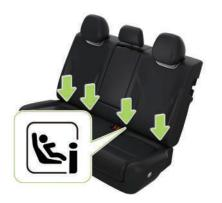
The ISOFIX anchorages are located between the backrests and cushions of the rear left and right seats. The exact location of each anchorage is marked as above (as shown in the figure).
