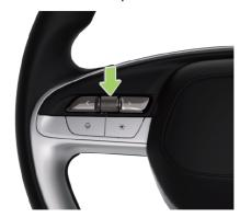
The roller at the left of the steering wheel can be used to set the cruise vehicle speed. Rolling up means acceleration, and rolling down means deceleration.
