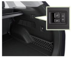
Press the up or down switch of the trunk inner suspension to adjust the height of the trunk, which can facilitate the loading and unloading of items.
