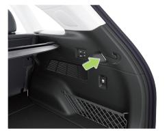
The trunk light automatically turns on when the trunk is opened.
