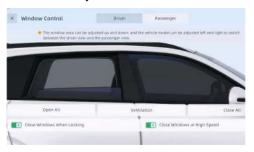
Tap "♠ → Controls→ Window Control" in turn to access the window adjustment interface. From there, you can adjust the window position, enable/disable the auto-closing window when locking, and enable/disable the auto-closing window at high speed.
