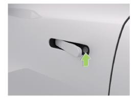
Press the front side of the driver's door handle to extend it, then insert the mechanical key to the keyhole.
