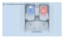
Open the A/C interface and tap "A" to activate the seat ventilation or heating interface.
