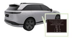
The product nameplate is located on the B-pillar of the front passenger's door. You can view it by opening the front passenger's door.
