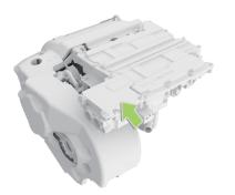
The front drive motor model and code are presented on the drive motor housing and the drive motor label.
