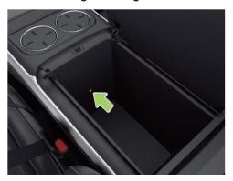
The sub IC storage box light will turn on when the box is opened, and it will automatically turn off when the box is closed.
