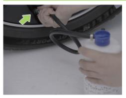
4. Screw one end of the sealant injection tube onto the tire valve and tighten it. Be careful not to invert the tire sealant can.
