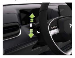
After turning on the turning lamps, the corresponding indicator on the ICM flashes and a "clicking" sound is heard.
