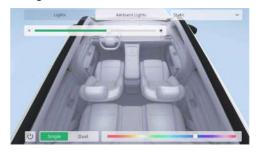
Via the CID, navigate to "■ →Lights→Ambient Lights" to enter the ambient light control interface. Tap the switch to turn the ambient lights on or off.
