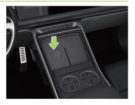
The wireless charging area is located inside the front storage box. When charging, please place the phone with the front side up within the sensing area along the stop bar. The CID will display an icon "• " while charging.
