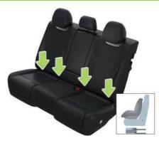
Insert the lower anchor bracket of the child safety seat into the ISOFIX anchorages according to the child seat manufacturer's instructions.
