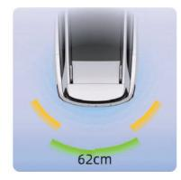
When the parking radar system is activated, ICM will simulate the approximate direction and distance of obstacles relative to the vehicle. Green indicates a greater distance, while red indicates a very close one. The distance between the vehicle and the nearest obstacle is also displayed numerically below.
