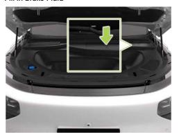
Wrap a flat head screwdriver in a cloth, open and remove the upper trim panel of the reservoir at the position indicated by the arrow in the figure.
