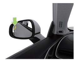
When the vehicle speed is greater than 10km/h, if there is a vehicle in the blind spot or a fast-approaching one behind the blind spot, the corresponding side's exterior rearview mirror warning light will illuminate. If the turning lamp or lane change signal on that side is activated at
