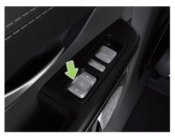
The rear door panels are equipped with rear seat backrest adjustment buttons, which is convenient for rear passengers to adjust the backrest angle.
