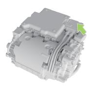
The rear drive motor model and code are presented on the drive motor housing and the drive motor label.
