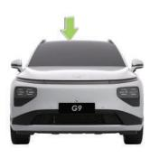
The microwave window is on the front windscreen. Please keep the front windscreen clean so as to ensure the best results and minimize interference with the driving view.
