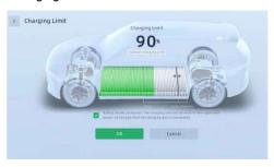
In order to protect the health of the battery, the vehicle is equipped with a charging limit function. Some models will not fully charge when charging. If there is a need for long-distance use, the charging limit can be set on the charging limit interface.
