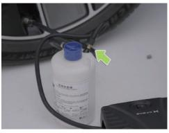
Connect the other sealant injection tube to the inflatable pump and tighten it, then insert the electrical source plug of the inflatable pump into the 12V power supply in the vehicle storage box.
