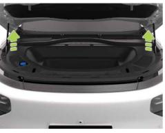
Slightly lift the front hood, and it will automatically rise to the limit position with the left and front air springs.
