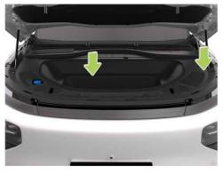
Remove the front compartment trim panel and storage box with proper tool, and you can see the coolant reservoir.
