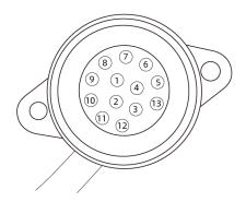
The vehicle is equipped with a 13-pin electrical connector coil, following the ISO 11446:2004 standard for the power supply socket. Each pin has specific functions as following:
