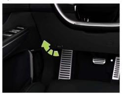
The front hood opening handle is located on the left side of the driver's foot space.
