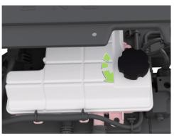
2. Unscrew the reservoir cap and fill the coolant.
