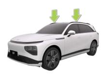
The vehicle features mounting holes for an optional roof rack. When using a roof rack, please follow the instructions and safety warnings provided in this section, as well as the user manual for the roof rack itself.
