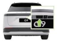
When the vehicle is unlocked, you can press the exterior trunk switch and the trunk will automatically open.
