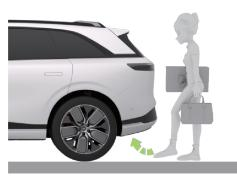
If there is a remote control key near the rear trunk, the rear trunk can be unlocked and opened or closed by foot movements.
