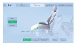
Select "Passenger > Leg Rest", and you can move forward/backward the leg rest.
