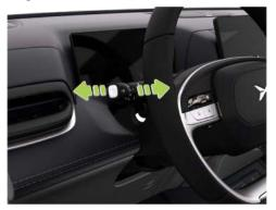
After the low beam is on, move the combination switch forward once, and the high beam is on. Move the combination switch forward again, and the high beam goes off;  Continuously move the combination switch backwards and release it, and the high beam will flash to remind the preceding vehicle.
