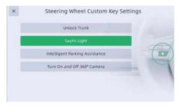
Tap "■ → Vehicle Settings→ Customized Key Settings" in turn on CID to set the custom functions for the steering wheel buttons.
