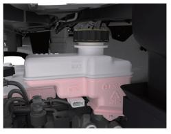
Check the level mark on the side of the brake fluid reservoir:
