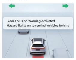
When the vehicle speed is between O-160 km/h, if there are vehicles, pedestrians, or two-wheelers approaching at a certain speed within the detection range, and there is a crash risk, RCW will be activated. It will provide warnings through ICM, audible alerts, and illuminate the
