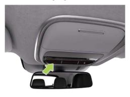
Press the hazard warning light switch on the roof switch panel to turn on the hazard warning lights, and all turning lamps will flash.
