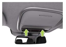
The interior reading light is installed in the switch panel on the roof. To turn on the reading light, simply touch the corresponding touch area on the reading light cover. Touch it again to turn it off.
