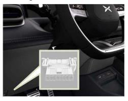
The OBD interface is located on the lower left of the instrument cluster and allows you to read the electronic VIN number and other vehicle information through an original diagnostic device or an officially authorized diagnostic device
