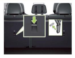
3. Thread the top tether strap of the child safety seat through the headrest, pull it to the back of the backrest, connect the hook of the strap to the anchor point, and tighten the strap.
