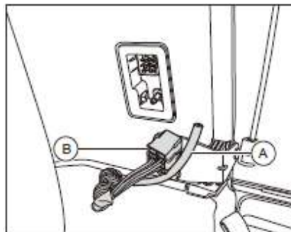
5. Unplug the right side of the rear panel - B-and Rubber tube - A - (illustrated position).
