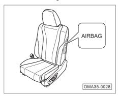
The front seat side airbags are installed in the outboard sides of the driver's seat back and the front passenger's seat back respectively (as indicated by the dotted dash) marked with "SRS AIRBAG".
