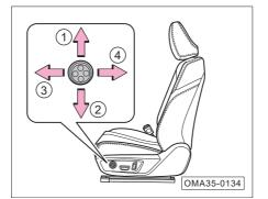
Press the switch in the direction of arrow
