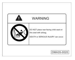
Warning labels are pasted on the front and back of the right sun visor to remind the front passenger of the danger of frontal airbag. Be sure to read and follow the instructions on the labels
