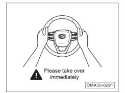
When the LDW detects that the steering wheel is out of the driver's hands for a long time, the system will issue a hands-on reminder and the instrument cluster displays an alarm message while beeping.
