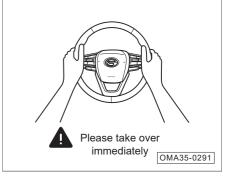
When detecting that the steering wheel is out of the driver's hands for a long time, TJA/ICA will issue a hands-on reminder and the instrument cluster will give a visible alarm and an audible alarm.
