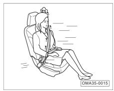
The seat belt pretensioner and load limiter can reduce the pressure of the seat belt on the chest of the driver or passenger and improve the protection performance.
