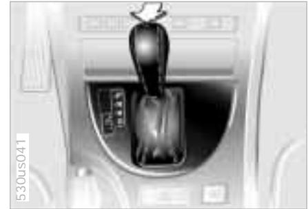
You can drive as with a normal automatic transmission. In addition, you can also shift manually.
