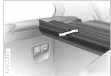
When the cover is pulled out, it can be opened behind the rear-seat backrest to gain access to the cargo area from the rear seats during a trip, for example. For removing the cover: refer to the next page.
