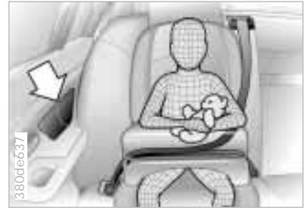
This is the right way for a child to sit in a child restraint when rear side airbags (arrow) are provided.
