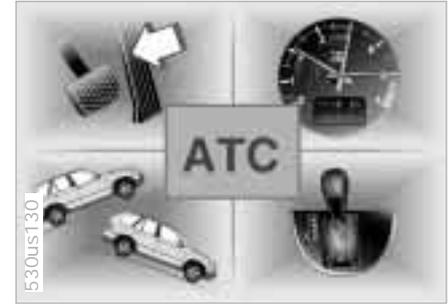
Adaptive Transmission Control (ATC) uses a number of factors to calculate the gear which provides the maximum efficiency of the automatic transmission. In this process, the system monitors your personal driving style, the driving situation, the condition of the road, and the traffic conditions.
