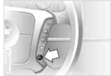
Steering wheel heating functions in ignition key position 2.
