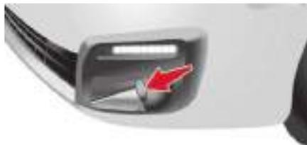
With dipped or main beams, this system makes use of the beam from a front foglamp to illuminate the inside of a bend, when the vehicle speed is below 25 mph (approximately 40 km/h) (urban driving, winding road, intersections, parking manoeuvres, etc.).
