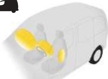
The airbags have been designed to optimise the safety of the occupants in the event of a serious collision; they work in conjunction with the force limiting seat belts.
