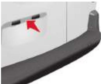
The reversing camera is activated automatically when reverse gear is engaged.
