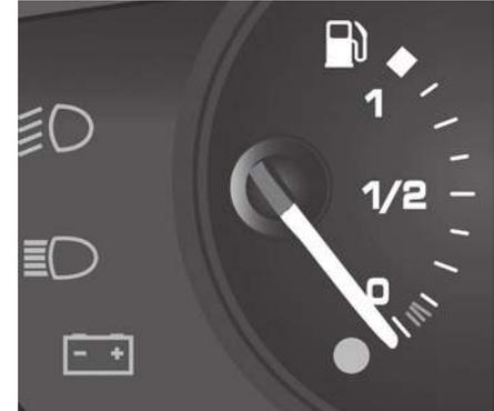
The fuel level is tested every time the ignition is turned to the "on" position.
