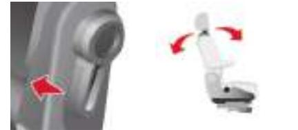
☞ With your back pressed against the backrest, press the lever forwards and set the desired angle.
