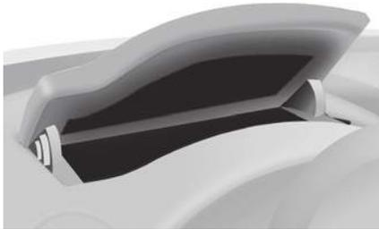
A cut-out makes it easier to raise the cover to open it. Guide it to its stop position. To close it, guide the cover then press the centre gently. Any liquid which could spill risks causing an electrical short circuit and therefore a potential fire.
