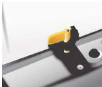
**i** It is possible to drive with the right-hand door open to make it easier to transport long loads. The left-hand door is kept closed by the distinctive "yellow" lock, positioned at the base of the door. This closed door must not be used to restrain the load.
