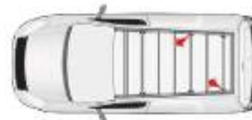
If you install transverse bars on these bars, refer to the weight values indicated by the manufacturer and do not exceed: 75 kg.
