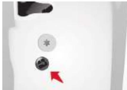
In the event of a battery or central locking fault, use the lock to lock the doors mechanically.
