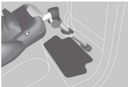
If the support leg is long enough and can be angled sufficiently (always respecting the recommendations given in the child seat installation instructions), you can position the support leg in such a way that it is in contact with the floor away from the storage compartment area. Consider using the longitudinal adjustment of the rear seat or front seat to obtain a satisfactory position for the support leg away from the storage area.
