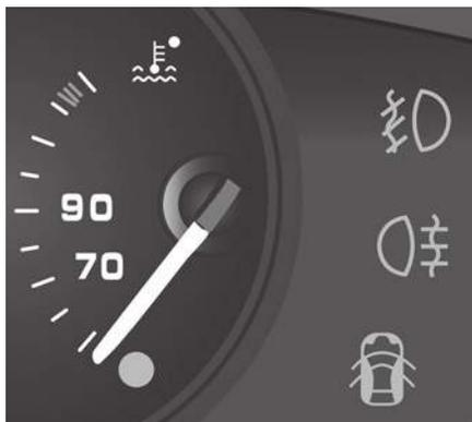
**The needle is positioned before the red zone:** normal operation.
