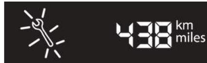
A few seconds after the ignition is switched on, the oil level is displayed, depending on the version, and then the distance recorder
