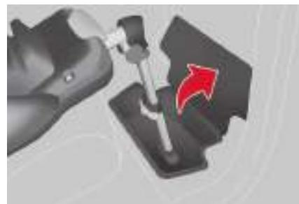
If the support leg is long enough, you can adjust it so that it is in contact with the bottom of the storage compartment. Remove all objects from the compartment before installing the support leg.
