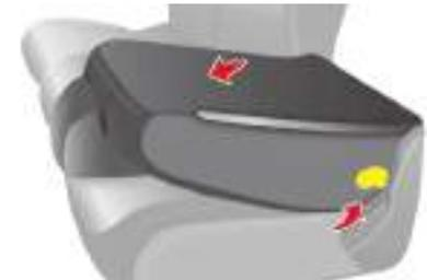
☞ Operate the control to fold the backrest onto the seat cushion.
