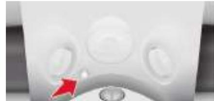
The fragrance diffuser diffuses a fragrance in the passenger compartment from the roof console vents.
