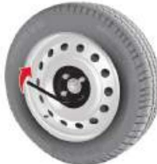
☞ Carry out an initial tightening of the bolts using the wheelbrace.
