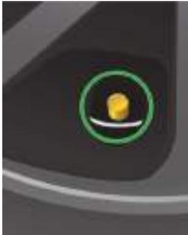
Correct valve position: above the ring.
