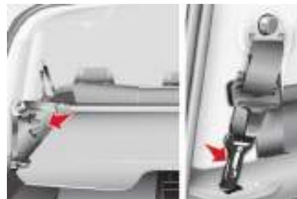
The row 3 seat belts which are not in use can be stored to clear the load space and to make use of the load space cover easier. Hook the spring hook into the location provided on the rear pillar trim.
