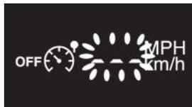
The programmed speed is cleared, then replaced by three dashes.
