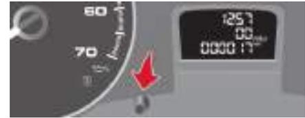
To adjust the time on the clock, use the left-hand button on the instrument panel.
