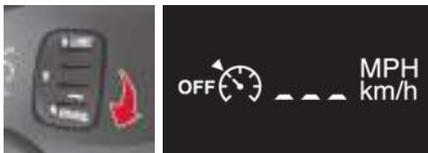
☞ Turn the knob to CRUISE position. The cruise control is selected but is not yet active and no speed has been programmed.
