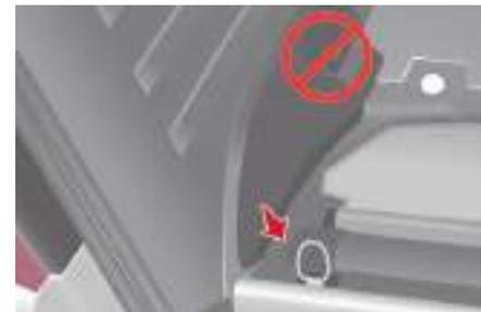
Use the stowing rings on the floor to firmly attach and secure your loads.
