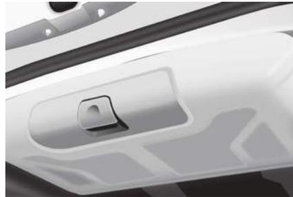
☞ From the vehicle boot, place your thumb on the recess then pull the handle to open.
