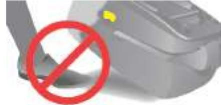
**!** Ensure that no object or foot of a passenger seated in the rear is obstructing the anchorage points or preventing correct locking of the seat.
