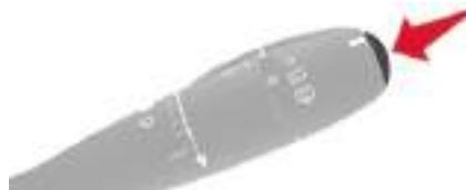
Each press of the button on the end of the windscreen wiper stalk allows you to scroll through the various trip computer information displays, depending on the screen.
