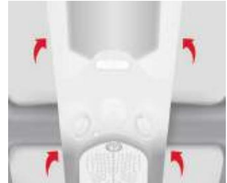
Storage compartments are provided on each side of the roof. The maximum authorised load is 6 kg.
