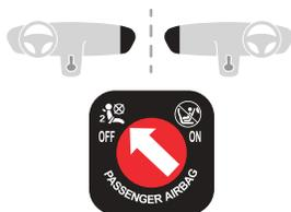
Only the passenger's front airbag can be deactivated.
