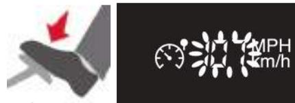
Pressing the accelerator pedal in order to exceed the programmed speed will have no effect unless you press the pedal **firmly** beyond the **point of resistance**.
