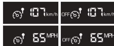
A first press on this button switches the speed limiter on, a second press deactivates it (**OFF**).
