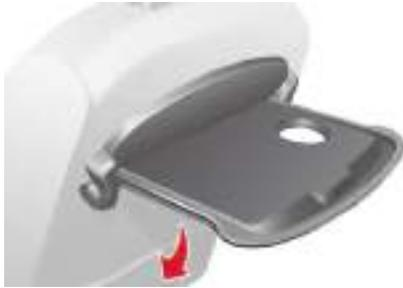
☞ To put the table in place, pull it upwards and fold it down.
