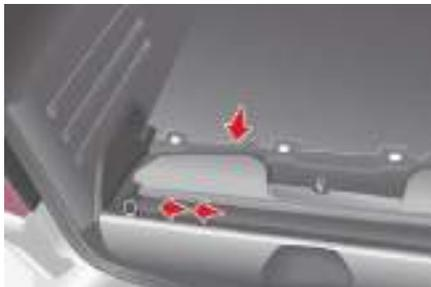
The recess immediately next to the boot sill is intended to accommodate the rolled tube containing the load space cover.
