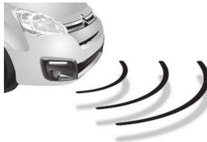
In addition to the rear parking sensors, the front parking sensors are triggered when an obstacle is detected in front and the speed of the vehicle remains below 6 mph (10 km/h).
