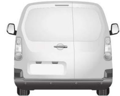
The side-hinged rear doors are asymmetrical (2/3-1/3), with the small side on the right. They are fitted with a central lock.
