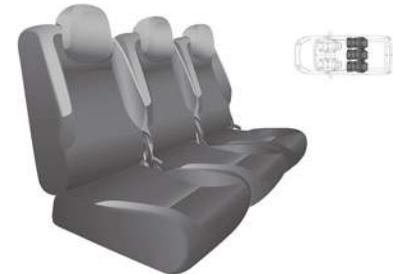
The three independent rear seats are fitted with rounded head restraints.
