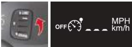
☞ Turn the knob to the **LIMIT** position. The speed limiter is selected but is not yet active. The display shows the last programmed speed.
