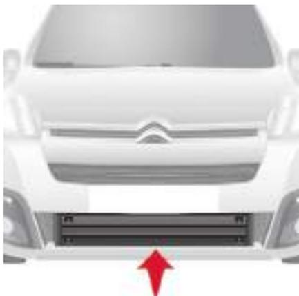
Depending on country, the removable snow shield plug is installed on the lower part of the front bumper, to avoid the accumulation of snow at the radiator cooling fan.
