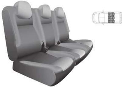
The 1/3-2/3 rear bench seat is fitted with rounded head restraints. Each 1/3-2/3 section can be folded into the fully folded position, then removable individually.
