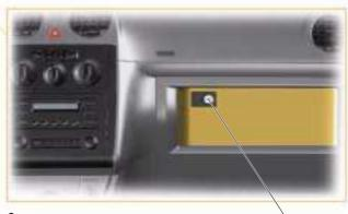
Storage compartment on passenger side containing key switch for front passenger airbag
