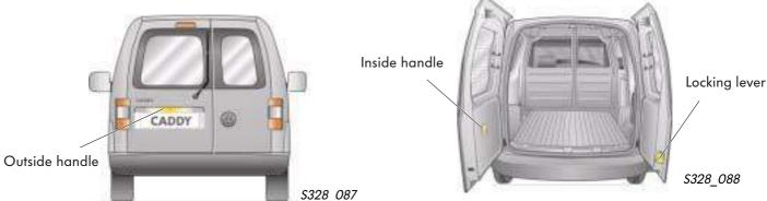
The left-hand wing door needs to be opened first. The outside handle on the left-hand door is integrated in the number plate light fitting. The locking level built into the bottom of the right-hand door can then be used to open the right-hand wing door. Wing doors lock at a 90° angle when opened. If the door latches are detached, the wing doors will open to approx. 170° due to a stop in the hinge.
