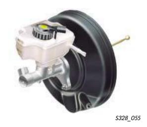
Crash-optimised pressure rods are built in the brake servo.
