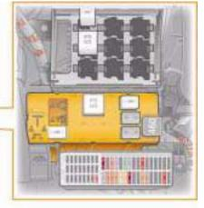
Relay carrier on control unit for onboard supply, on left under dash panel
