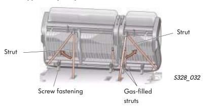
The double seat bench for the second row of seats is fixed to the floor with 4 bolts.
