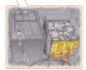
Pre-fuse box on left of engine compartment
