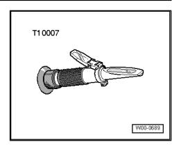
Read precise value for the following tests at bright/dark boundary. Using a pipette, place a drop of water on the glass to improve the readability of the bright/dark boundary. The bright/dark boundary can be clearly recognised on the "WATERLINE".
