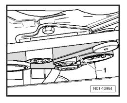
To pull off lines -1- press release buttons on connecting pieces of fuel filter -2-.
