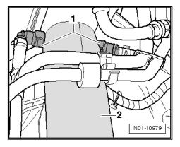
To remove fuel filter -1-, press fuel filter from below -movement arrow- upwards out of holder -2- and remove it downwards.
