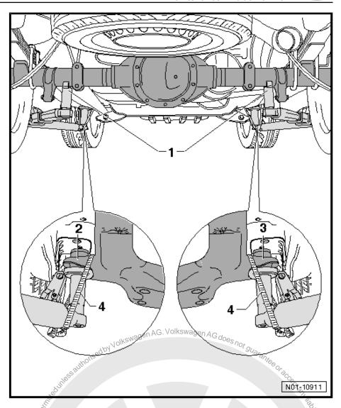
Vehicle can now be raised and lowered to required working height.
