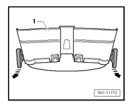
Remove "SC fuse / 25 A" -arrow-, which is attached to dash panel insert -K-.
