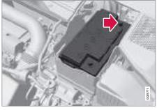
1. Lower the battery into the battery box.
