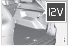
Fold down the cover to access the electrical socket. It works irrespective of whether or not the ignition is switched on.
