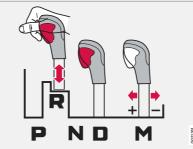
The gear selector can be moved forward and back freely between N and D. Other positions are locked with a latch that is released with the inhibitor button on the gear selector.
