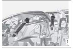
When installing, check that the long lock pin is engaged - it should be engaged in both eyes.
