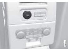
12 V socket in tunnel console, rear seat.
