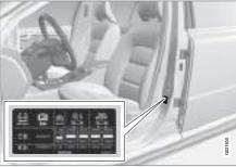
The tyre pressure label on the driver's side door pillar (between front and rear door) shows which pressures the tyres should have at different loads and speed conditions, this is also specified in the tyre pressure table, see below.
