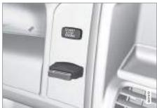
Ignition switch with remote control key, start/stop button.
