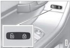
All of the doors and the tailgate can be locked or unlocked simultaneously using the central locking button on either front door. Press one side of the button to lock - the other side to unlock.
