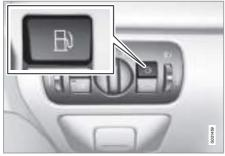
Open the fuel filler flap using the button on the lighting panel. The filler flap is located on the right-hand rear wing, as indicated by the symbol's arrow in the information display.
