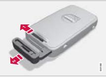
Unlocking doors with the key blade
