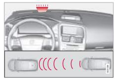
A small section of the red warning lamp in the windscreen illuminates with a constant glow when driving closer than the set time interval to vehicles in front.
