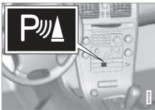
The system is automatically engaged when the car is started and the switch's On/Off lamp is illuminated. If parking assistance is switched off with the button, the lamp goes out.
