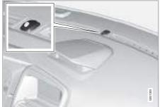
A red LED on the instrument panel indicates the alarm system's status:
