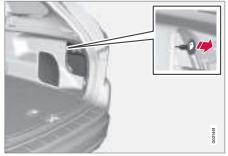
The fuel filler flap can be opened manually when electric opening from the passenger compartment is not possible.
