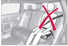
Incorrect position, the head must not be positioned above the head restraint and the seatbelt must not be below the shoulder.
