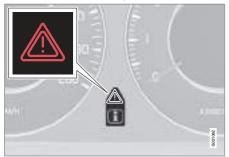
If the car is involved in a collision, the text **Safety mode See manual** may appear on the information display. This means that the car has reduced functionality. Safety mode is a protective state that is enforced when the collision may have damaged any of the car's vital functions, such as the fuel lines, sensors for one of the safety systems, or the brake system.
