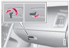
The glovebox can only be locked/unlocked using the remote control key's detachable key blade. (For information on the key blade, see page 42).
