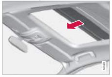
One long press on the lock button, see pages 43 (remote control key) and 50 (central locking button), closes the panorama roof and all the windows. The door mirrors are retracted\* and the doors and tailgate are locked. To interrupt closing, press the lock button again.
