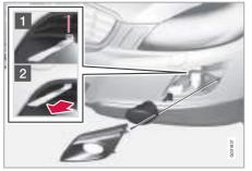
Undo the cover by pulling out the top corner, closest to the grille, see the illustration above.
