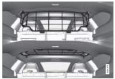
A safety grille prevents loads or pets from being thrown forward in the passenger compartment in the event of sudden braking. For safety reasons, the grille must always be mounted and secured correctly.
