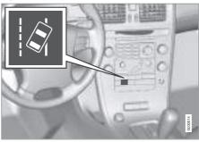
The function is switched on or off by means of a switch on the centre console. An indicator lamp in the button illuminates when the function is switched on.
