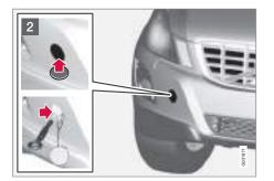
2 Use a slotted screwdriver or a coin to detach the cover at its bottom edge.
