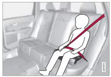
Correct position, the seatbelt is positioned above the shoulder.
