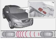
Laser sensor transmitter and receiver window.
