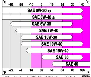
\* Oils with viscosity 0W-30 and 0W-40 must fulfil the requirements of ACEA A3 (petrol engines).
