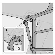
Red marking - unlocked Green marking - locked
