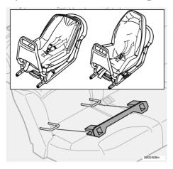
**NOTE:** Isofix attachment points are located on both outer rear seats. The rail can be moved from one side to the other as needed.
