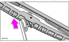
Then pull the blade up so that the wiper arm eye passes beside the wiper blade mounting.
