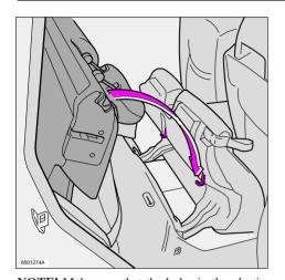
NOTE! Make sure that the holes in the plastic ferrules on the top of the backrest engage with the hooks on the bottom of the seat cushion. When you later raise the backrest and seat cushion, the head restraints must be returned to their normal positions.
