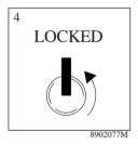
Turn the key anticlockwise to the locked position and remove it from the lock.
