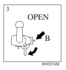
Remove the connector pin cover.
