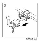
Put in the key and turn it clockwise to the unlocked position.
