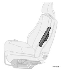
The side impact airbags are installed in the front seat backrest frames
