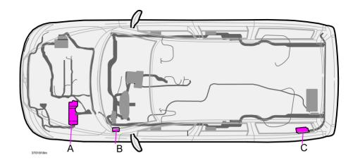
If an electrical component or function does not operate it may be because the component fuse was temporarily overloaded and burned out. Look in the fuse diagram to locate the affected fuse. Pull out the fuse and look at it from the side to see if the curved wire is burned out. Replace with a new fuse of the same colour and amperage. The fuse box in the engine compartment contains a number of spare fuses. There are also pliers to assist you in pulling out and replacing the fuses.
