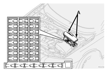
A. Press in the catches on the rear of the box and pull the cover up.
