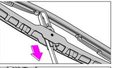
Press the entire wiper blade down so that the wiper arm eye passes through the hole in the wiper blade mounting.
