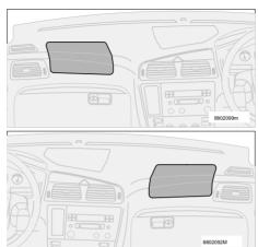
The side airbag is above the glovebox, marked SRS
