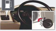
Press the button to open the fuel filler flap. Hang up the fuel filler cap during refuelling.
