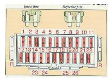
The fuses are removed by pulling them straight out. If they are defective, the metal wire is broken. When fitting a new fuse, be certain to use one with **the same amperage and color** as the one removed (see top of fuse)! Spare fuses are located on each side of the fusebox (1x15A, 1x25A, 1x30A).
