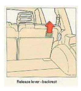
Remove head restraints from rear seat. This is done by grasping the restraint and lifting straight up. Move the backrest release lever upwards and fold the backrest forward.
