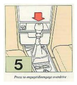
The overdrive is automatically disengaged when downshifting from 4th gear, but you should always disengage the overdrive manually before downshifting.
