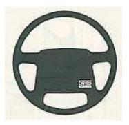
As an enhancement to the three-point seatbelt system, certain models are equipped with a Supplemental Restraint System (SRS). The Volvo SRS consists of a driver's side airbag with a driver's side knee bolster. The system is designed to supplement the protection provided by the three-point seatbelt system.
