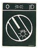
With the headlight switch in position it the parking lights will stay on. Switch from high to low beams, and vice versa, by moving the turn signal switch lever on the left side of the steering column towards the steering wheel.
