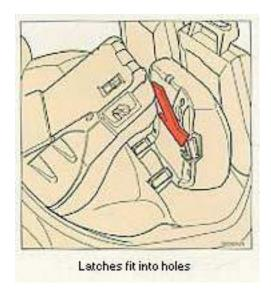
**Important:** Check that latches under seat cushions engage holes at top edge of backrest. Seat belts must be correctly positioned as seat is returned to normal position.
