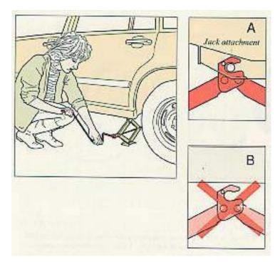
There is a jack attachment adjacent to each wheel location. Hang the jack from the attachment as shown in the illustration and crank while simultaneously guiding the base to the ground. **Before raising the car check that the jack is still correctly positioned in the attachment.**
