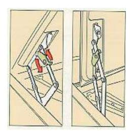
The normal opening angle for the hood is approximately 55°. By turning the catches or the hinges as illustrated, the hood can be opened to the vertical position. The catches will return to their normal positions when the hood is closed.
