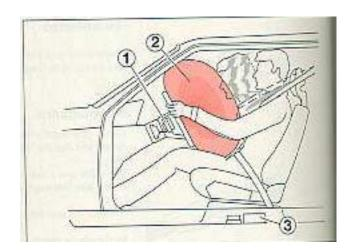
The airbag system includes a gas generator (1). surrounded by airbag itself (2). In the event of a frontal or front-angular collision equivalent to impacting a rigid barrier at 12 mph (19 kph) or greater the sensor (3) activates the gas generator causing the airbag to be inflated with harmless nitrogen gas. As the movement of the driver compresses the airbag some of the gas is expelled at a controlled rate to provide better cushioning.
