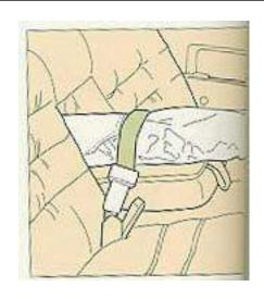
Protective covers (for skis) should also be used to avoid soiling or tearing the upholstery. Please note that the flap in the rear seat is only intended for light loads such as skis, wood etc.
