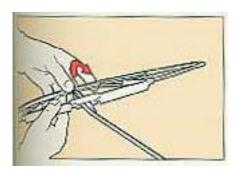
Install new blade, installation is the reverse of removal, and make sure that it is properly attached to the wiper arm.
