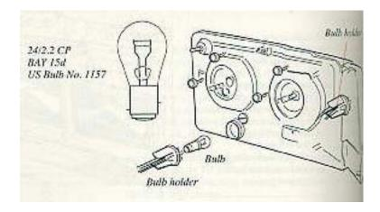
5 Turn the bulb holder clockwise to secure it. Check the bulb function.
