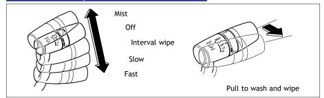
With the wiper lever in the OFF or INT position, the wipers will operate continuously until the lever is released.
