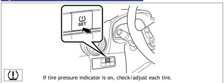
After adjusting tire pressures, or after tires have been rotated or replaced, turn the ignition switch to "ON" and press and hold the "SET" button until indicator blinks twice and a beep sound once. Let the vehicle sit for a few minutes to allow initialization to complete.
