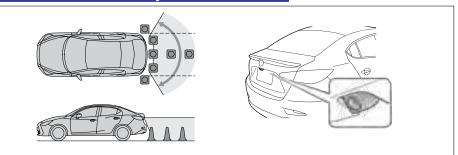
The rear view monitor system displays an image of the view from the bumper of the rear area of the vehicle. The camera for the rear view monitor system is located above the license plate.
