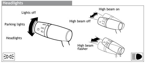
When the headlights are turned off, the high beams will only operate in the flasher mode.
