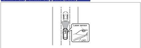
Smart City Brake Support (SCBS) is designed to reduce damage in the event of a collision by operating the brake control (SCBS brake) when the system's laser sensor detects a vehicle ahead and determines that a collision with a vehicle ahead is unavoidable.
