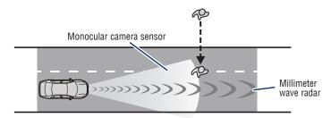
As part of the Pre-Collision System, this function is also designed to first provide an alert and then automatic braking if needed.
