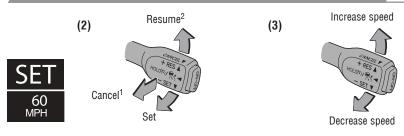
Vehicle will cruise at a set speed, decelerate to maintain selected distance from a slower vehicle traveling in front and accelerate back up to the selected speed if the vehicle in front changes lanes or speeds up.
