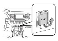
Connecting a compatible device and cable into the USB media port will support charging and music playback through the audio multimedia system.
