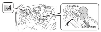
The initial shift range in "S" mode is set automatically to 5 or 4 according to vehicle speed.
