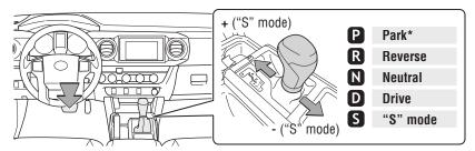
\*The engine switch must be in the "ON" position (without Smart Key) / "IGNITION ON" mode (with Smart Key) and the brake pedal depressed to shift from Park.
