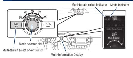
Improves driveability in off-road situations. Select one of five modes that most closely matches the terrain on which you are driving. Brake control can be optimized in accordance with the selected mode.
