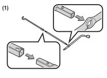
Insert the jack handle end into the lowering screw.
