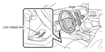
Hold wheel, push lever down, set angle and length, and return lever.
