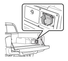
The power outlet can be used when the engine is running. *Refer to the Owner's Manual for more details.*
