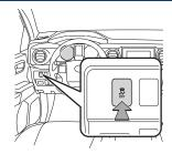
The VSC OFF switch is used to switch between modes related to the TRAC. VSC and Auto LSD functions.
