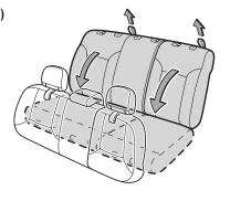
Pull lock release strap and fold down the seatback.
