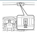
The active traction control system automatically helps prevent the spinning of four wheels when the vehicle is started or accelerated on slippery road surfaces.
