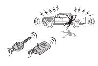
\* Driver door unlocking function can be programmed to unlock driver door only, or all doors. Grasping front passenger door handle will unlock all doors.
