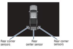
If the sensors detect an obstacle, the buzzer and MID display informs the driver of the approximate position and distance of the obstacle by illuminating continuously (far) or blinking (near). Depending on your Audio Multimedia System, you can adjust settings.
