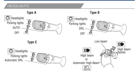
**Daytime Running Light (DRL) system** Automatically turns on under certain conditions to make vehicle more visible to other drivers. Not for use at night.
