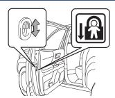
Moving the lever to "LOCK" will allow the door to be opened only from the outside.
