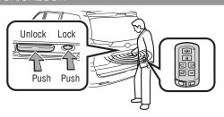
\* Driver door unlocking function can be programmed to unlock driver side doors only, or all doors. Grasping any passenger door handle will unlock all doors. Please refer to the Owner's Manual for more details on how to program the doors.
