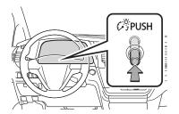
Pressing the button will adjust the brightness of the meter panel lights. The brightness level of the meters when the surroundings are bright (day mode) and dark (night mode) can be adjusted individually.
