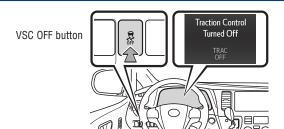
The VSC OFF switch can be used to help free a stuck vehicle in surroundings like mud, dirt or snow. While the vehicle is stopped, press switch to disable the TRAC system.
