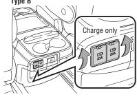
The ignition/"ENGINE START STOP" switch must be in "ACC" or "ON"/ACCESSORY or IGNITION ON position for use.
