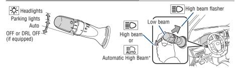
**Daytime Running Light (DRL) system (if equipped)** Automatically turns on under certain conditions to make vehicle more visible to other drivers. Not for use at night. **Automatic light cut off system** Automatically turns lights off after a delay of 30 seconds, or lock switch on remote is pushed after locking.
