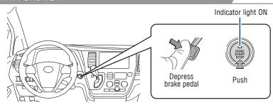
NOTE: The Smart Key must be carried to enable the start function. With gear shift lever in Park and the brake pedal depressed, push the "ENGINE START STOP" switch.
