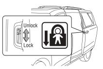
Moving the lever downward will allow the door to be opened only from the outside.
