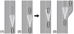
(1) Constant speed cruising when there are no vehicles ahead The vehicle travels at the speed set by the driver. The desired vehicle-to-vehicle distance can also be set by operating the vehicle-to-vehicle distance control.
