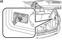
The ignition/"ENGINE START STOP" switch must be in "ON"/IGNITION ON position for use.
