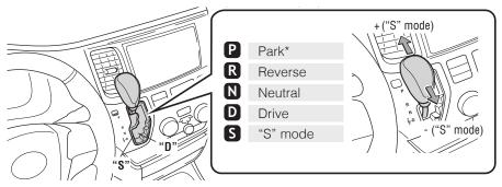
\* The "ENGINE START STOP" switch/ignition switch must be "ON" and the brake pedal depressed to shift from Park.
