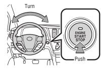
The green indicator light on the engine switch will flash and a message will be shown on the multi-information display. Press the engine switch while turning the steering wheel left and right.
