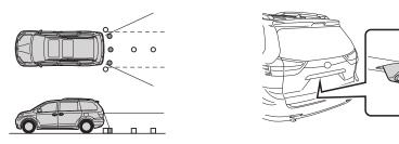
The rear view monitor system displays an image of the view from the bumper of the rear area of the vehicle. The camera for the rear view monitor system is located above the license plate.
