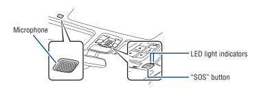
Safety Connect is a subscription-based telematics service that uses Global Positioning System (GPS) data and embedded cellular technology to provide safety and security features to subscribers. Safety Connect is supported by Toyota's designated response center, which operates 24 hours per day, 7 days per week.
