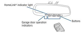
Garage door openers manufactured under license from HomeLink®\* can be programmed to operate garage doors, estate gates, security lighting, etc.
