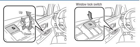
**All window auto up/down** Push the switch completely down or pull it completely up and release to fully open or close. To stop window partway, lightly push the switch in the opposite direction.
