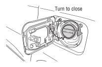
NOTE: Tighten until one click is heard. If the cap is not tightened enough, Check Engine " (Control of the control of the cap is not tightened enough, Check Engine " (Control of the cap is not tightened enough).
