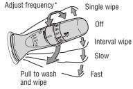
\* Rain-sensing windshield wiper Rotate to increase/decrease sensor sensitivity.
