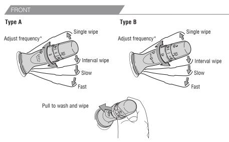
\* Intermittent windshield wiper frequency adjustment Rotate to increase/ decrease wipe frequency.
