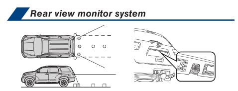
The rear view monitor system displays an image of the view from the bumper of the rear area of the vehicle. The camera for the rear view monitor system is located above the license plate.
