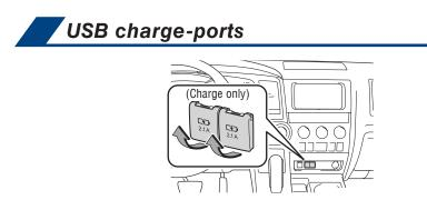
The engine switch must be in the "ACCESSORY" or IGNITION ON mode for use.
