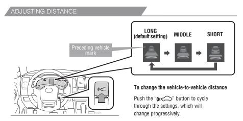
This mode employs a radar sensor to detect the presence of a preceding vehicle up to approximately 328 ft (100 m) ahead, determines the current vehicle-to-vehicle following distance and operates to maintain a preset following distance from the vehicle ahead. These distances vary based on vehicle speed.
