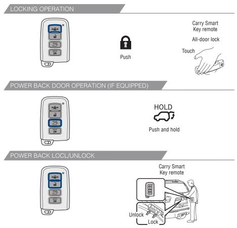
\* Driver door unlocking function can be programmed to unlock driver door only, or all doors. Grasping passenger door handle will unlock all doors.
