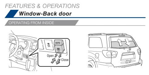
**Automatic operation** Push the switch completely in or pull it completely out and release to fully open or close. To stop window midway, lightly push the switch in the opposite direction.
