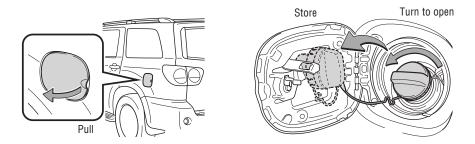
NOTE: To close, tighten until one click is heard. If the cap is not locked or tightened, Check Engine " $\overset{\text{H}}{_{\text{CHECK}}}$ " indicator may illuminate.
