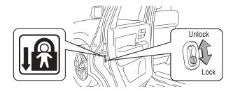
Moving the lever downward will allow the door to be opened only from the outside.
