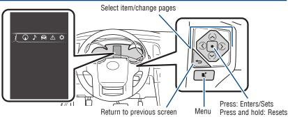
Use the meter control switches on the steering wheel to scroll through the following information screens:
