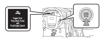
NOTE: The Smart Key must be carried to enable the start function. With the gear shift lever in Park and the brake pedal depressed, push the "ENGINE START STOP" switch.
