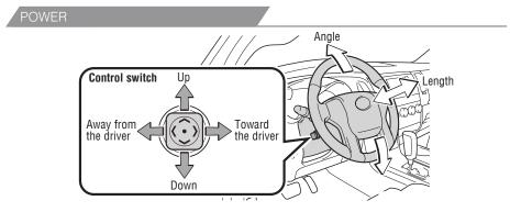
Toggle the control switch to set angle and length.
