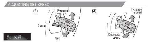
Vehicle will cruise at a set speed, decelerate to maintain selected distance from a slower vehicle traveling in front and accelerate back up to the selected speed if the vehicle in front changes lanes or speeds up.
