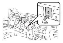
The VSC OFF switch is used to switch between modes related to the TRAC, VSC and AUTO LSD functions.
