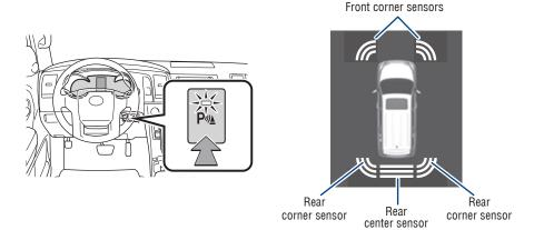
The parking assist sonar system operates when the vehicle approaches an obstacle. The distance from your vehicle to nearby obstacles when parallel parking or maneuvering into a garage is measured by sensors and communicated via the Multi-Information Display (MID) and audible beeps.
