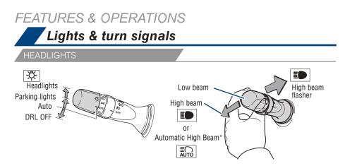
**Daytime Running Light system (DRL)** Automatically turns on under certain conditions to make vehicle more visible to other drivers. Not for use at night. **Automatic light cut off system** Automatically turns lights off after 30 second delay, or the lock switch on remote is pushed after locking.
