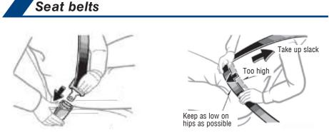
NOTE: If a passenger's seat belt is fully extended, then retracted even slightly, the Automatic locking retractor (ALR) will prevent it from being re-extended beyond that point, unless fully retracted again. This feature is used to help hold child restraint systems securely.
