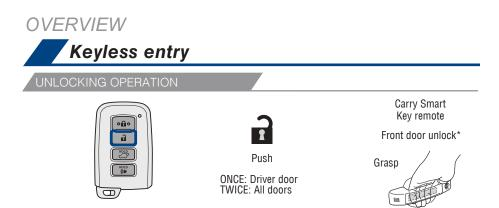
NOTE: If a door is not opened within 60 seconds of unlocking, all doors will relock for safety.
