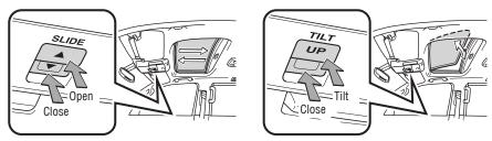
Lightly press either side of the moonroof switch while opening/tilting is in progress, the moonroof stops partway.
