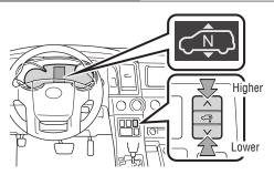
Vehicle height can be adjusted only when the engine is running.
