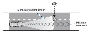
As part of the Pre-Collision System, this function is also designed to first provide an alert and then automatic braking if needed.
