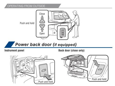
Open: Push and hold Close: Push and hold again NOTE: Door will stop closing if obstructed, or to manually stop door closing, push button again.
