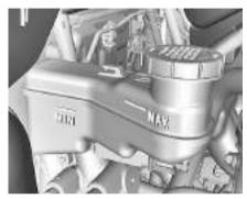
The level of the brake fluid should be between the 'MIN' and 'MAX' marks on the side of the brake fluid container. If the level falls below the 'MIN' mark, add recommended brake fluid.
