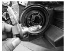
11. Refit position high beam bulb.
