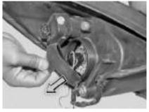
2. Press the pin and pull the connector from the bulb.
