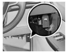
3. Raise the bonnet slightly and with your finger slide the secondary lock lever located under the bonnet centre to the left side.
