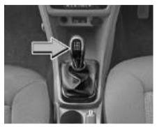
The gearshift pattern is as shown on the gear lever knob. Gear shifting should always be done with clutch pedal pressed.
