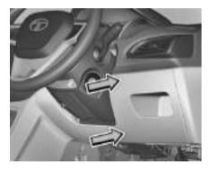
2. To remove the cover, gently pull the cover from bottom side such that the lugs get disengaged.
