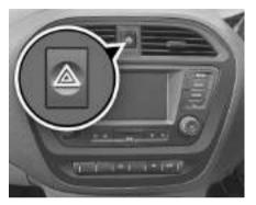
Press the hazard warning switch to activate the hazard warning. All the turn signal lamps will flash simultaneously. To turn OFF, press the switch again.
