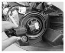
9. Unlock position high beam bulb from its place
