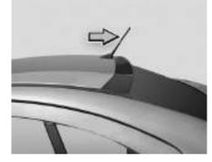
Antenna is located on the roof. Turn antenna counter clockwise to remove from vehicle, if required.
