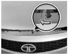
4. Lift the bonnet up. Pull the bonnet stay rod from its clip and insert the free end into the slot.
