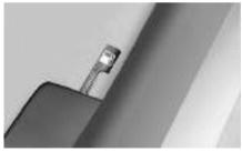
Fuel lid opening Lever is located on the right hand side of the driver seat. Lift the lever to unlock fuel flap. Open the fuel cap by turning it in counter clockwise direction for fuel filling.
