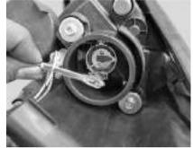
6. Refit low beam bulb by locking high beam bulb holder clip.
