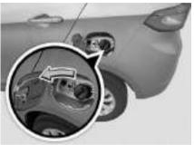
For closing, lock the fuel cap and gently push the fuel flap till it gets locked.
