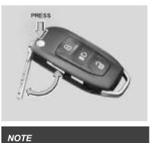
Key Blade should not be folded without pressing the button. Also, it should not be forced in any direction apart from folding direction to avoid damage to Flip Mechanism.
