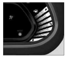
When fuel in the tank is near to empty position, low fuel warning telltale turns 'ON'. Refill the tank as soon as possible.
