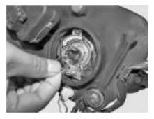
4. Pull out the bulb from the socket.
