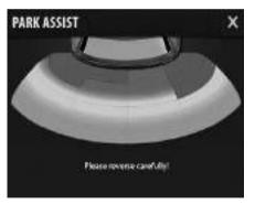
There are 4/3 ultrasonic sensors placed on the rear bumper of the vehicle. Once the system is activated, the sensors will detect the proximity of an obstacle from the bumper, and this information would be displayed on the vehicles infotainment system. In Low variants, only audio warning shall be given through a buzzer.
