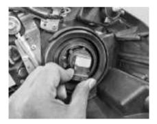
10. Remove position high beam bulb
