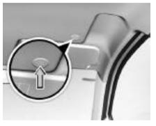
A mic is provided on roof interior above driver seat position.
