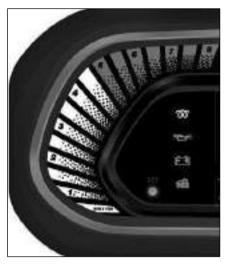
Tachometer indicates engine speed in revolutions per min (rpm).
