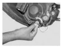
Replace with the new bulb (refer bulb specification table) and refit it by pressing and turning in clockwise direction firmly into the socket.
