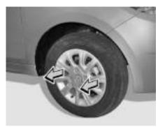
Insert a piece of cloth between the spokes of the wheel cover and pull it outwards. Take out detached wheel cover from the wheel rim.
