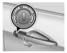
Insert the key and turn it clockwise to lock and counter clockwise to open the door.
