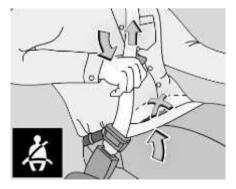
To unlatch the belt, press the red button on the buckle. Guide the belt to the pillar as it retracts.
