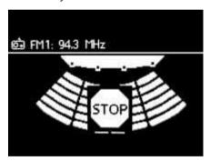
There are 4 ultrasonic sensors placed on the rear bumper of the vehicle. Once the system is activated, the sensors will detect the proximity of an obstacle from the bumper, and this information would be displayed on the vehicles infotainment system.
