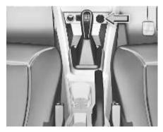
The power socket will work when the ignition switch is in the "ACC" or "ON" position. This socket can be used to provide 12V (10A) power for electrical accessories.
