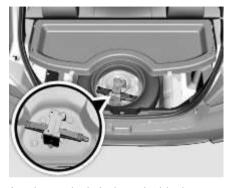
A scissors jack is kept inside luggage compartment below the spare wheel. Jack handle is kept in the tool kit bag.
