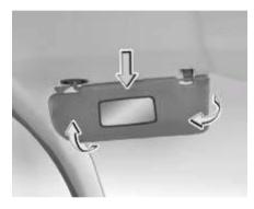
The sun visors can be pulled down to block glare coming through the wind-shield.
