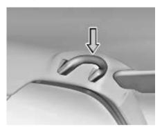
Roof grab handles are provided on all seats except driver's seat. This helps in comfortable positioning of passengers during a journey.
