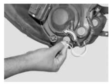
Replace with the new bulb (refer bulb specification table) and refit it by pressing and turning in clockwise direction firmly into the socket.
