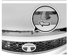
4. Lift the bonnet up. Pull the bonnet stay rod from its clip and insert the free end into the slot.
