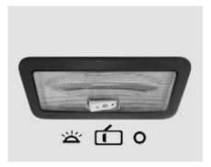
Interior roof lighting lamp is provided on the roof with inbuilt switch.
