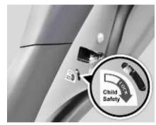
Both the rear doors of the vehicle are provided with a child proof lock. Push the lock lever located on vertical face of the door downward before closing the door. The door which has been locked by activating the child lock cannot be opened from inside, it can be opened only from the outside.
