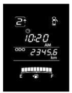
Digital clock appears on the DIS screen. To adjust the values in Hrs. Min. and AM/PM mode, Press 'SET' knob on Instrument Cluster. A delayed press on the 'SET' knob for selected value will confirm it and move towards next respective value.
