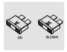
Remove the blown fuse by "fuse puller". The fuse puller and spare fuses are provided in the engine compartment fuse box.
