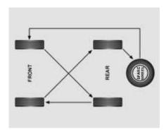
For 175/65 R14 alloy wheel rims with spare wheel of steel wheel rim (if equipped)
