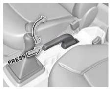
Mechanical parking brake acting only on the rear wheels is provided on the vehicle. To apply the parking brake, pull the lever up fully. The parking brakes telltale illuminates on the instrument cluster. To release it, pull the lever up slightly, press the release button and push the lever down. Parking brakes telltale on the instrument cluster will turn 'OFF' when the lever is fully released.
