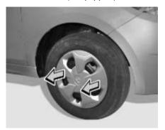
Insert a piece of cloth between the spokes of the wheel cover and pull it outwards. Take out detached wheel cover from the wheel rim.
