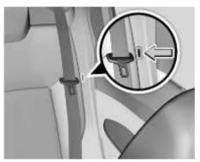
Insert the rear seat belt tongue (except middle seat) in the slit (shown in fig.) provided when not in use or during seat folding.
