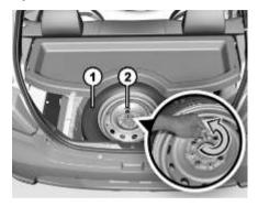
1. Spare Wheel 2. Retaining bolt
