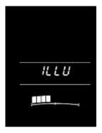
For Instrument Cluster illumination level settings, it is necessary to turn the Park Lamp 'ON' and then Press the 'SET' knob on Instrument Cluster.
