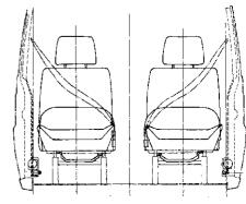
Seat-belt Arrangement on Driver & Co-driver's Seat
