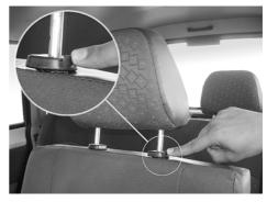
Release Button for Head rest height adjustment
