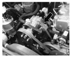
Power Steering Pump Belt Adjustment Nut
