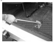
Loosening/Tightening of wheel winch screw
