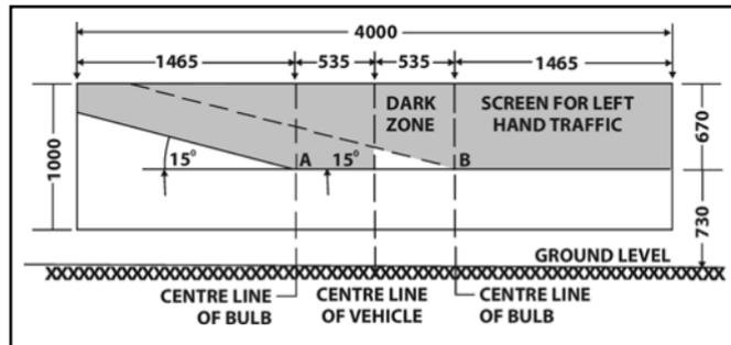
When properly adjusted, most brightly illuminated area will be just below the intersection point 'A' of these two lines.
