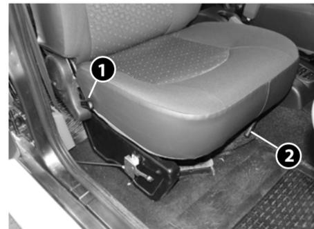
1. Seat backrest inclination adjustment lever
