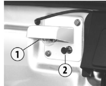
*1. Engine Compartment Lamp 2. ON / OFF Switch*
