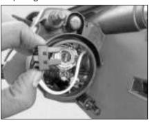
4. Remove high beam bulb.
