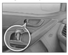
All the doors can also be locked from inside by pressing knob on driver door and independently on other doors respectively.
