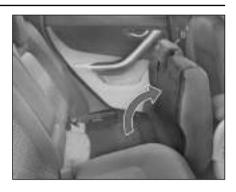
Pull the backrest release knobs upwards
