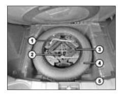
Tool kit, tow hook, jack and spare wheel are provided in rear boot.
