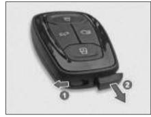
Slide the knob (1) to unlatch the key. Pull the key blade (2) out.
