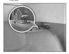
Fold the backrest seat forward. Move the driver and co-driver seat forward if necessary.
