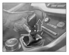
For engaging reverse gear, lift the latch and keeping latch lifted, shift to reverse position.
