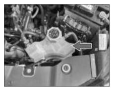
Check whether the coolant level is between the 'MIN' and 'MAX' marks provided on the coolant reservoir.
