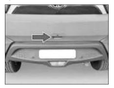
If vehicle is locked and Tail gate is closed and Tail gate DHS switch is pressed with valid smart key in the authentication range, Tail gate gets unlatched.
