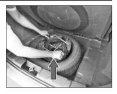
To remove the spare wheel, unscrew and remove the retaining bolt.
