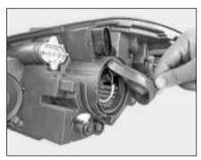
Press the pin and pull the connector from the bulb.
