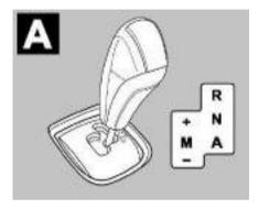
Auto mode will be engaged only when vehicle is stationary and brake pedal pressed. An audio signal indicates when Automatic gear is engaged. May will be indicated in instrument cluster.
