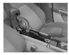
Tambour door is provided on center console. To access Tambour door, lift arm rest (1). Slide the shutter (2) to open and close the stowage area.
