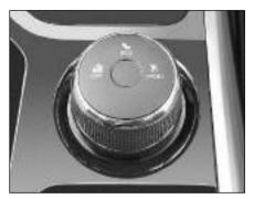
'ECO', 'CITY' and 'SPORT' drive modes are provided. These modes can be used to adjust engine characteristics and vehicle performance in line with desired requirement.
