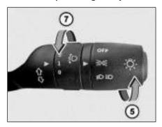
Inner rotary switch on right hand stalk is provided for head lamp leveling. With the inner rotary switch, Head lamp leveling can be done with head lamp in Low Beam and in 'ON' position. Select correct position before start of trip and vehicle is stationary. Depending upon the number of passengers and luggage in the vehicle headlamp focus may change. This can be adjusted by rotating the knob to one of the 3 level positions.
