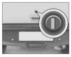
Tail gate opened by using door key, the lock is located on the Tail gate.
