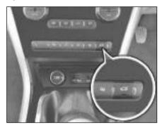
To open the Tail gate, press the switch located on fascia switch.
