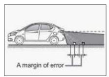
When any part of the vehicle sags due to the number of passengers or the distribution of the load, there is a margin of error between the fixed guide lines on the screen and the actual distance/course on the road.
