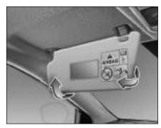
The sun visors can be pulled down to block the glare coming through the windshield.
