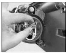
3. Unlock high beam bulb holder clip, by pulling it backward.
