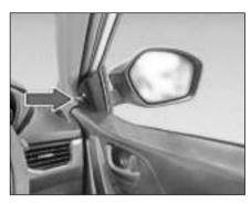
You can adjust the outer rear view mirrors manually by joy stick knob located in the driver's and front passenger's door panel.
