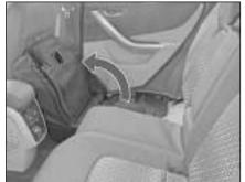
Pull the backrest release knobs upwards.
