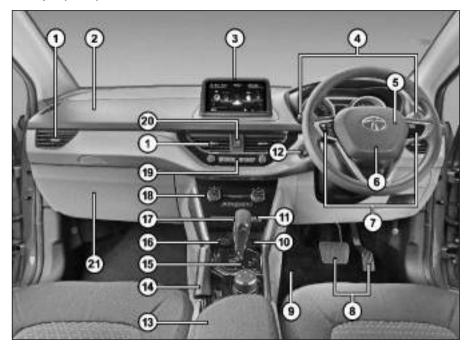
A.C. Air vent Air Bag (PAB) (if fitted) Infotainment Display (if fitted) Combi-Switch Horn pad 6 Air Bag (DAB) (if fitted) Steering Wheel Switches (if fitted) 8 Controls Foot Rest 9 USB/AUX Port 10 Fascia switches 11 Start/Stop switch 12 Foldable Arm-Rest (if fitted) 13 Parking Brake Lever 14 Drive Control knob 15 Power socket 16 Gear Shift Lever 17 **HVAC Control panel** 18 19 Infotainment Switches 20 Hazard Warning Switch Glove Box 21
