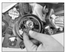
4. To free the headlamp bulb from the socket, press and swing the retaining spring and pull it straight back.
