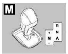
Shift gear lever to left for engaging manual mode. An audio signal indicates when manual mode is engaged. M will be indicated in instrument cluster.
