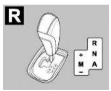
Reverse gear will be engaged only when vehicle is stationary and brake pedal pressed. An audio signal indicates when reverse gear is engaged. will be indicated on instrument cluster.
