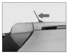
Antenna is located on the roof. Turn antenna anticlockwise to remove from vehicle, if required.
