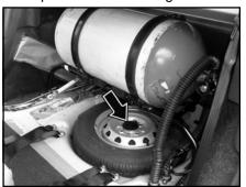
Once this nut is removed, the wheel can be lifted and taken out.
