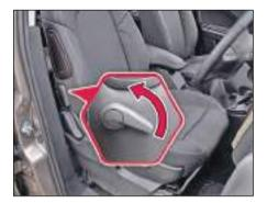
Continuous (Multiple adjusting position) lumbar support is provided on driver and front passenger seat to give you comfort while driving. It is adjusted by the lever provided on the side of the seat backrest.
