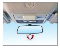
To adjust the mirror, set the selector tab to the normal or antiglare position and then move the mirror up, down or sideways manually to obtain the best rear view.
