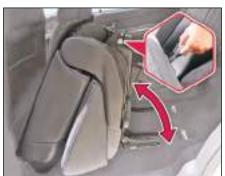
The second row seat can be tumbled from its base by pulling the fabric hook located behind the seat's back.
