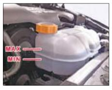
Check the coolant level when the vehicle is on a level surface and the engine has cooled down.
