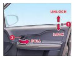
All the doors can also be locked from inside by pressing knob (1) on driver door and independently on other respective doors.
