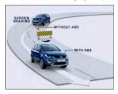
ABS regulates brake pressure in such a way that the wheels do not lock when you brake.
