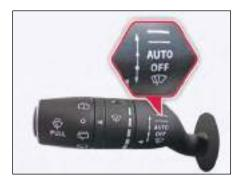
The wiper stalk will also provide five rain sensitivity/frequency settings to allow you to select the sensitivity of the auto wipe system,
