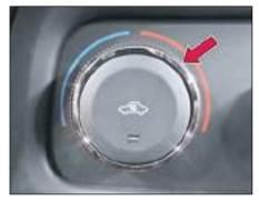
The temperature control dial allows you to adjust the temperature. Turn the dial counter-clockwise to lower the temperature. To increase the temperature, turn the dial in clockwise direction.
