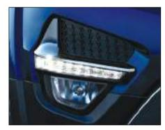
Day time Running Lamps (DRL) are used to increase the visibility of the vehicle to other drivers during daytime.
