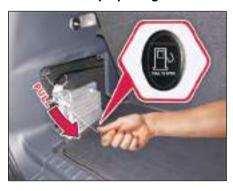
Alternatively, you can also open the fuel flap manually by following the below steps:
