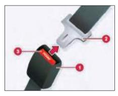
Make sure that the seat belt is fully rolled up. Otherwise, the seat belt or belt tongue will be trapped in the door or in the seat mechanism. This could damage the door, the door trim panel and the seat belt. Damaged seat belts can no longer fulfill their protective function and must be replaced. Visit a TATA MOTORS Authorized Service Centre.
