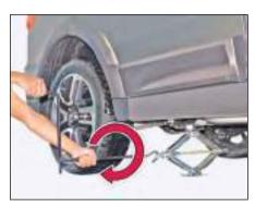
Remove wheel-mounting nuts and take out the flat tyre.
