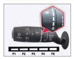
These will vary the amount of rain that must be detected by the rain light sensor before the auto wipe system turns 'ON'. The speed of wiping will be varied depending on the intensity / frequency of rain falling.
