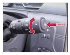
By rotating the outermost ring of the Combi Switch, you can set the TRIP, FUEL and SET functions that are displayed on the instrument cluster. To reset/scroll the values, press the outermost selector switch on the stalk.
