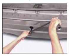
Rotate the handle counter-clockwise to lower the spare wheel till it rests on the ground.
