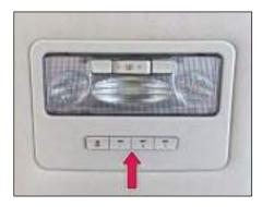
Separate auxiliary unit is provided for rear AC.
