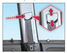
Adjust the height of seat belt shoulder section according to your comfort.
