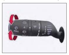
Turn the outer rotary knob such that it aligns its position with arrow mark and hold it, to operate rear windshield wash and wipe.
