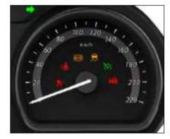
Speedometer indicates the actual vehicle speed in km/h.
