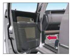
Access the Inertia switch through cutout (opening) and press it.
