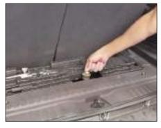
Remove the window cover provided on the rear bumper to access the spare wheel bracket.
