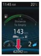
Odometer indicates total distance traveled by vehicle up to 999999 km with the resolution of 1 km.
