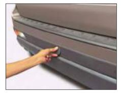
➤ Insert the spare wheel handle with extension through the window.
