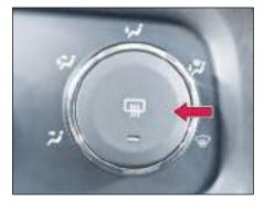
Press the button to turn ON the rear windshield and outside rear view mirror (if equipped) demister. This clears the fog / mist formation.
