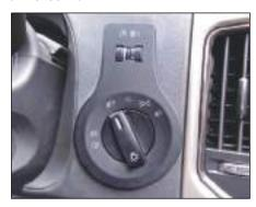
Automatic Headlamp mode is activated if Master Light switch is in auto mode.
