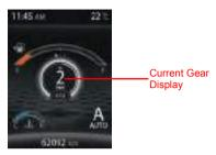
Current Gear number displayed on the DIS screen based on gear shift lever position when clutch pedal is fully released.
