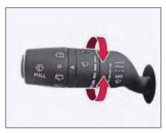
Inner rotary switch on left hand stalk is provided for intermittent front wiper delay. The switch has 5 delay timers.
