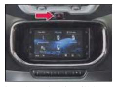
Press the hazard warning switch to activate the hazard warning. All turn signal lamps and their tell tales will start flashing simultaneously. To turn it off, press the switch again.
