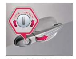
All doors can be locked / unlocked manually from outside using driver door key slot. Insert the mechanical key and turn it clockwise to lock and counter clockwise to open the doors.
