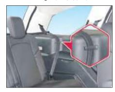
When second or third row seat is not occupied, hook the seat belts at its respective belt hanger to avoid rattling. Make sure the belt webbing is not twisted.
