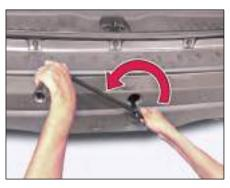
Remove the holding bracket from the spare wheel and get the spare wheel separated.
