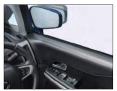
Outer rear view mirrors can be folded by operating the mirror fold switch (3). This enables you to park your vehicle in limited parking space. Press the mirror fold switch to fold both outside mirrors simultaneously. Press again to unfold.
