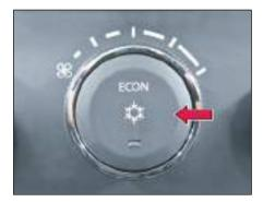
Press the switch to activate / deactivate the climate control. The indicator lamp in the button will light up when climate control is activated.
