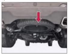
Open the tail gate and storage box lid, remove the anti-theft rubber lock.
