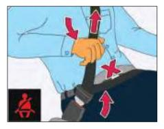
To unlatch the belt, press the red button on the buckle. Guide the belt to the pillar as it retracts.
