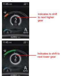
Gear Up/Down recommender shall recommend the user to change the gears for better performance.
