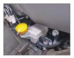
The level of the brake fluid should be between the 'MIN' and 'MAX' marks on the side of the brake fluid container. If the level falls below the 'MIN' mark, top up with recommended brake fluid.
