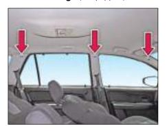
Curtain air bags are integrated into the side of the roof frame and deployed in the area from the  $1^{st}$  row seat to the  $2^{nd}$  row seat.
