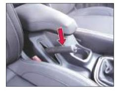
Parking brake lever is provided between the driver and co-driver seat on the floor console.
