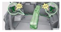
The carabiners on the two sides latch into the lashing eyes.
