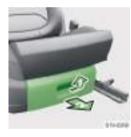
The maximum permissible load for the storage compartment is 1.5 kg.
