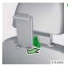
Press the safety button and unfold the holder.
