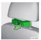
> Place the open adapter on the front guide rods of the headrest and clip in carefully.
