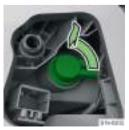
> Turn and remove the socket with the bulb.
