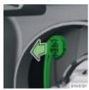
Remove the base with the bulb.
