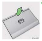
With the ignition switched on, press the brake pedal and at the same time push the (D) button.
