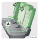
Pull on the loop A and adjust the inclination of the seat backrests.
