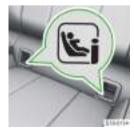
Holding eyelets for installing the child seat using the ISOFIX system.
