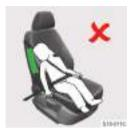
The child should not be in the deployment area of the side airbag.
