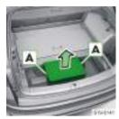
Remove the battery cover using the handles A.
