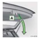
Grasp the fixture A and pull the lid down.
