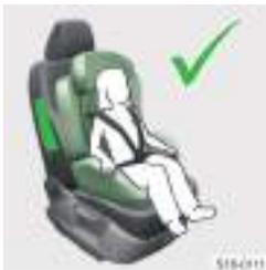
There must be enough room between the child and the exit area of the side airbag for the side airbag to offer the best possible protection.
