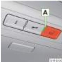
The system state is displayed after the ignition is switched on by the warning light **A** illuminating.
