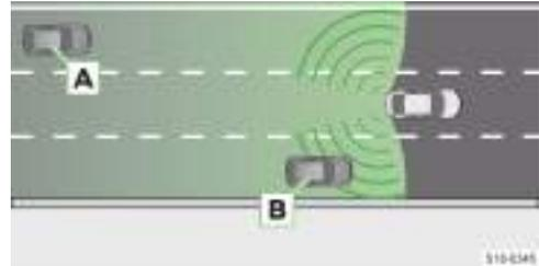
Your vehicle is overtaken by vehicle **A**. The faster vehicle **A** approaches, the sooner the warning is given by the indicator light.
