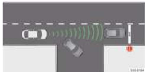
If a vehicle in front turns and there is a stationary vehicle in front of this vehicle, the ACC will not respond to the stationary vehicle.
