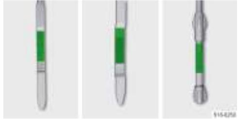
The oil level must be within the marked range.
