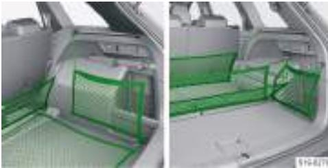
The maximum load of the respective fastening nets is 1.5 kg.
