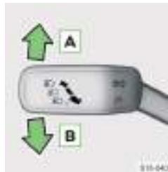
**A** Switching on the indicator light on the right - the warning light flashes in the instrument cluster
