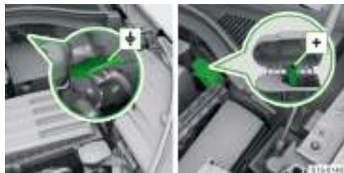
Engine compartment: Earth point and  $\oplus$  pole on vehicles with the battery in the luggage compartment
