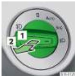
Positions for pulling out the light switch
