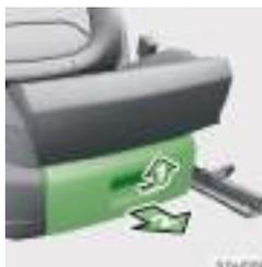
The maximum permissible load for the storage compartment is 1.5 kg.
