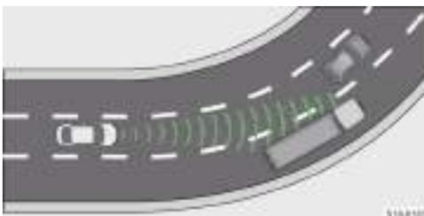
When cornering, a vehicle in the next lane may enter the detected area. Your vehicle will be controlled according to this vehicle.
