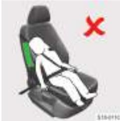
The child should not be in the deployment area of the side airbag.
