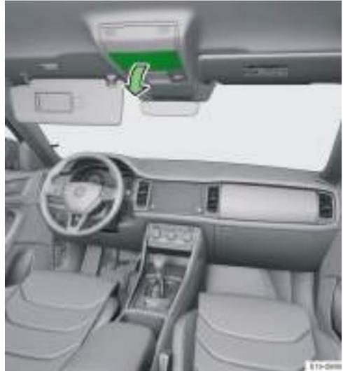
The maximum load for the compartment is 0.25 kg.
