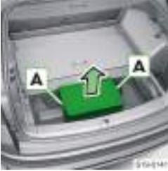
Access to the vehicle battery in the luggage compartment
