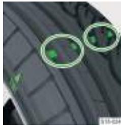
Wear indicators are located in the profile of the tyres that display the permissible minimum tread depth.
