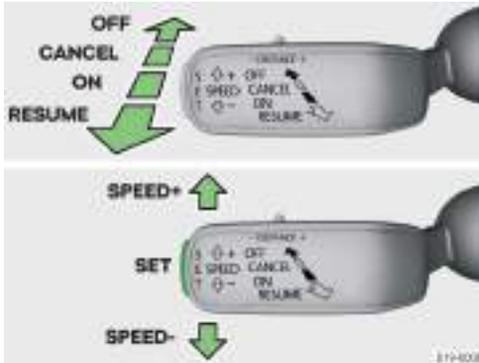
**ON** Activate ACC (condition for the subsequent activation of the limiter). To enable the speed limiter, press the key and in the instrument cluster choose the menu item *Speed limit*.
