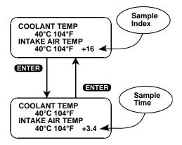
The sample time display gives the time in seconds (relative to the trigger sample) at which the tester received the currently displayed sample. For example, a sample time of +3.4 means the sample was received 3.4 seconds after the trigger sample. A sample time of -2.6 seconds means the sample was received 2.6 seconds before the trigger.
