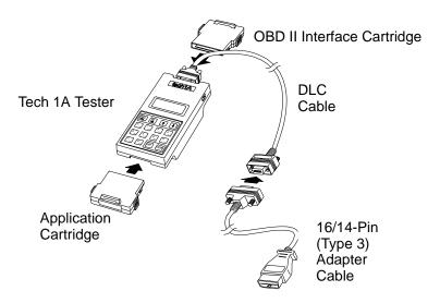
FIGURE 2-2. Tech 1A ABS Delphi Brake Control 7 with 16-Pin Connector (OBD II)
