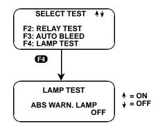
FIGURE 5-15. Lamp Test (ABS DBC7)
