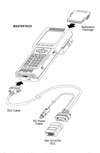
FIGURE 2-4. MTS 3100 ABS/Airbag with 12-Pin Connector
