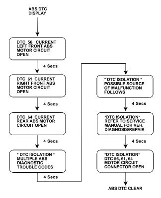
FIGURE 5-4. Example of ABS Fault Isolation
