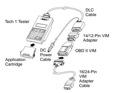
FIGURE 2-3. Tech 1ABS Delphi Brake Control 7 with 16-Pin Connector (OBD II)
