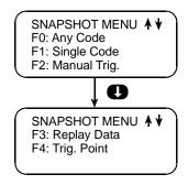
Selecting F0: Any Code or F2: Manual Trigger causes the tester to proceed directly to the DATA CAPTURE phase of the SNAPSHOT mode.
