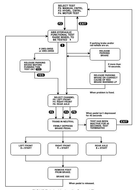
FIGURE 5-9. Hydraulic Control Test
