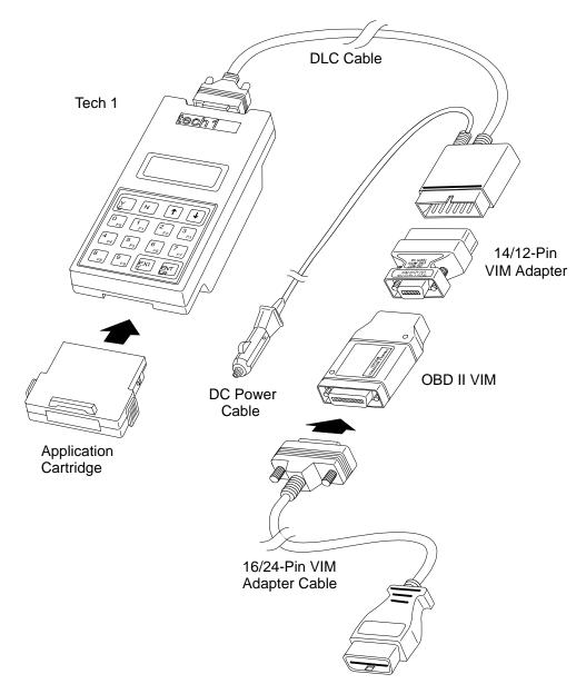
FIGURE 2-3. Tech 1 Adapter and Cables
