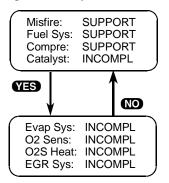
The first three items on the display indicate the vehicle's monitoring capability for continuously monitored systems:
