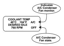
A/C Condenser Fan Control Mode Screen
