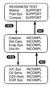
The first three items on the display indicate the vehicle's monitoring capability for continuously monitored systems:
