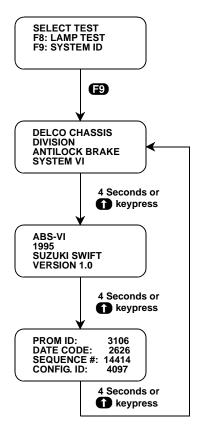
FIGURE 5-12. Examples of System ID Displays
