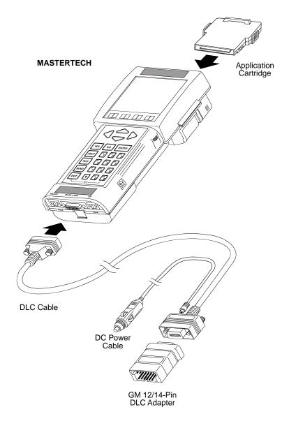
FIGURE 2-1. MTS 3100 Adapter and Cables
