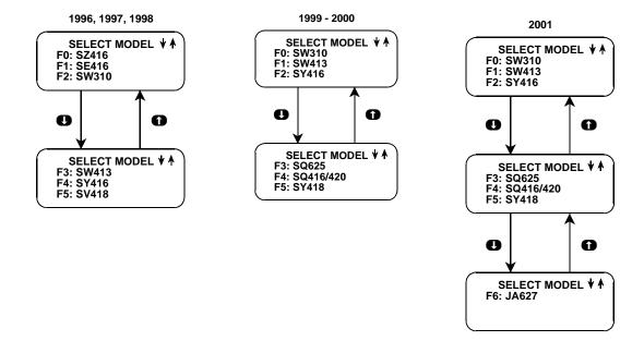
Press the function key corresponding to the model of the vehicle being tested. More information about each model and model year is included in Chapter 1.
