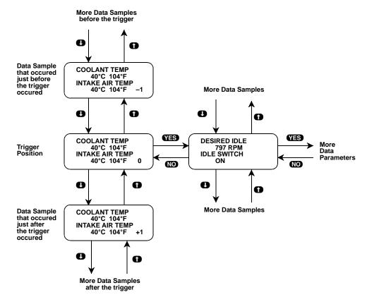
10. While in the data display phase, pressing **ENTER** will cause the tester to toggle between the sample index and sample time.
