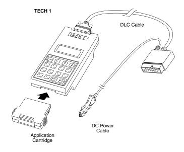
FIGURE 2-6. Tech 1 ABS/Airbag with 12-Pin Connector
