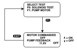
FIGURE 5-13. Pump Motor Test
