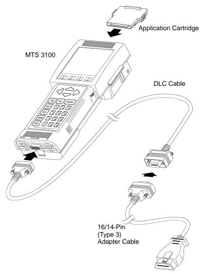
FIGURE 2-1. MTS 3100 Adapter and Cables
