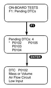
A pending DTC description can be displayed for any Pending DTC by moving the \* next to the desired DTC and pressing **ENTER**.
