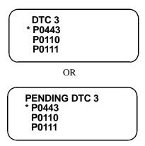
A DTC description can be displayed for any DTC by moving the \* next to the desired DTC and pressing **ENTER**. The \* is moved by pressing the 1 or 1 keys.
