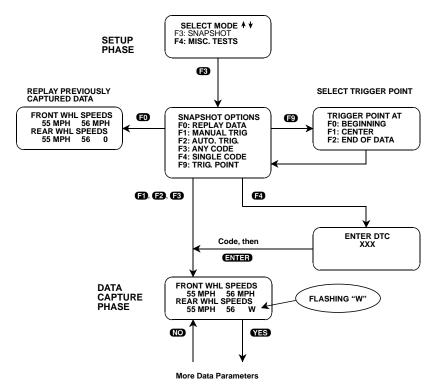
FIGURE 5-5. Snapshot Setup Phase
