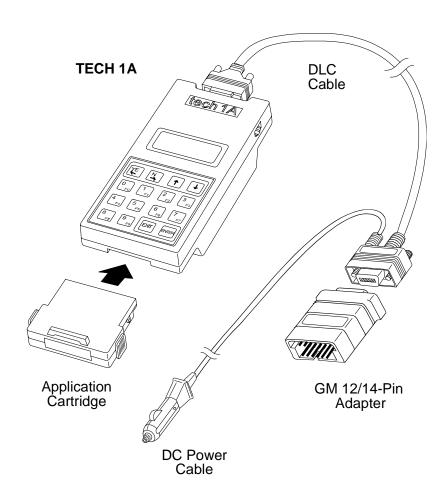
FIGURE 2-2. Tech 1A Cable Configuration
