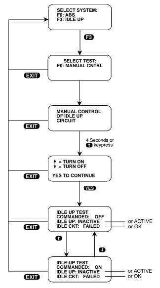
FIGURE 5-10. Idle Up Test
