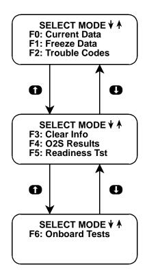
Select the desired function by pressing the key indicated to the left of the function.
