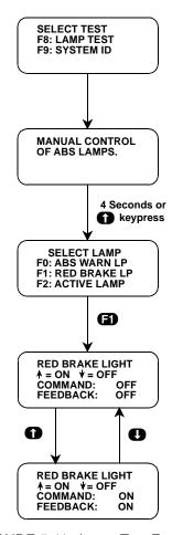
FIGURE 5-11. Lamp Test Example
