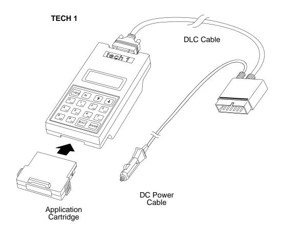
FIGURE 2-3. Tech 1 Cable Configuration
