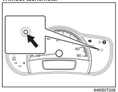
This light will blink with the ignition switch in the "LOCK" or "ACC" position. The blinking light is intended to deter theft by leading others to believe that the vehicle is equipped with a security system.
