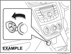
The accessory socket will work when the ignition switch is in the "ACC" or "ON" position. This socket can be used to provide 12 volt/120 watt power for electrical accessories.
