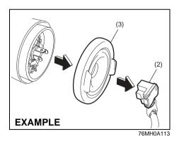
1) Open the engine hood. Disconnect the coupler (2). Remove the sealing rubber
