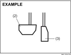
Do not drive with your foot resting on the clutch pedal. It could result in excessive clutch wear, clutch damage, or unexpected loss of engine braking.
