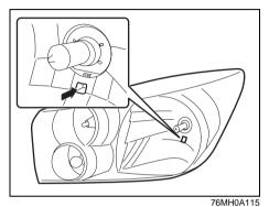
NOTE: You can see the position of retaining spring from the hole of headlight.
