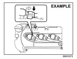
For nickel spark plugs (traditional type): You should inspect spark plugs periodically for carbon deposits. When carbon accumulates on a spark plug, a strong spark may not be produced. Remove carbon deposits with a wire or pin and adjust the spark plug gap.
