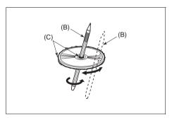
New discs may have some roughness around the edges. The unit may not work or the sound may skip if such discs are used. Use a ball-point pen (B), etc. to remove the roughness (C) from the edges of the disc before inserting it into the unit.
