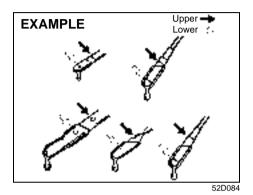
Pull out the oil dipstick, wipe oil off with a clean cloth, insert the dipstick all the way into the engine, then remove it again. The oil on the stick should be between the upper and lower limits shown on the stick. If the oil level indication is near the lower limit, add enough oil to raise the level to the upper limit.
