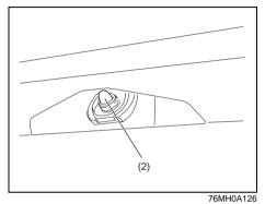
2) To remove and install the bulb of the license plate light (2), simply pull out or push in the bulb.
