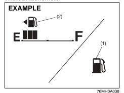
When the ignition switch is in the "ON" position, this gauge gives an approximate indication of the amount of fuel in the fuel tank. "F" stands for full and "E" stands for empty.
