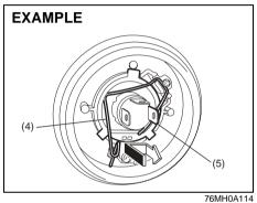
2) Push the retaining spring (4) forward and unhook it. Then remove the bulb (5). Install a new bulb in the reverse order of removal.
