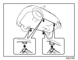
6) Position the jack vertically and raise the jack by turning the jack handle clockwise until the jack head groove fits around the jacking bar beneath the vehicle body. See illustrations.  Continue to raise the jack slowly and smoothly until the tire clears the ground. Do not raise the vehicle more than necessary.
