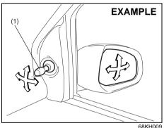
You can adjust the outside rearview mirrors by hand with the knob (1) located on the driver's or front passenger's door panel.
