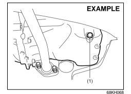
Tightening torque for drain plug (1): 35 Nm (3.6 kg-m, 25.8 lb-ft)
