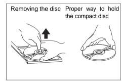
To remove the compact disc from its storage case, press down on the center of the case and lift the disc out, holding it carefully by the edges.
