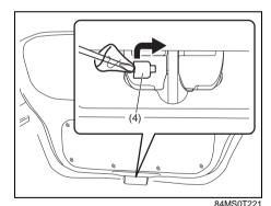
2) Open the tailgate latch cover (4) by using a flat blade screwdriver covered with a soft cloth as shown in the illustration.
