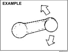
Raise or lower the door windows by turning the handle located on the door panel.
