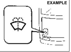
Check that there is washer fluid in the tank. Refill it if necessary. Use a good quality windshield washer fluid, diluted with water as necessary.
