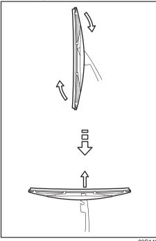
NOTE: Do not flex the wiper blade frame end more than necessary. If you do, it can break off.
