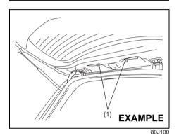
1) Open the tailgate, and remove the nuts (1) as shown in the illustration.
