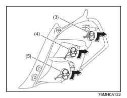
2) To remove the bulb holder of the tail/ brake light (3), the turn signal light (4) or the reversing light (5) from the light housing, turn the holder counterclockwise and pull it out.
