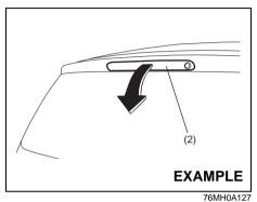
2) Close the tailgate. Remove the high-mount stop light housing (2) from the tailgate.
