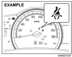
When the driver doesn't buckle his or her seat belt with the ignition switch in the "ON" position, the driver's seat belt reminder light in the instrument cluster will blink until the driver's seat belt is buckled.
