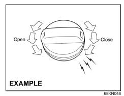
To remove the fuel filler cap:
