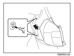
NOTE: When reinstalling the light housing, make sure the clips are properly attached.
