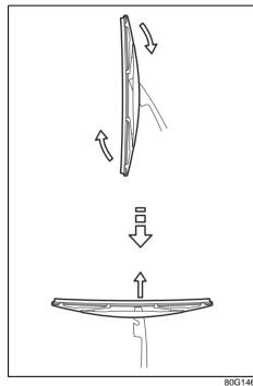
NOTE: Do not flex the wiper blade frame end more than necessary. If you do, it can break off.
