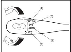
To turn the lights on or off, twist the knob on the end of the lever. There are four positions:
