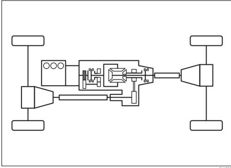
In this position, engine power is not supplied to the front or rear axles. Only use this position for towing your vehicle. When you turn the transfer switch to the "N" position, "N" indicator will come on with
