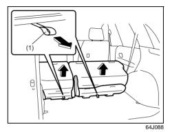
5) Pull the lock release strap (1) rearward to unlatch the seat cushion.
