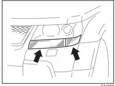
To replace the bulb of position/turn signal light, follow the procedure for the bulb replacement of the "Front Fog Light".
