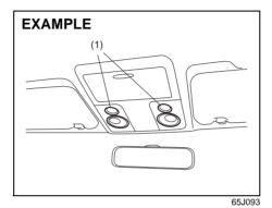
Push the switch (1) to turn on the light and push it again to turn off the light.
