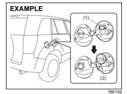
The cap holder (1) can hold the fuel filler cap (2) when refueling.
