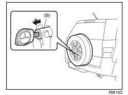
Pull out the lock cover (B) fitted on the lock nut of the spare wheel while inserting the key full into the key hole of the lock cover (B).
