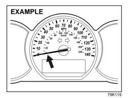
The speedometer indicates vehicle speed in km/h and mph.
