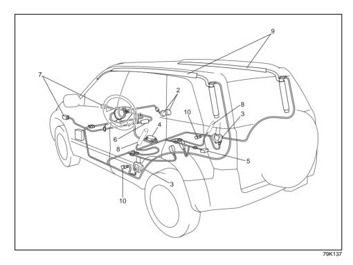
Your vehicle is equipped with a Supplemental Restraint System consisting of the following components in addition to a lapshoulder belt at each front seating position.
