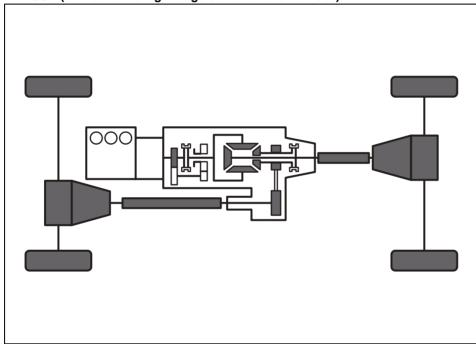
In this position, engine power is supplied to the front and rear axles and you get better traction than when driving in "4H". Use this position when you need better traction than "4H" provides, such as when driving on slippery roads etc.
