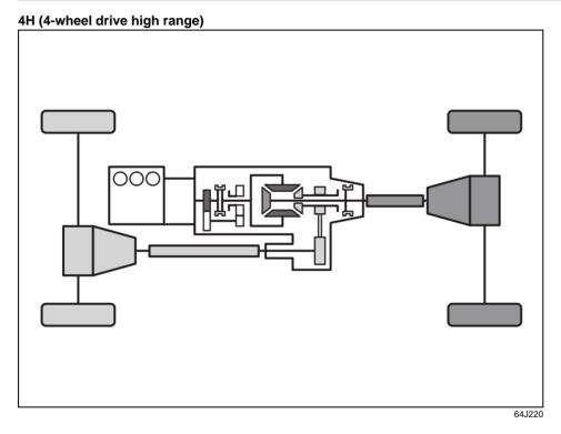
In this position, engine power is supplied to the front and rear axles. Use this position for normal driving.
