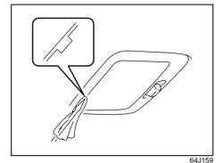
Pull down the lens by using a flat blade screwdriver covered with a soft cloth as
