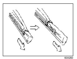
Pull the locked end of the wiper blade firmly to unlock the blade and slide the blade out as shown.
