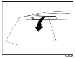
3) Close the tailgate. Remove a highmounted stop light housing (2) from the tailgate.
