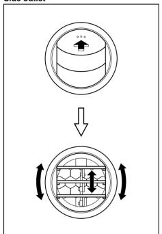
When "Open", air comes out from the side outlets regardless of the air flow selector position.
