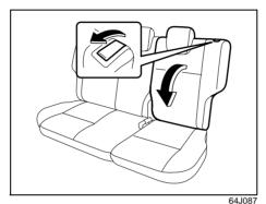
Pull the release lever forward on the top of each split seat, and fold the seatbacks forward.
