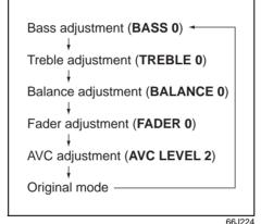
2) Turn the tone/balance/fader control knob (2) to adjust the sound.
