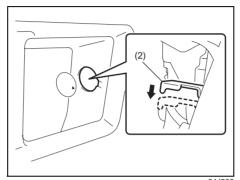
5) Push down on the emergency lever (2) using a jack handle or a flat blade screwdriver. To lock the tailgate, push up on the emergency lever (2).
