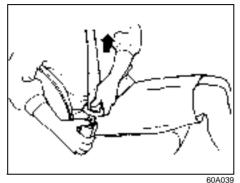
To unfasten the belt, push the red "PRESS" button on the buckle and allow the belt to retract.
