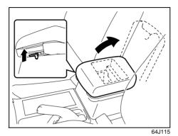
To use the console bin, pull the lever up and open the lid.
