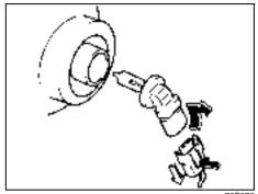
4) Open the fender cover. Disconnect the coupler with pushing the lock release. Turn the bulb holder counterclockwise and remove it.
