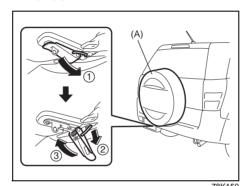
2) Release the lock at the underneath of the spare wheel full cover (A) as shown in the illustration.
