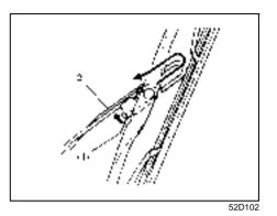
Squeeze lock lever (1) towards wiper arm (2) and remove the wiper frame from the arm as shown.
