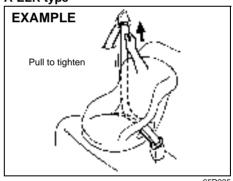
4) Try moving the child restraint system in all directions, to make sure it is securely installed. If you need to tighten the belt, pull more webbing toward the retractor.
