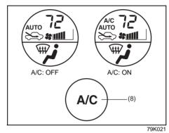
The air conditioning switch (8) is used to turn on and off the air conditioning system. To turn on the air conditioning system, push in the switch and "A/C" will appear on the LCD display. To turn off the air conditioning system, push in the switch again and "A/C" will go off.
