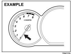
The tachometer indicates engine speed in revolutions per minute.
