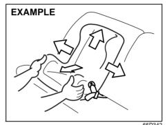
Make sure the child restraint is securely fastened by trying to move the child restraint system in all directions, especially forward.
