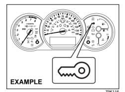
If the remote controller is not in the vehicle under the following conditions, a buzzer sounds intermittently for about 2 seconds and the keyless start system indicator light on the instrument cluster blinks in red:
