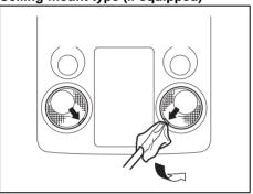
Remove the bulb holder by turning it counterclockwise. Pull out the bulb.
