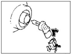
Open the engine hood. Disconnect the coupler while pushing the lock release. Turn the bulb holder counterclockwise to remove it.
