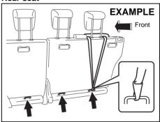
Some child restraint systems require the use of a top strap. Top strap anchor brackets are located on the back of the rear seat as shown in the illustration. Install the child restraint system as follows:
