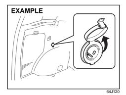
The accessory socket will work when the ignition switch is in the "ACC" or "ON" position.
