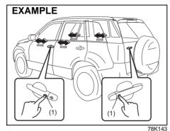
When the remote controller is within the operating range described in this section, you can lock or unlock the doors by pushing the request switch (1) on the door handle of each door or the tailgate.
