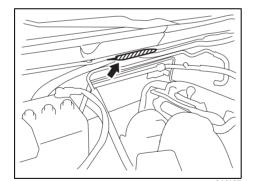
The Vehicle Identification Number (VIN) may be found in the two locations shown in the above illustrations. This number is used to register the vehicle. It is also used to assist your dealer when ordering parts or referring to special service information.
