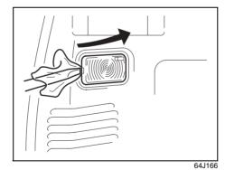
**High-mount stop light (if equipped)**The followings are the general procedure for replace the bulbs of high-mount stop light.
