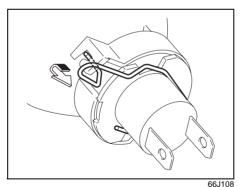
Open the engine hood. Disconnect the coupler. Remove the sealing rubber.
