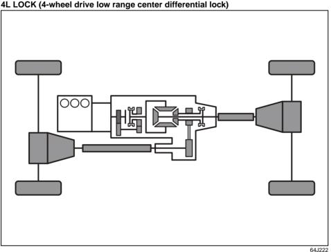
In this position, engine power is supplied to the front and rear axles and you get better traction and more low-speed torque than when driving in "4H". Use this position when you need better traction than "4H" provides and more low-speed torque than "4H LOCK" provides, such as when climbing or descending steep, slippery hills etc.
