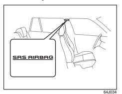
Side curtain air bags are located in the roof lining. The words "SRS AIRBAG" are molded into the pillar to identify the location of the side curtain air bags.
