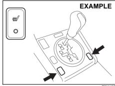
With the ignition switch in the "ON" position, push in one or both of the seat heater switches to warm the corresponding seat(s). The indicator light below the switch will also come on. To turn off the seat heater, push in the switch again. The indi-
