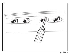
2) Release the claws of the light housing by the flat head etc. through the service holes as shown in the illustration.
