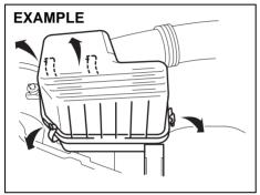
If the air cleaner is clogged with dust, there will be greater intake resistance, resulting in decreased power output and increased fuel consumption.
