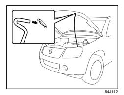
3) Continue to lift up the hood until it is high enough to support with the prop rod.
