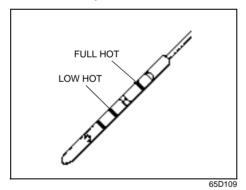
Remove the dipstick, clean it and push it back in until the cap seats. Pull out the dipstick and read the fluid level.
