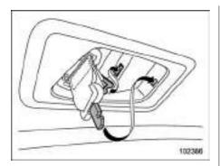
3. With the belt held by hand, allow the retractor to roll up the belt slowly. You should hold the webbing end and guide it back into the retractor while it is rolling up. Neatly store the tongue plate in the recess on the ceiling and then insert the tonque plate and connector (tongue) plate into the slot as shown in the illustration.
