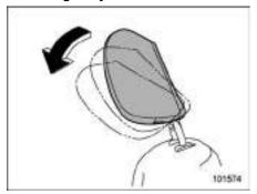
The angle of the head restraint can be adjusted in several steps. While maintaining a suitable driving posture, adjust the head restraint to a position where the back of your head is as close to the head restraint as possible.
