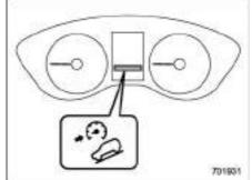
This indicator appears while the hill descent control function is in the standby mode. It flashes while the function is operating. It will disappear when the function is in the disabled mode. When this function is changed from operational to non-operational, it will disappear when the vehicle speed reaches more than approximately 18 mph (30 km/h).
