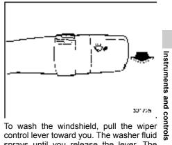
sprays until you release the lever. The wipers operate while you pull the lever.
