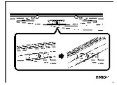
2. Turn the wiper blade assembly counterclockwise.
