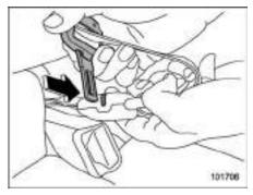
2. Insert a tongue plate or other hard pointed object into the slot in the connector (buckle) on the right-hand side and push it in. The connector (tongue) plate will then disconnect from the buckle.
