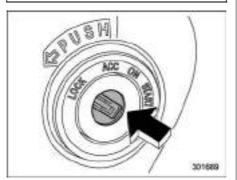
The ignition switch has four positions: LOCK, ACC, ON and START.
