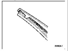
Securely retain both ends of the rubber with the stoppers on the plastic support
