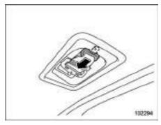
The center seatbelt is stowed in the recess of the ceiling.
