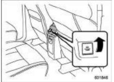
Power outlet behind the center console The maximum power rating of an appliance that can be connected is 100 W.
