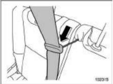
2. Slide the seat belt through the slot of the guide. The elastic cord must be placed behind the seat belt.
