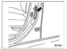
The vehicle placard is attached to the driver's side door pillar.
