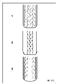
Correct tire pressure (tread worn evenly) Roadholding is good, and steering is responsive. Rolling resistance is low, so fuel consumption is also lower.
