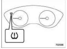
The tire pressure monitoring system provides the driver with the warning message indicated by sending a signal from a sensor that is installed in each wheel when tire pressure is severely low.
