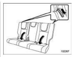
While pulling the straps, fold down the seatbacks.
