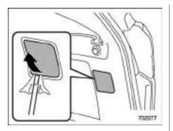
1. Remove the access cover at the rightside of the cargo area trim using a flathead screwdriver.
