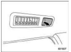
To turn on the reading light, push the lens. To turn it off, push the lens again.
