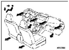
**Bi-level:** Instrument panel outlets and foot outlets
