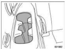
3rd-row seat's cup holder (right side) The cup holder is built into the rear side trim.
