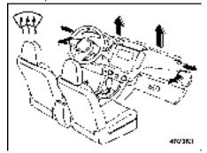
**Defrost:** Windshield defroster outlets and both side outlets of the instrument panel (Refer to "Defrosting" P276.)
