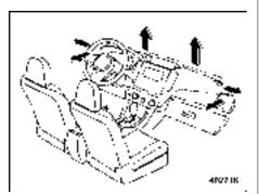
Select the "\(\frac{\psi}{\psi}\)" or "\(\psi\)" mode to defrost or dehumidify the windshield and front door windows
