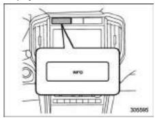
Pressing the INFO button on the instrument panel changes the display to the following sequence.
