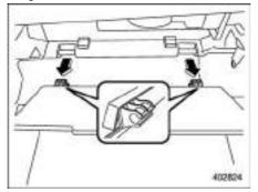
(4) Pull out the glove box horizontally and remove the hinge portion. When
