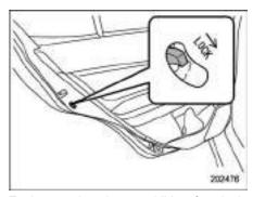
Each rear door has a child safety lock. When the child safety lock lever is in the lock position, the door cannot be opened from the inside. The door can only be opened from the outside.
