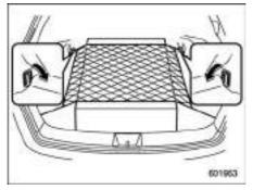
The cargo area is equipped with several tie-down hooks so that cargo can be secured with a cargo net or ropes.
