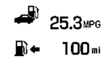
: Current fuel consumption The Driving range on remaining fuel
