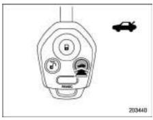
Power rear gate button on the transmitter To open the rear gate:
