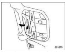
To open the console, push up the lid lightly that is located on the "PUSH" mark and it will automatically open.
