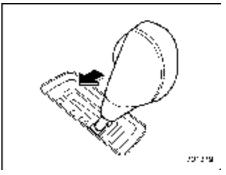
With the vehicle either moving or stationary, move the select lever from the "D" position to the "M" position to select the manual mode.
