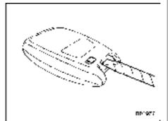
2. Wrap a flat-head screwdriver with vinyl tape or a cloth, and insert it in the gap to remove the cover.
