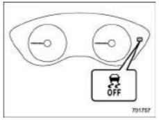
When the switch is pressed with the ignition switch in the "ON" position, the Vehicle Dynamics Control OFF indicator light "\$" on the combination meter illuminates. The Vehicle Dynamics Control system will be deactivated and the vehicle will behave like a model not equipped with the Vehicle Dynamics Control system. When the switch is pressed again to reactivate the Vehicle Dynamics Control system, the Vehicle Dynamics Control OFF indicator light turns off.
