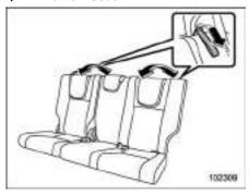
Pull the strap up and adjust the seatback to the desired position.
