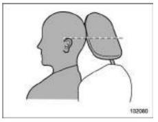
Each head restraint should be adjusted so that the center of the head restraint is closest to the top of the occupant's ears.
