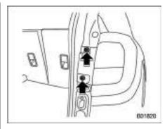
Using a Phillips screwdriver, remove the upper and lower screws that secure the rear combination light assembly.
