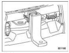
Hitch harness connector (4-pin type)
