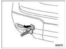
2. Cover the tip of a flat-head screwdriver with vinyl tape or cloth so that it will not scratch the bumper. Pry off the cover on the rear bumper using a screwdriver, and you will find a threaded hole for attaching the towing hook.
