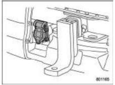
Hitch harness connector (7-pin type)
