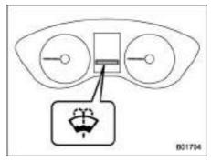
When there is only a small amount of washer fluid remaining, the windshield washer fluid warning light will illuminate. When this occurs, refill the washer fluid.
