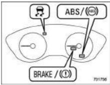
If a malfunction occurs in the EBD system, the system stops working and the following warning lights illuminate simultaneously.
