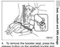
release button on the seatbelt buckle and allow the belt to retract.
