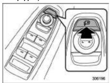
The power folding mirror switch operates only when the ignition switch is in the "ON" or "ACC" position.
