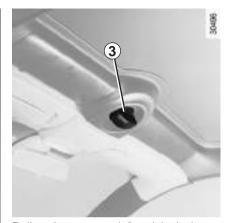
Pull and turn control **3** anticlockwise to lock the roof.
