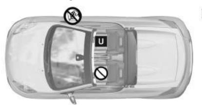
Check the status of the air bag before fitting a child seat or allowing a passenger to use the seat.
