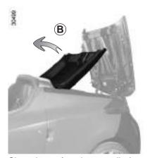
Close the roof again manually (movement **B**), making sure that there is no contact with the roof cover.
