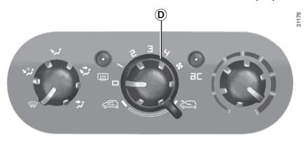
Prolonged use of this position (isolation mode) may mist up the windows slightly or cause odours due to the air not being renewed. It is therefore advisable to return to normal operation (external air) by pressing control **D** when you have passed through the polluted area.
