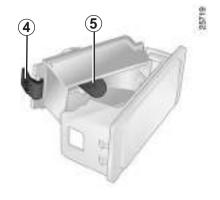
Press tab 4 to release the lens and access bulb 5.
