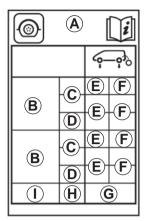
**B**: dimension of the tyres fitted to the vehicle.
