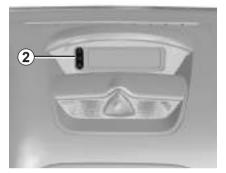
To deactivate the air bags: with the vehicle stationary, push and turn lock 1 to the OFF position.
