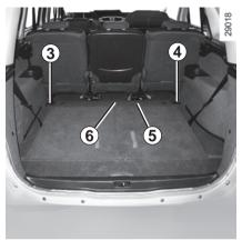
The third ring **3**, **4** and **5** (for long chassis versions) or **6** (for short chassis versions) is used to attach the upper strap on some ISOFIX seats
