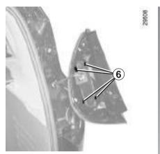
Unclip the bulb holder by pressing on the tabs **6**.
