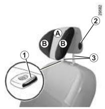
**To raise the headrest**Pull the headrest upwards to the desired height.
