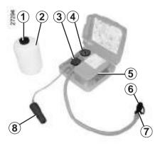
Open the kit, remove caps 1 and 3 (it is essential not to remove the cap from the bottle) then screw bottle 2 to its base 3.
