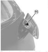
From the outside of the vehicle, pull on the light unit to remove it then unscrew bulb holder 11 a quarter of a turn.
