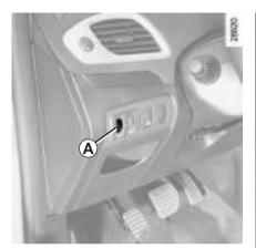
On vehicles fitted with this function, control **A** allows you to adjust the height of the beams according to the load. Turn control **A** downwards to lower the headlights and upwards to raise them. For vehicles not fitted with control **A**, adjustment is automatic.
