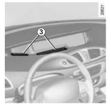
Storage compartment under the instrument panel 3
