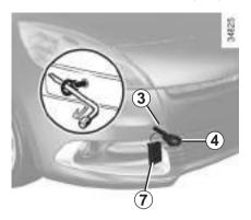
Only use the front 3 and rear towing points 5 (never use the driveshafts). These towing points may only be used for towing: never use them for lifting the vehicle directly or indirectly.
