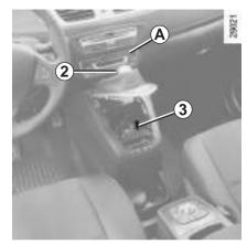
When setting off, if the lever is locked in position P even though you are depressing the brake pedal and pressing unlocking button 2, the lever can be released manually. To do this, unclip the base of the gear lever starting on the side below air conditioning controls A, press button 3 and at the same time, press unlocking button 2 on the lever.
