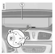
On equipped vehicles, this function, which is integrated in trip computer and warning system 1, allows you to activate/deactivate and adjust some of the vehicle's functions.
