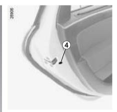
**Vehicle with manual door locking**Move lever **4** and check from the inside that the doors are securely locked, to prevent the rear doors being opened from the inside.
