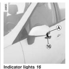
Unclip indicator light **16** using a flatblade screwdriver or similar. Position it to **A** to tilt the rear indicator light towards the front of the vehicle.
