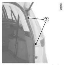
From the outside, undo screw **2** using a flat-blade screwdriver or similar and pull the light unit towards you.
