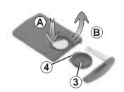
When refitting, proceed in the reverse order, then press one of the buttons on the card four times, close to the vehicle: the next time the vehicle is started, the message will disappear.
