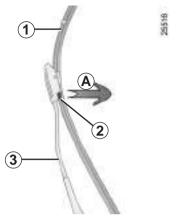
Windscreen wiper blades 1 With the ignition on and engine switched off. lower the windscreen wiper stalk completely: they stop slightly away from the bonnet.
