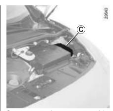
Some accessories are protected by fuses located in the engine compartment in fuse box C.
