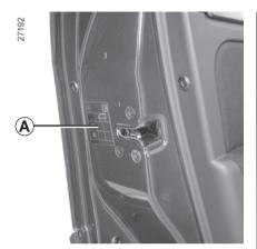
The tyre pressure is indicated on label  $\boldsymbol{A}$  affixed to the edge of the driver's door. Open the door to read it.
