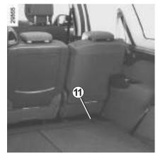
Depending on the vehicle, remove the anchoring rings 11 before installing a luggage net.
