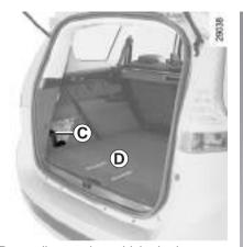
Depending on the vehicle, in the event of a puncture, use the kit located in storage compartment  $\boldsymbol{C}$  or underneath luggage compartment carpet  $\boldsymbol{D}$ .
