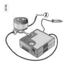
If a minimum pressure of 1.8 bar is not reached after 15 minutes, repair is not possible; do not drive the vehicle but contact an approved dealer.
