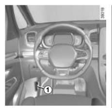
To open, pull handle 1, located on the left-hand side of the dashboard.
