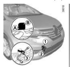
Only use the front 1 and rear 4towing points (never use the driveshafts or any other part of the vehicle). These towing points may only be used for towing: never use them for lifting the vehicle directly or indirectly.
