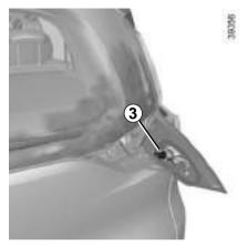
From the outside of the vehicle, pull on the light unit to remove it then unscrew bulb holder **3** a quarter of a turn.
