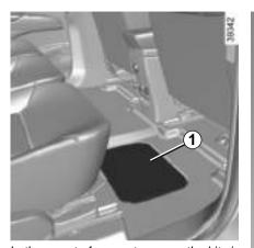
In the event of a puncture, use the kit situated under the second row rear passenger footwell flap 1.
