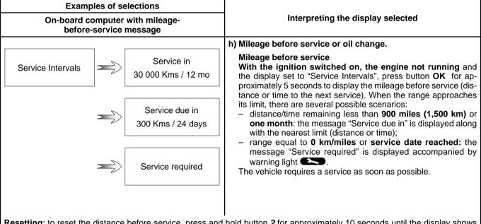
**Resetting**: to reset the distance before service, press and hold button **2** for approximately 10 seconds until the display shows the mileage permanently.
