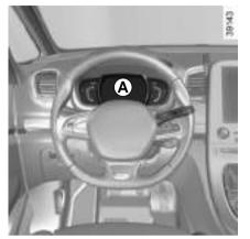
Instrument panel A: lights up when the driver's door is opened.
