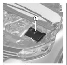
The battery **1** does not require any maintenance.
