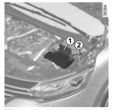
Lift the red cover on box 1 located behind the battery.
