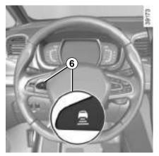
The cruising speed replaces the dashes and cruise control is confirmed by the appearance of the message "Adaptive cruise ctrl" and the warning light (5). If you try to activate the function below 30 mph (50 km/h) or above 85 mph (140 km/h), the message "Invalid speed" is displayed and the function will remain inactive.
