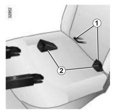
The two rings 1 are located between the seatback and the seat base and are identified by a marking. Use the access guides 2 of the child seat to ease it into place and lock it into the rings 1.
