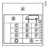
**B**: dimension of the tyres fitted to the vehicle.
