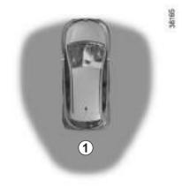
The hazard warning lights **flash twice** and a beep sounds to indicate that the doors have locked.
