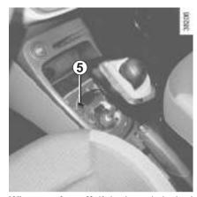
When setting off, if the lever is locked in position P even though you are pressing the brake pedal, the lever can be released manually. For this, unclip the base of the lever then insert a tool (with a hard rod to it) into the slot 5 to unlock the lever.
