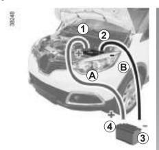
Depending on the vehicle, unclip the battery cover.
