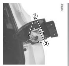
Pull on the outside  $\boldsymbol{A}$  of the light and remove the rear light unit.
