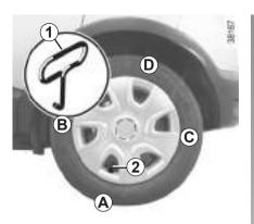
Remove the wheel trim using hubcap tool 1 (located in the tool kit) by engaging the hook in the opening near valve 2.
