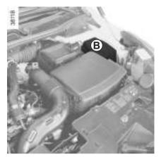
Fuses in engine compartment B
