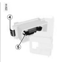
Press tab 4 to release the bulb holder and access bulb 5.
