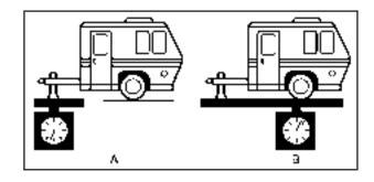
If a weight-carrying hitch or a weight-distributing hitch is being used, the trailer tongue (A) should weigh 10-15 percent of the total loaded trailer weight (B).
