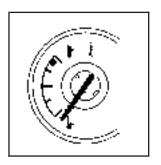
This gage measures the temperature of the vehicle's engine coolant.
