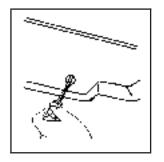
Use a tool to push the service release lever located on the latch until you hear or feel the gate release.
