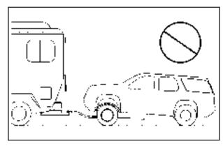
All-wheel-drive vehicles must not be towed with two wheels on the ground. To properly tow these vehicles, they should be placed on a platform truck or trailer with all four wheels off of the ground or dinghy towed from the front.
