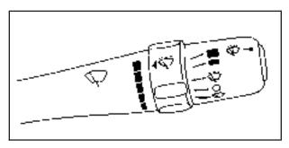
The windshield wiper lever is located on the right side of the steering column.
