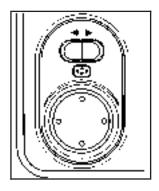
Controls for the outside power mirrors are located on the instrument panel.
