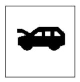
Pull the handle with this symbol on it. It is located inside the vehicle, to the left of the brake pedal.
