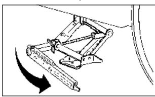
Lower the vehicle by turning the jack handle counterclockwise.
