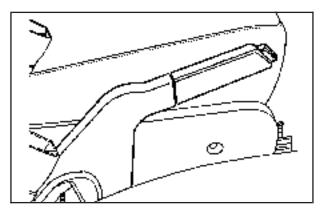
The parking brake lever is located to the right of the driver seat.
