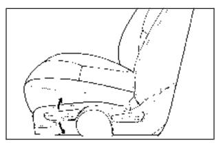
To manually raise or lower the seat, move the lever repeatedly upward or downward.
