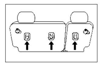
The top tether anchors for each rear seating position are located on the back of the rear seatback. You may need to adjust the rear compartment storage panel/cover in the
