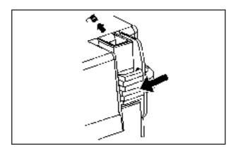
To remove the fuse block cover, release the rear of the cover first, by unlocking both of the tabs in the back. Then lift the cover off. Do not lift the front of the cover until the tabs at the rear have been unlocked. To reinstall, fit together the tabs located on the front of the cover, and push down on the cover until the tabs on the rear of the cover click into place.
