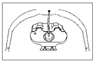
Screw the threaded wheel stow rod onto the spare tire bracket. The final position of the wheel stow rod must be turned to the farthest forward position.
