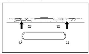
2. Turn and pull the license plate lamp down through the liftgate opening.
