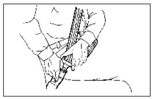
To unlatch the belt, just push the button on the buckle. For outboard seating positions, slide the latch plate up the safety belt webbing when the safety belt is not in use. The latch plate should rest on the stitching on the safety belt, near the guide loop.
