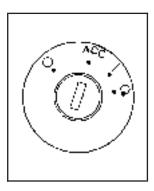
The ignition switch has four different positions.
