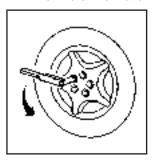
Loosen all five plastic caps by turning the wheel wrench counterclockwise.
