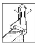
Squeeze the release buttons (A) together and move the height adjuster to the desired position.
