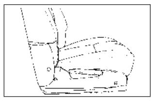
Lift up fully on the recliner lever, located on the outboard side of the seat, and fold the seatback forward until it disengages.
