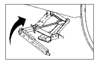
Raise the vehicle by turning the jack handle clockwise. Raise the vehicle far enough off the ground so there is enough room for the road tire to clear the ground.
