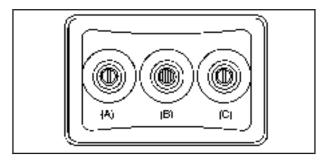
The A/V jacks are located on the rear of the floor console. The A/V jacks allow audio or video signals to be connected from an auxiliary device such as a camcorder or a video game unit to the RSE system. Adapter connectors or cables might be required to connect the auxiliary device to the A/V jacks. Refer to the manufacturer's instructions for proper usage.
