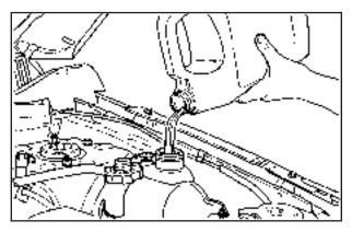
Fill the coolant surge tank with the proper DEX-COOL<sup>®</sup> coolant mixture, to the COLD FILL line.
