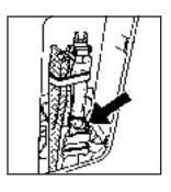
Remove the wing-bolt holding the jack and then remove it.
