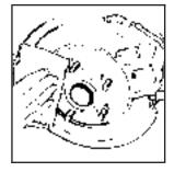
Remove any rust or dirt from the wheel bolts, mounting surfaces, and spare wheel.  Place the compact spare tire on the wheel-mounting surface.
