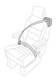
If your vehicle is fitted with individual seats, they have three-point seat belts with their guides and belt reels built into the backrests.
