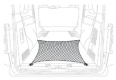
Attached to the stowing rings on the rear floor, it allows objects to be held down.
