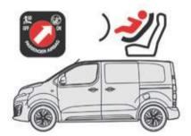
When a forward facing child seat is installed on the **front passenger seat**, adjust the vehicle's seat to the fully back and highest position with the seat backrest straightened and leave the passenger's front airbag activated.
