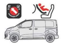
When a rearward facing child seat is installed on the **front passenger seat**, adjust the seat to the fully back and highest position, with the backrest straightened.
