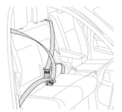
If your vehicle is fitted with a front bench seat, ensure that each belt is used with its correct buckle.
