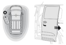
To unlock the vehicle, remote control on your person and in the recognition zone A, pull and release the door handle to trigger the electric powered opening of the corresponding door.
