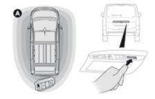
To lock the vehicle, with the remote control in the recognition zone A, press the tailgate locking control.
