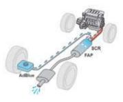
The AdBlue® is held in a special tank with a capacity of about 22 litres: this provides a driving range of about 12 500 miles (20 000 km), after which an alert is triggered warning you when the reserve remaining is enough for just 1 500 miles (2 400 km).
