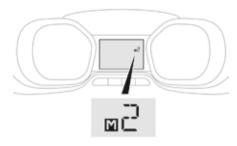
When you move the gear selector, the symbol corresponding to its position is displayed in the instrument panel.
