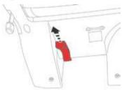
Before refitting a seat or bench seat to the vehicle, pull the strap fully to ensure that the latching mechanism has engaged.
