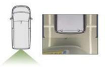
The camera records the surroundings during a manoeuvre in order to create a reconstruction of the view from above the rear of the vehicle in its close surroundings, allowing the vehicle to be manoeuvred among the obstacles nearby. This view is available with Au To view or by selecting of the view in the change view menu.
