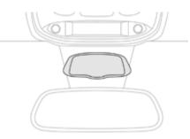
This mirror, placed on top of the central mirror, enables the driver or front passenger to observe all the rear seats.
