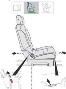
Two controls are provided for moving the seat forwards and backwards:
