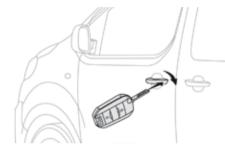
To unlock the vehicle totally, turn the key to the rear of the vehicle.
