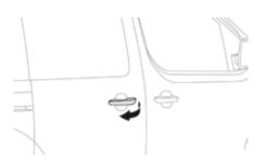
After unlocking the vehicle (using the key, remote control or Keyless entry and Starting, depending on equipment) pull the door handle.
