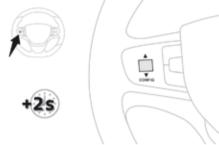
o r, depending on equipment, press the thumbwheel on the steering wheel for more than two seconds.
