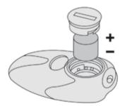
use a coin to unscrew the cap and replace the bulb.
