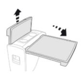
Pull each table top fully up then pivot them on each side into the horizontal position.
