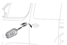
Insert the key in the door lock and turn it to the rear.
