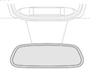
This system automatically and progressively changes between the day and night uses by means of a sensor, which measures the light from the rear of the vehicle.
