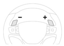
You can temporarily take control of gear changes using the "+" and "-" steering mounted control paddles. The gear change instruction is acted on if the engine speed permits.
