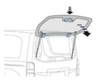
Close the rear screen by pressing the centre of the glass until it is fully closed.
