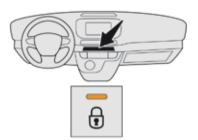
This button is inoperative if the vehicle has been locked or deadlocked from outside (using the key, remote control or Keyless entry and Starting, according to equipment) or if one of the doors is still open.
