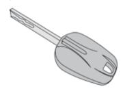
The key allows the central locking or unlocking of the vehicle using the door lock.
