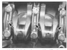
11.17 Main bearing cap identification markings (arrowed)
