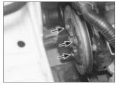
5.6a Undo the three retaining bolts (arrowed) . . .
