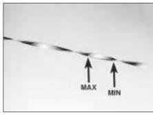
Note the oil level on the end of the dipstick, which should be between the upper ("MAX") mark and lower ("MIN") mark. Approximately 1.0 litre of oil will raise the level from the lower mark to the upper
