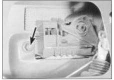
14.7a Exterior door handle securing nut (arrowed) - early model
