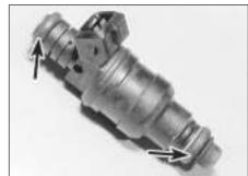
14.30 Injector O-ring seals (arrowed)
