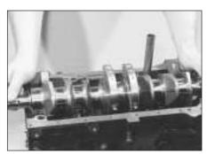
11.20 Lifting out the crankshaft - XU series engine
