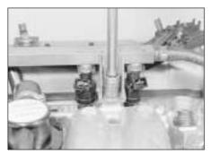
14.28a Removing a fuel rail bolt . . .
