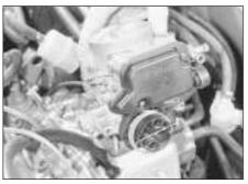
12.10b ... and lift off the carburettor
