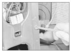
22.18b Unscrew the aerial motor securing bolt . . .
