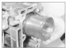
12.18a On aluminium block engines, remove each liner . . .
