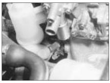
12.7 Disconnecting the float chamber breather solenoid wiring
