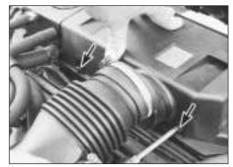
21.14a ... then slacken the retaining screws (arrowed) . . .
