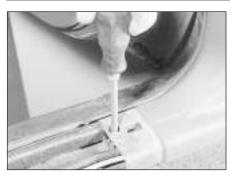
27.6 Removing a lower B-pillar trim panel bottom securing screw
