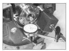
14.2 Checking crankshaft endfloat using a dial gauge
