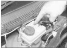
Check the operation of the low fluid level warning light. Chock the roadwheels, release the handbrake, and switch on the ignition. Ask an assistant to press the button on top of the reservoir. The brake fluid level/ handbrake warning light should come on. Apply the handbrake and switch off the ignition
