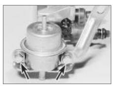
14.37 Regulator-to-fuel rail bolts (arrowed)
