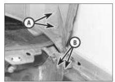
8.3 Hinge-to-bonnet bolts (A) and hinge-to-body bolts (B)
