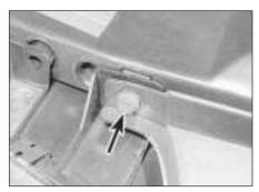
25.3 ... and the upper securing bolts (arrowed)
