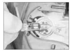
5.23b Removing a headlight-mounted driving light bulb
