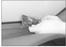
21.9b ... and disconnect the wiring plug - models from 1993
