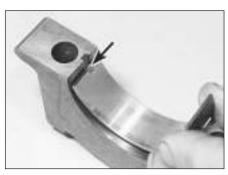
18.34 On XU engines, all the lower shells have a plain bearing surface. Ensure tab (arrowed) is correctly located in the cap
