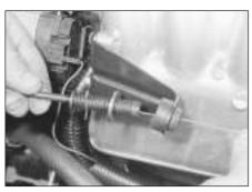
3.1b Disconnecting the accelerator cable end fitting (Bosch L3.1 system)
