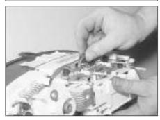
6.27 Removing an instrument panel illumination bulb
