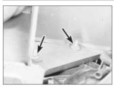
6.3 Front bumper front securing nuts (arrowed)
