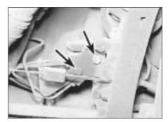
21.4 Rear brake pressure-regulating valve securing bolts (arrowed)
