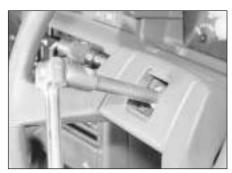
16.4 Unscrewing the steering wheel nut
