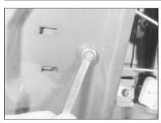
20.8 Unscrewing the tailgate lock motor securing bolt
