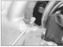
18.3 Disconnecting the brake servo vacuum hose
