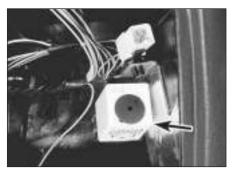
13.2 "Lights on" warning buzzer (arrowed)
