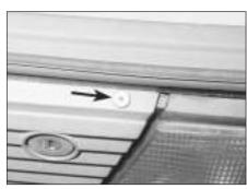
17.3 Drill out the rivets (arrowed) from the body rear trim panel
