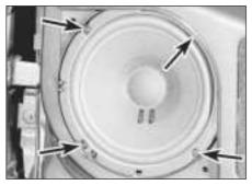
21.3 Door-mounted loudspeaker securing screws (arrowed)
