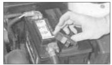
Check that the ignition coil wiring plug is secure, and spray with water-dispersant if necessary.
