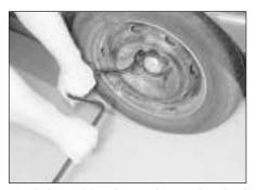
Before raising the car, loosen the wheel bolts slightly using the wheelbrace.
