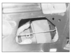
14.7c . . . and withdraw the plastic shield -
