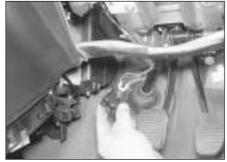
30.62b . . . then pull the connector from the steering column bracket
