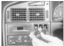
30.39b . . . then remove the remaining housing securing screw
