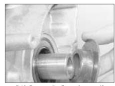
7.12 Remove the flanged spacer if necessary
