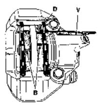
4.12b Correct fitting of brake pads - Bendix caliper
