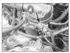
16.14 Throttle potentiometer wiring connector (arrowed)
