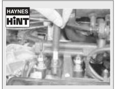
It is often difficult to insert spark plugs into their holes without cross-threading them. To avoid this possibility, fit a short length of 5/16 inch internal diameter rubber hose over the end of the spark plug. The flexible hose acts as a universal joint to help align the plug with the plug hole. Should the plug begin to cross-thread, the hose will slip on the spark plug, preventing thread damage to the cylinder head.
