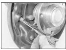
19.19 Tapping the handbrake cable sheath end fitting from the brake backplate
