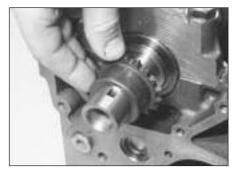
11.16b . . . then slide off the drive sprocket . . .
