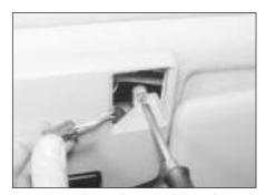
20.31 Removing a roof console securing screw
