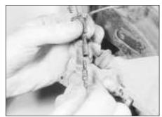
4.2 Disconnecting the pad wear sensor wiring connector
