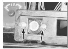
8.10 Headlight adjuster switch securing screws (arrowed)
