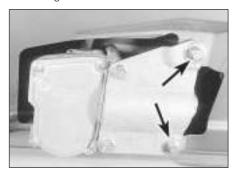
18.7 Tailgate wiper motor securing bolts (arrowed)
