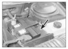
The battery is located on the left-hand side of the engine compartment. The exterior of the battery should be inspected periodically for damage such as a cracked case or cover.
