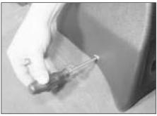
29.26 Unscrew the console rear screws ("Lowline" console - models from 1993)
