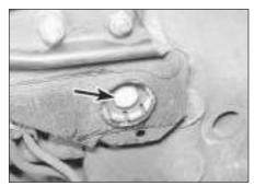
9.9 Subframe rear mounting bolt (arrowed)
