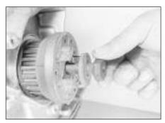
7.11a Remove the crankshaft sprocket retaining bolt . . .
