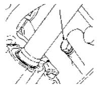
20.5b Cylinder block drain plug location (arrowed) - 2.0 litre engine
