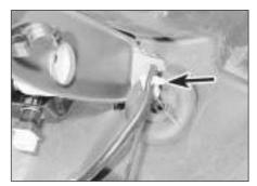
7.4 Accelerator cable connection to accelerator pedal (arrowed)
