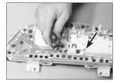
10.6 Remove the two recessed lens securing screws
