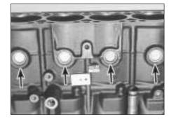
12.1 Cylinder block core plugs (arrowed)
