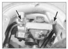
3.5c Coil mounting bolts (arrowed) on Bosch L3.1 system
