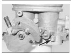
14.6a Secondary throttle adjusting screw (arrowed) . . .
