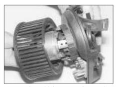
9.66 ... then withdraw motor from casing
