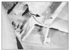
6.4 Front bumper side securing bolt (arrowed)
