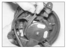
9.64 Pull the rubber grommet from the motor casing for access to the wiring
