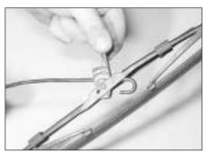
Pull the arm fully away from the glass until it locks. Swivel the blade through 90°, then pull up the blade securing clip, and slide the blade out of the arm's hooked
