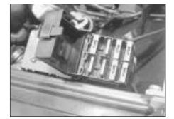
3.4 Fusebox location on right-hand side of engine compartment
