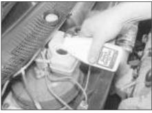
Carefully add fluid, avoiding spilling it on surrounding paintwork. Use only the specified hydraulic fluid; mixing different types of fluid can cause damage to the system and/or a loss of braking effectiveness. After filling to the correct level, refit the cap securely. Wipe off any spilt fluid.
