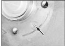
9.2 Rear brake drum retaining screw (arrowed)
