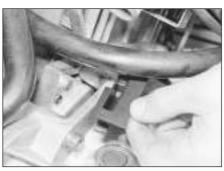
6.2a Removing the plastic cover from the timing aperture
