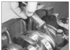
14.3 Checking crankshaft endfloat using feeler gauges
