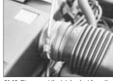
21.13 Disconnect the intake duct from the front of the cylinder head cover . . .
