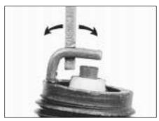
Adjusting spark plug gap
