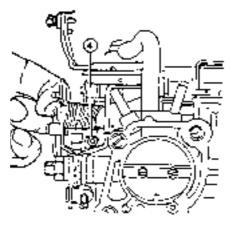
13.36 Choke mechanical opening adjustment nut (4) (Weber carburettor)
