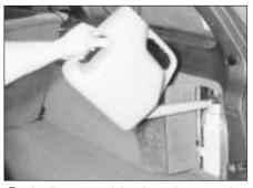
On Estate models, the tailgate washer fluid reservoir is located behind a hinged cover on the right-hand side of the luggage compartment.
