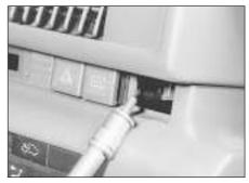
9.3a . . . and remove the visor securing screws
