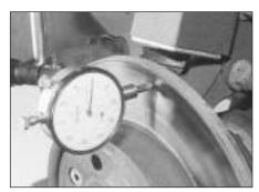
7.4 Checking disc run-out using a dial gauge
