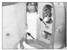
19.8a Remove the two securing screws (arrowed) . . .
