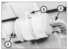
14.55 Fuel filter showing fuel hoses (A) and clamp bolt (B)
