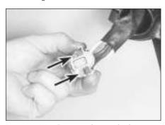
18.8a Remove the two lock securing screws . . .
