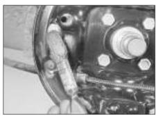
6.17 Apply high-melting-point grease to the shoe contact points on the backplate
