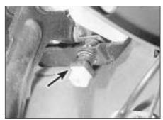
22.1 Stop-light switch (arrowed) on brake pedal bracket
