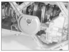
13.11b . . . then refit the plate to the base of the cylinder block/crankcase
