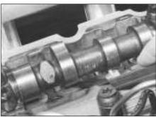
11.9 Measuring a valve clearance using a feeler blade
