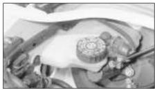
☐ The fluid reservoir must be secure and the fluid level must be between the upper (A) and lower (B) markings.
