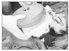
15.15 Removing the vacuum servo/pedal bracket assembly
