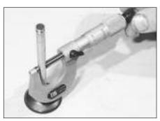
8.11 Measuring a valve stem diameter
