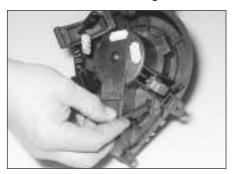
9.67 Disconnect the wiring plug . . .
