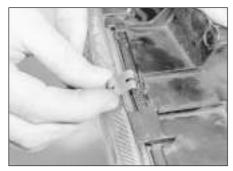
7.9 Removing a headlight lens securing clip
