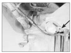
4.5a Extract the spring clip (arrowed) . . .
