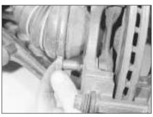
7.7 Removing a Girling caliper mounting bracket bolt
