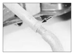
23.3 Track rod end locknut (arrowed)
