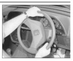
movement of the steering wheel, indicating wear in the column support bearings or couplings.
