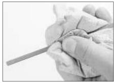
Using a clean rag or paper towel remove all oil from the dipstick. Insert the clean dipstick into the tube as far as it will go, then withdraw it again.
