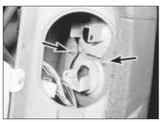
7.34a Rear wing-mounted light cluster securing nuts (arrowed) - Estate model
