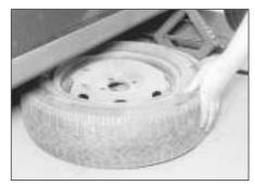
Temporarily place the spare wheel under the sill as a precaution should the jack topple.
