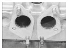
15.7 New gaskets fitted to the exhaust ports on the cylinder head (XU engine)
