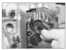
7.4c Remove the spring retainer . . .
