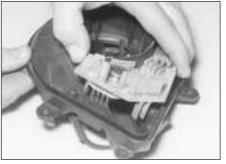
9.68b ... and withdraw the control module
