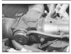
3.17 Air temperature control valve assembly (TU engine)
