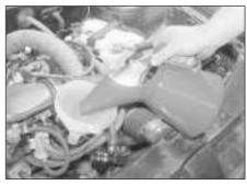
Oil is added through the filler cap. Unscrew the cap and top-up the level; a funnel may help to reduce spillage. Add the oil slowly, checking the level on the dipstick often. Don't overfill (see "Car Care" left).
