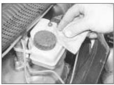
2 If topping-up is necessary, first wipe the area around the filler cap with a clean rag before removing the cap. Check the fluid already in the reservoir - the system should be drained and refilled if dirt is seen in the fluid (see Chapter 9 for details).
