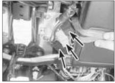
17.8 Ignition switch wiring connectors (arrowed) - models from 1993
