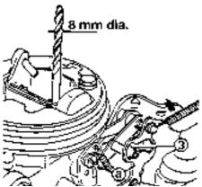
13.34 Checking the choke mechanical opening (Weber carburettor)
