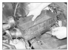
2.4 Removing the air cleaner housing
