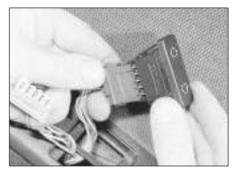
13.7 Removing an electric window switch from the door
