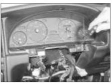
9.21 Unscrew the lower instrument panel securing screws
