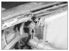
20.4c Radiator bleed screw (arrowed)
