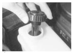
If topping-up is necessary, and before removing the cap, wipe the area so that dirt does not enter the reservoir. Unscrew the cap, allowing the fluid to drain from the bottom of the cap as it is removed.
