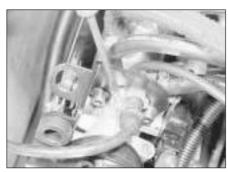
12.4 Disconnecting the coolant inlet hose
