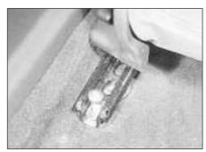
26.3 Front seat rear securing bolt partially removed
