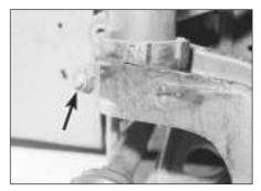
2.12 Hub carrier-to-suspension strut clamp nut (arrowed)
