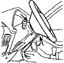
25.7 Turn the steering wheel for access to the two air bag unit screws (arrowed)
