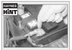
Battery corrosion can be kept to a minimum by applying a layer of petroleum jelly to the clamps and terminals after they are reconnected.
