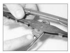
On Estate models, to remove a tailgate wiper blade, pull the arm fully away from the glass until it locks. Swivel the blade through 90°, then press the locking tab, and slide the blade out of the arm's hooked end.
