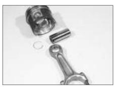
13.15c Piston and connecting rod components
