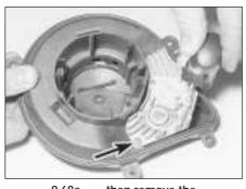
9.68a ... then remove the securing screws . . .
