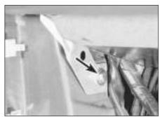
30.21 Lower facia mounting bracket-tofootwell bolt (arrowed)
