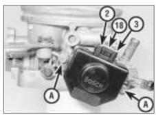
14.13 Throttle switch unit mounting bolts (A) and plug terminal numbers
