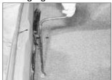
In the boot, use the wheel brace to loosen the spare wheel cradle bolt.
