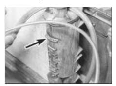
The coolant level varies with engine temperature. When cold, the coolant level should be on the "MAXI" mark (arrowed). When the engine is hot, the level may rise slightly above the "MAXI" mark.
