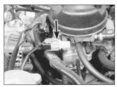
16.3 Injector wiring connector (arrowed)
