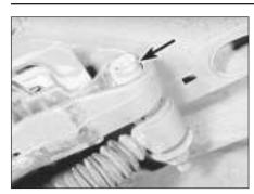
13.3 Rear shock absorber upper mounting bolt (arrowed)
