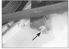
5.15 Auxiliary drivebelt tension adjustment bolt (arrowed)
