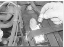
Note that the battery negative terminal stud can be removed for cleaning or renewal. Unscrew the lead clamp, then pull off the plastic insulator, and lever off the stud and cover.
