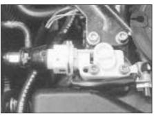
17.32 Throttle housing heating element
