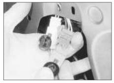
22.3 Disconnecting the door mirror wiring connectors
