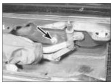
30.70 Facia securing nut (arrowed) in scuttle
