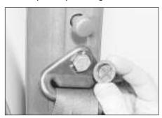
27.3 Removing the trim plate from the front seat belt upper anchor bolt
