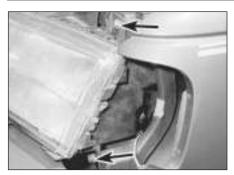
7.8 Outer headlight securing bolts (arrowed)
