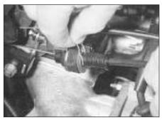
7.9 Adjusting the accelerator cable
