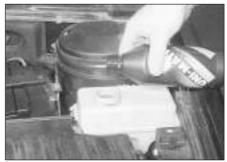
Top-up to the "MAX" mark, using the specified type of fluid. Take great care not to allow dirt to enter the reservoir, and do not overfill the reservoir. When the level is correct, refit the cap.
