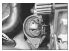
7.6a Withdraw the coolant pump . . .
