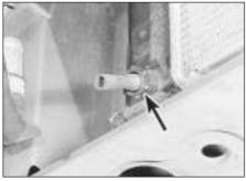
20.3 Radiator drain outlet (arrowed)
