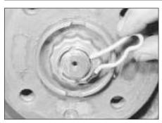
2.3 Withdraw the R-clip from the driveshaft nut locking cap
