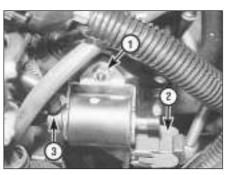
19.19 ACAV solenoid valve retaining nut (1), wiring connector (2) and hose connections (3)
