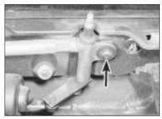
17.8b Windscreen wiper linkage securing nut (arrowed)
