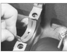
11.21 Remove the upper main bearing shells from the cylinder block/crankcase, and store them with their lower shells
