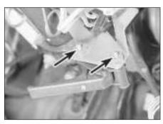
9.3 Bonnet release lever securing bolts (arrowed) lever mounted on right-hand side
