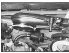
... and remove the duct, positioning it clear of the air cleaner housing
