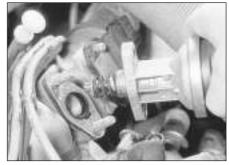
4.5 Removing the fuel pump (XU engine)
