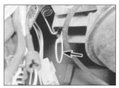
5.13 Front direction indicator light retaining spring (arrowed)
