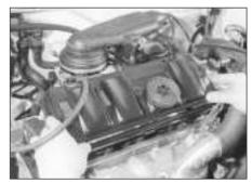
4.5 ... and lift off the cylinder head cover
