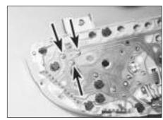
10.9 Fuel gauge securing nuts (arrowed)
