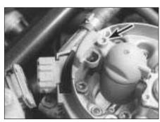
15.16 Disconnecting the injector wiring connector. Injector screw is arrowed
