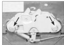
10.2 Bonnet lock securing bolts (arrowed)
