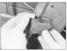
20.9 Disconnecting the wiring plug from the tailgate lock motor
