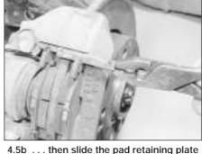
4.5b . . . then slide the pad retaining plate from the caliper - Bendix caliper
