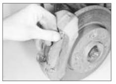
4.6 Withdrawing the outer brake pad - Bendix caliper
