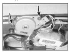
24.11 Sunroof motor securing screws (arrowed)
