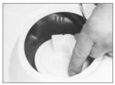
10.1 Removing the fuel gauge sender unit
