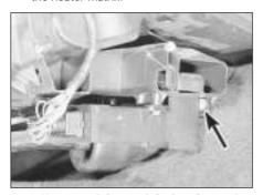
9.47 Heater unit lower right-hand securing bolt (arrowed)
