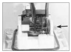
14.4 Pedal pivot bolt and nut (arrowed)
