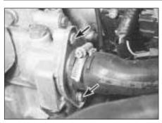
4.4a Thermostat housing cover retaining bolts (arrowed) - 1.4 litre engine
