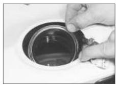
9.12b ... and recover the rubber sealing ring
