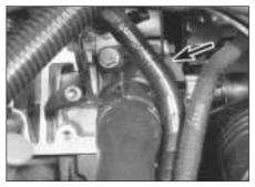
4.4b Thermostat housing cover (arrowed) - 2.0 litre engine
