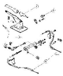
19.4 Handbrake lever and cable components
