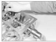
10.9b ... and slide out the camshaft
