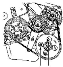
22.25 Unscrew the two front pump mounting bolts (arrowed) - XU7 and XU10 engines without air conditioning
