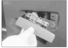
14.8 Withdrawing the exterior door handle
