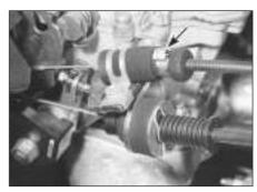
9.10 Choke cable-to-rubber collar retaining clip (arrowed)
