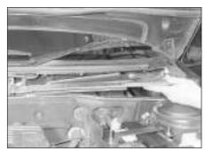
30.64b . . . and withdraw the shield from the scuttle
