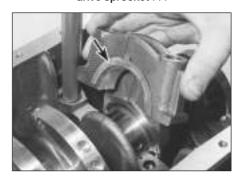
11.19 Removing No 2 main bearing cap.
