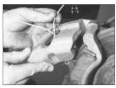
4.23 ... then refit the caliper, feeding the pad wiring through the caliper aperture
