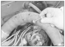
The dipstick top is often brightly coloured for easy identification (see "Underbonnet check points" on pages 0.10 and 0.11 for exact location). Withdraw the dipstick.
