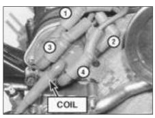
4.17 Distributor cap and HT leads on the XU9J4 16-valve model
