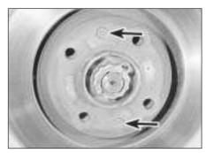
7.8 Disc securing screws (arrowed)
