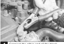
Connect the other end of the black jump lead to a bolt or bracket on the engine block, well away from the battery, on the vehicle to be started.
