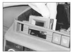
11.5 Removing the clock - models up to 1992
