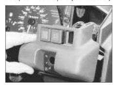
9.6 Withdrawing the driver's side upper facia panel
