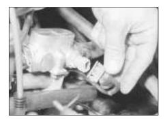
14.48 Disconnecting the injection thermistor wiring
