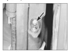
4.29 Rubber gaiter pulled back to expose courtesy light securing screw (arrowed)
