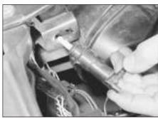
7.4 Removing a cable-operated headlight adjuster
