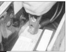
Connect the other end of the red lead to 2 the positive (+) terminal of the booster battery.
