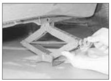
Locate the jack head in the jacking point and use the brace to raise the car until the wheel is clear of the ground.
