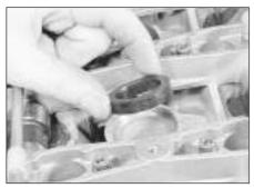
4.32 Fitting a spark plug hole oil seal
