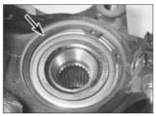
3.3 Front hub bearing retaining circlip (arrowed)
