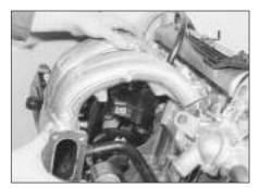
18.12c Fitting the inlet manifold
