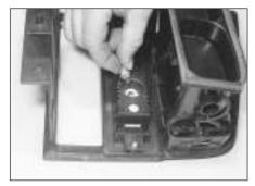
6.23 Removing the clock illumination bulb - models from 1993
