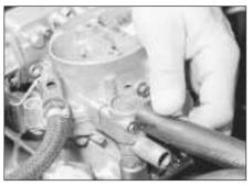
12.5 Disconnecting the float chamber breather pipe
