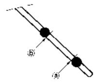
4.2b Automatic transmission fluid dipstick lower (a) and upper (b) fluid level markings
