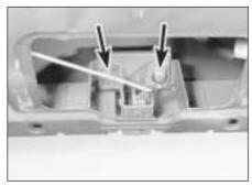
19.9 Tailgate lock securing bolts (arrowed)
