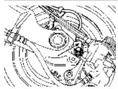
24.15 Rear wheel ABS sensor (arrowed)
