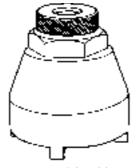
7.3 Peugeot special tool for removing front suspension lower balljoint
