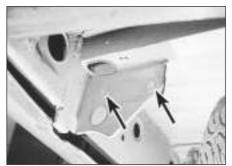
7.13 Rear bumper side securing bolts (arrowed) - Estate model
