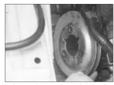
5.6b ... and remove the crankshaft pulley
