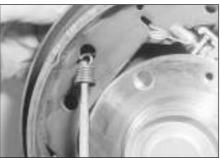
6.6b Removing an early type Bendix shoe retainer spring
