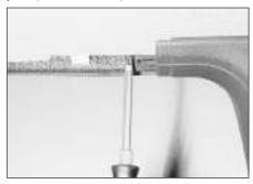
27.2 Removing an upper B-pillar trim panel top securing screw
