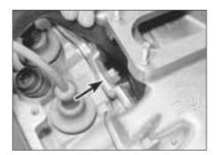
14.6 Inlet manifold centre clamp on the XU engine
