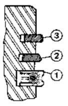
17.10 Piston ring fitting diagram (typical)
