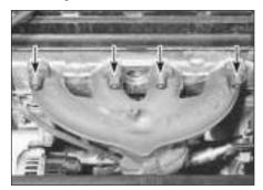
15.6 The exhaust manifold retaining nuts (TU engine)
