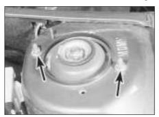
4.2 Suspension strut top mounting nuts (arrowed)
