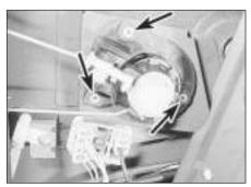
19.4 Tailgate lock cylinder securing rivets (arrowed)
