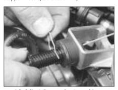
4.3 Adjust the accelerator cable as described in text
