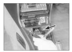
29.32a Remove the front securing screws . . .
