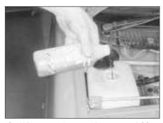
When topping-up the reservoir(s) a screenwash additive should be added in the quantities recommended on the bottle.
