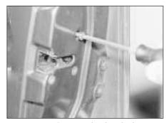
14.16 Remove the door lock securing screws
