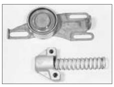
8.31 Timing belt tensioner assembly components - early 1580 cc and 1905 cc 8-valve models
