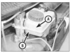
The "MAX" (A) and "DANGER" (B) marks are indicated on the side of the reservoir, which is located in the scuttle at the rear driver's side of the engine compartment. The fluid level must be kept between these two marks.
