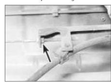
17.7 Handbrake cable adjuster (arrowed)
