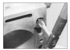
12.9 Cleaning a cylinder block threaded hole using a suitable tap
