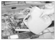
Add a mixture of water and antifreeze through the expansion tank filler neck, until the coolant level is up to the "MAXI" level mark. Refit the cap, turning it clockwise as far as it will go to secure.
