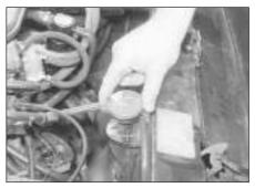
If topping up is necessary, wait until the engine is cold. Unscrew the expansion tank cap to the first stop, to release any pressure present in the system. Push the cap down, turn to the second stop, and remove it.
