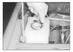
The windscreen/headlight washer fluid reservoir is located in the scuttle at the rear right-hand corner of the engine compartment.
