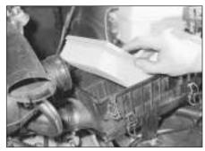
21.9 Removing the air filter element
