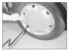
Use the wheel brace to remove the wheel
