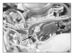
10.7 Idle mixture adjustment screw (arrowed)
