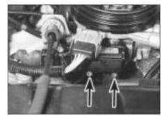
15.11 Idle control stepper motor retaining screws (arrowed)
