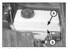
The fluid level is visible through the translucent material of the reservoir, and should be between the maximum (A) and minimum (B) level lines marked on the side of the reservoir.
