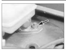
13.5 Master cylinder securing nut (arrowed)
