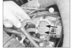
4.3 Arrows on raised fuel pump unions indicate the direction of fuel flow
