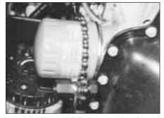
3.8 Using an oil filter removal tool to slacken the oil filter
