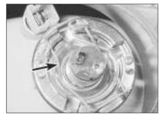
5.4a Release the spring clip (arrowed) . . .
