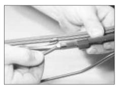
Check the condition of the wiper blades; if they are cracked or show any signs of deterioration, or if the glass swept area is smeared, renew them. For maximum clarity of vision, wiper blades should be renewed annually, as a matter of course. To remove a front wiper blade, first prise off the securing clips, and disconnect the washer tube from the arm.
