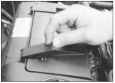
21.14b . . . and release the retaining clips
