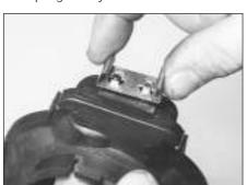
3.14a Remove the retaining clip . . .
