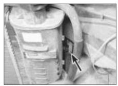
8.2b Headlight beam horizontal fine adjuster (arrowed)
