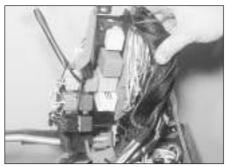
3.14c Main relay box located behind fusebox at rear of facia - models from 1993 (viewed with facia removed and inverted)
