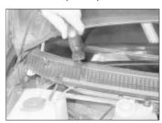
25.9 Unscrew the grille panel securing screws
