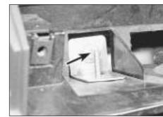
30.23 Upper facia securing bolt (arrowed)
