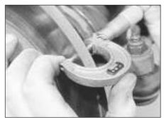
7.3 Using a micrometer to measure disc thickness
