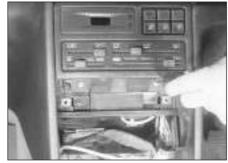
30.38a Remove the two screws from the front of the ventilation nozzle housing . . .
