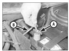
Check the tightness of the battery cable clamps (A) to ensure good electrical connections. You should not be able to move them. Also check each cable (B) for cracks and frayed conductors.
