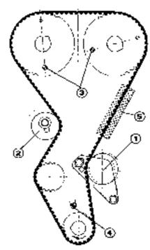
7.27 Timing belt arrangement -1998 cc 16-valve models
