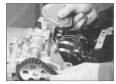
14.3 Removing the oil pump
