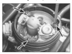
15.15a Undo the three retaining screws (arrowed) . . .
