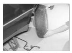
Remove the bolts and remove the wheel. Fit the spare wheel and hand-tighten the bolts. Lower the car, then tighten the wheel bolts firmly. Have the bolts tightened to the correct torque at the earliest opportunity.
