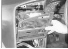
30.40 Withdrawing the ventilation nozzle housing
