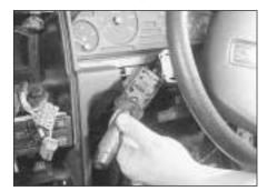
4.6b . . . and withdraw the steering column combination switch - models from 1993
