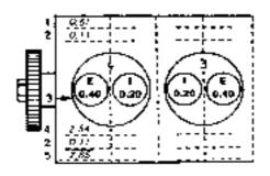
11.7 Example of valve shim thickness calculation
