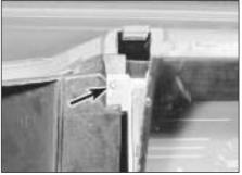
9.8 Instrument panel securing screw (arrowed)
