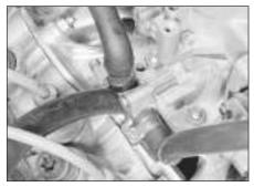
12.6b ... and base heating pipes
