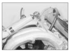
18.12d Tightening the manifold securing bolts
