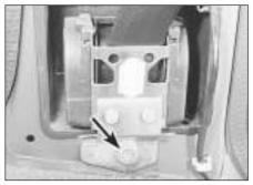
27.7 Front inertia reel securing bolt (arrowed)
