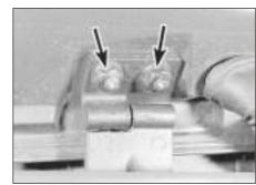
18.12 Hinge-to-tailgate nuts (arrowed)
