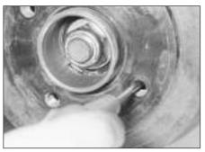
9.3b Releasing the handbrake operating lever
