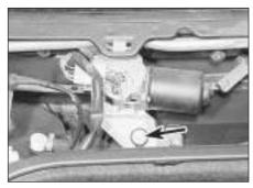
17.8a Windscreen wiper motor securing nut (arrowed)
