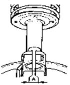
2.19b Gap (A) on later type hub carrier clamp lugs must not be less than 6.5 mm
