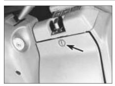
3.3a Release the securing clips (arrowed) . . .
