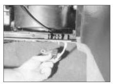
9.59 Disconnect the blower motor wiring plug
