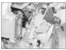
12.8 Removing the throttle housing
