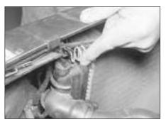
3.10 Releasing a radiator upper securing clip
