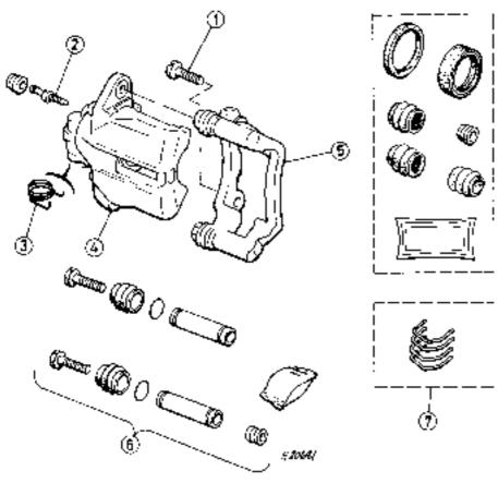
11.6 Components of rear caliper
