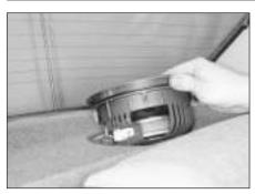
21.13 Removing the rear loudspeaker - Saloon models
