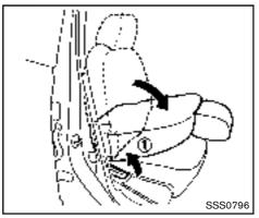
Folding front passenger's seat (if so equipped)
