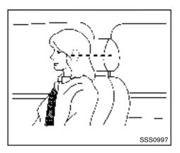
Adjustment Adjust the head restraint so the center is level with the center of your ears.
