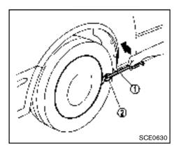
Removing wheel cover (if so equipped)
