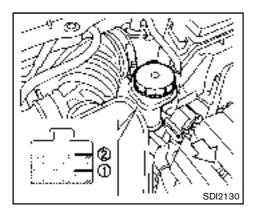
Check the fluid level in the reservoir. If the fluid is below the MIN line ① or the brake warning light comes on, add Genuine NISSAN Super Heavy Duty Brake Fluid or equivalent **DOT 3** fluid up to the MAX line ②. If fluid must be added frequently, the system should be checked by a NISSAN dealer.
