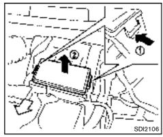
Push the tabs ① and pull out the filter element ②.
