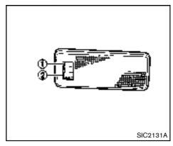
When the switch is in the ON position (1), the light illuminates while the lift gate is opened. When the lift gate is closed, the light will turn off.
