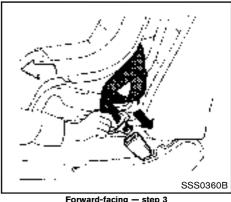
Route the seat belt tongue through the child restraint and insert it into the buckle until you hear and feel the latch engage. Be sure to follow the child restraint manufacturer's instructions for belt routing.
