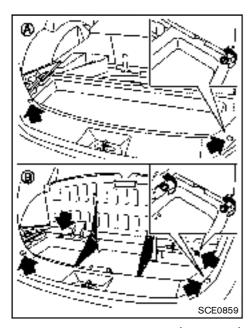
5. Remove the luggage floor box (Type A or B) by turning the clips counterclockwise.
