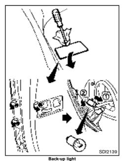
Open the lift gate to remove the back-up light assembly. One screw is located behind the cover on the lift gate.
