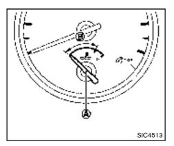
normal range, reduce vehicle speed to decrease temperature. If the gauge is over the normal range, stop the vehicle as soon as safely possible. If the engine is overheated, continued operation of the vehicle may seriously damage the engine. See "If your vehicle overheats" in the "6. In case of emergency" section for immediate action required.
