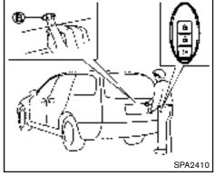
When you carry the Intelligent Key with you, you can lock or unlock all doors by pushing the door handle request switch (driver's or front passenger's) (a) or lift gate request switch (b) within the range of operation.
