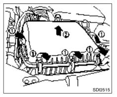
To remove the filter, release the lock pins (1) and pull the unit upward (2).
