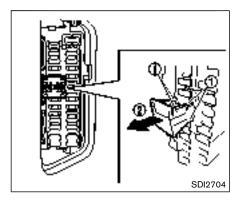
Extended storage fuse switch (if so equipped)
