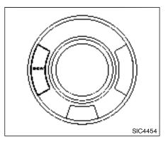
For driving or starting the vehicle on snowy roads or slippery areas, turn the SNOW mode on.
