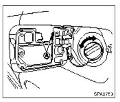
To remove the fuel-filler cap:
