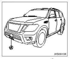
The FEB system uses a sensor (a) located below the front bumper to measure the distance to the vehicle ahead in the traveling lane.
