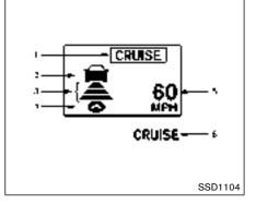
Vehicle-to-vehicle distance control mode display and indicators
