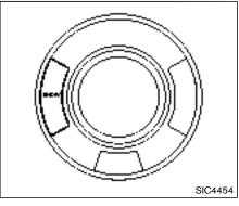
For driving or starting the vehicle on snowy roads or slippery areas, push on the SNOW mode switch. The SNOW mode indicator light will illuminate. When the SNOW mode is activated, engine output is controlled to avoid wheel spin.
