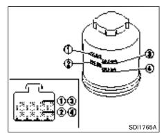
Check the fluid level in the reservoir.
