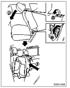
and fold the seatback forward onto the seat base. Then lift up on the seat base and tip it forward.
