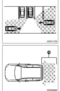
The radar sensors (A) detect an approaching vehicle from up to approximately 49 ft (15 m) away. The sonar sensors (B) detect stationary objects behind the vehicle up to approximately 4.9 ft (1.5 m). Refer to the illustration for approximate zone coverage areas (C).
