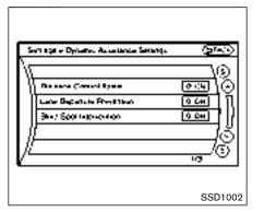
Highlight the "Distance Control Assist" key, select ON (enabled) or OFF (disabled) and push the ENTER button (2).
