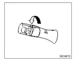
FOG LIGHT SWITCH (if so equipped) To turn the fog lights on, turn the headlight switch to the g position, then turn the switch to the  $\pm$  position. To turn them off, turn the
