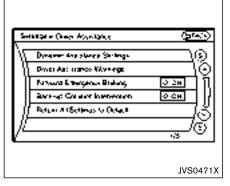
Highlight the "Forward Emergency Braking" key, select ON (enabled) or OFF (disabled) and push the ENTER button (B).
