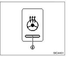
The heated steering wheel system is designed to operate only when the surface temperature of the steering wheel is below  $68^{\circ}F$  ( $20^{\circ}C$ ).
