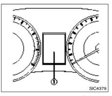
The vehicle information display (1) located between the speedometer and odometer, and shows the indicators for the driving systems, Intelligent Key operation and various warnings and information.
