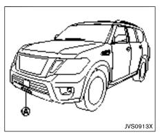
The PFCW system uses a radar sensor (A) located below the front bumper to measure the distance to a second vehicle ahead in the same lane.
