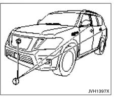
To display the multiple views, the Around View<sup>®</sup> Monitor system uses cameras (1) located in the front grill, on the vehicle's outside mirrors and one just above the vehicle's license plate.
