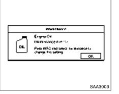
The Reminder will be automatically displayed when the specified distance has been driven and every time the ignition switch is pushed to the ACC or ON position. The reminder will not appear while driving.
