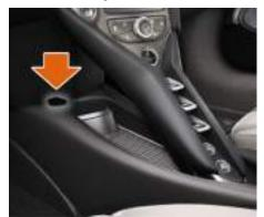
The interior accessory 12 V socket is located adjacent to the front cup holder in the center console and has a maximum load rating of 15 Amps.
