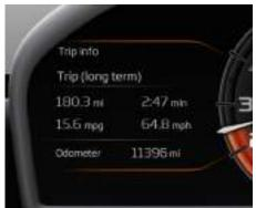
Displays distance, time, average fuel consumption and average speed since the last trip reset.
