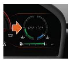
The oil temperature is displayed in the form of a colored gauge on the right-hand side of the Driver Display.
