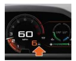
The gearbox mode indicator displays M and the currently selected gear. All forward gear changes are made by operating the gearshift paddles, see Gearshift paddles, page 2.20.
