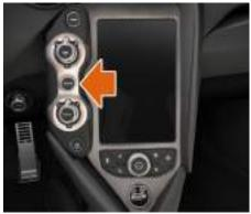
3. Press the **ACTIVE** button to switch on the Active Dynamics Panel.
