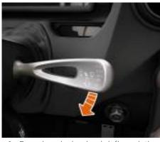
For a slow single wipe, briefly push the wiper stalk down and release. The wipers will operate once at slow speed, without washers.
