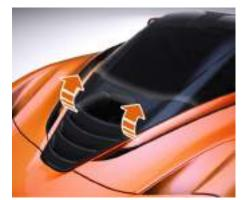
From the side of the vehicle, grasp the two rear edges of the service cover and rotate the service cover upwards towards the rear windscreen to remove.
