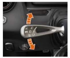
Push the turn signal/hi beam stalk downwards (1) to switch on the left-hand turn signal.
