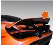
The active central high mounted stop lamp, located in the Airbrake, will illuminate under braking if the Airbrake is deployed as the Airbrake will obscure the static central high mounted stop lamp.
