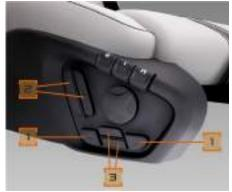
Press the switches (3) until the seat reaches the desired height.
