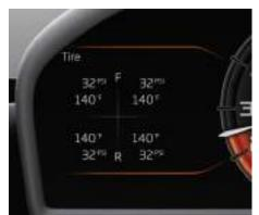
This shows the pressures and temperatures of each of the 4 tires. If the figures appear in white, no action is required. If they appear as amber or red text, have the tires inspected and pressures rectified as soon as possible.
