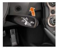
Before nose lift can be activated, the engine must be running. To raise the nose of the vehicle, activate the nose lift menu (see Nose lift operation, page 1.44) and then move the control stalk upwards.
