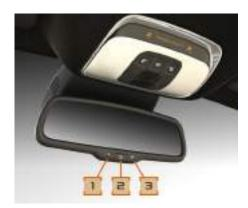
The automatic dimming function of the interior mirror is activated or deactivated by pressing the switch (2) on the bottom of the mirror. The indicator light (1) will illuminate when automatic dimming is active.
