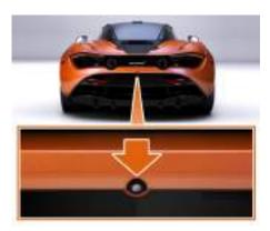
The rear view camera (RVC) is mounted in the center of the rear bumper. The live video feed is displayed on the Driver Display when the function is active.
