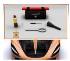
The tire sealant (3) is located at the front of the luggage compartment.
