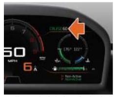
Accelerate to the desired speed and push the stalk up briefly, to activate cruise control. The set speed will appear on the Driver Display.
