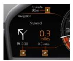
The current navigation turn-by-turn guidance will be displayed on the Driver Display if route guidance has been started using the Central Display.
