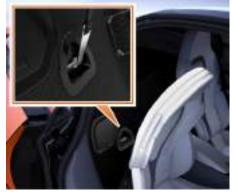
An upper tether anchorage is provided on the passenger's seat.
