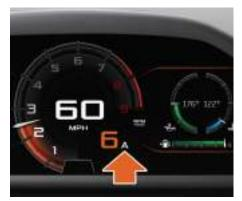
The gearbox mode indicator displays A. All gear changes occur automatically, but if a gearshift paddle is operated the gearbox will adopt a temporary manual mode. This mode will remain active for as long as the driver continues to make manual gear changes, each within an eight second period. The gearbox mode indicator displays A/M, see Gear position indicator, page 3.14.
