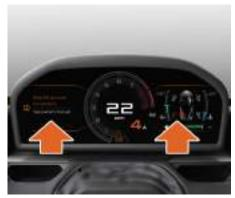
This shows the current temperature of each of the four tires. If the temperature appears in blue, the tires have not yet warmed up to optimum operating temperature. If the temperature appears in green, no action is required. If it appears in red, the safe operating temperature of the tires has been exceeded. Reduce speed or stop the vehicle until the temperatures are at a safe level, i.e. temperatures are displayed in green.
