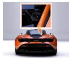
2. Unscrew the engine oil filler cap.
