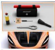
The engine cover release tool (6) is located inside the first aid kit case at the front of the luggage compartment.
