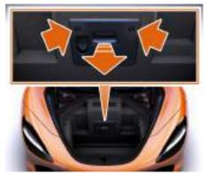
2. Remove the 2 quarter turn screws securing the top of the battery access cover.
