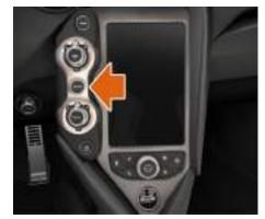
1. Press the **ACTIVE** button to switch on the Active Dynamics Panel.
