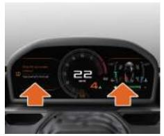
The display shows the pressures of each of the four tires. If the pressure figure appears in green, no action is required. If it appears as red text, inflate the associated tire to the correct pressure as soon as possible.
