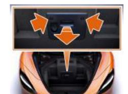
Remove the 2 quarter turn screws securing the top of the battery access cover.
