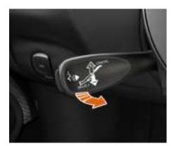
6. When the function required is selected or a setting is made, pull the stalk towards you (FORWARD) to confirm.
