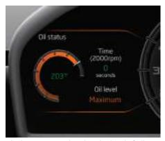
Displays a gauge showing the level of oil, together with the oil temperature.
