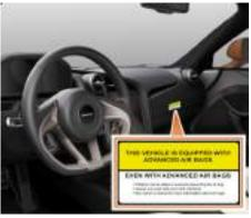
MARNING: Correct operation of the air bags can only occur if the steering wheel, the passenger's air bag cover, the knee air bag cover and the door trim are not covered.
