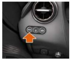
Alternatively, press the dashboard button to fully unlock and slightly open the luggage compartment.
