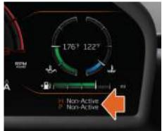
Confirmation that the ACTIVE button has not been pressed (Active Dynamics Panel is off), the handling and powertrain displays will both show Non-Active and will be displayed in white. The mode will not be implemented if all pre-conditions are not met, if the handling and powertrain mode selected is displayed. For more information on the different settings that are available, see Active dynamics control, page 2.22.
