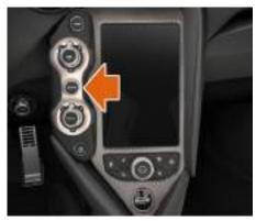
Pressing the ACTIVE button switches on the Active Dynamics Panel. This activates the Launch, Aero, ESC off, handling and powertrain controls. The ACTIVE button and handling and powertrain switches will illuminate.
