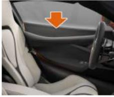
The side head air bags are located in the upper area of each door panel, and are deployed if the system determines they can offer additional protection for the head of the occupant on the side of the vehicle on which the impact occurs.
