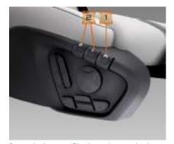
Press the button (2) where the required setting is stored, and hold until the seat, exterior mirrors and steering wheel have completed their adjustment.
