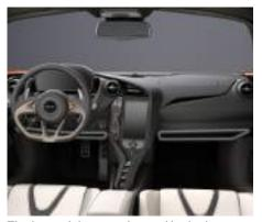
The knee air bags are located in the lower area of the dash board, and are deployed if the system determines they can offer additional protection for the knees and lower body of the occupant on the side of the vehicle on which the impact occurs.
