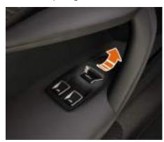
Pull door handle upwards, in direction of arrow, and push the door outwards until the opening mechanism takes over. The door will then swing outwards and upwards automatically.
