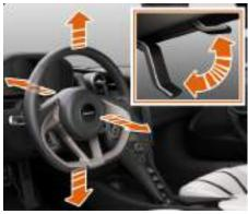
Push the lever (highlighted) downwards and position the steering wheel so that:
