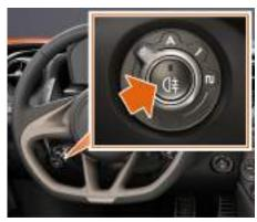
Press the rear fog lamp button in the center of the light switch.
