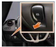
To engage the parking brake, pull the switch outwards, the red parking brake applied status light on the Driver Display illuminates.
