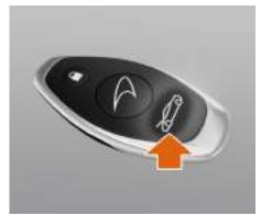
Press the luggage release button on the key fob, the luggage compartment will fully unlock and open slightly.
