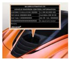
The vehicle emission label can be found permanently affixed to the intake manifold.
