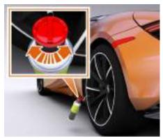
You can use the tire sealant to seal small. punctures, particularly those in the trey's tread. The tire sealant can be used at ambient temperatures down to -4°F (-20°C).
