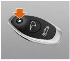
If either the doors or the luggage compartment lid are left open, or the key fob is still inside the vehicle, the horn will sound indicating mislock when an attempt to lock the vehicle is made.
