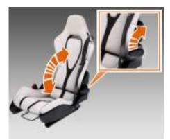
Lift the lever, move the seat backrest to the position required, and release the lever.
