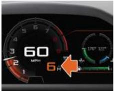
When in manual mode and driving more economically, the gear shift indicator (GSI) will illuminate when an upshift would maintain optimum economy. The GSI will not illuminate if the requested acceleration or deceleration cannot be met with a higher gear. See Economical driving, page 2.11.
