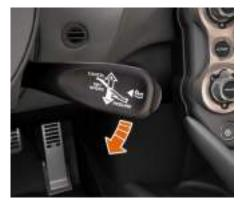
To lower the nose of the vehicle, activate the nose lift menu (see Nose lift operation, page 1.44) and then move the menu control stalk downwards.
