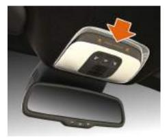
The status of the air bags is indicated by the PASSENGER AIR BAG OFF warning light on the overhead console.
