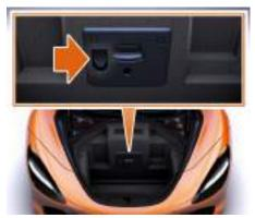
The accessory socket, located in the luggage compartment, has a maximum load rating of 20 Amps and is the only one that can be used to connect a McLaren supplied battery charger.
