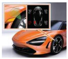
The tire pressure monitoring system warns you when the pressure drops or the temperature increases above an acceptable level in one or more of the tires.
