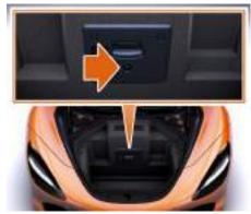
The button is located in the luggage compartment area. The button is illuminated green when the car is awake and flashes when the vehicle is locked or shut down. This operation is completely independent of ignition state. There are 2 modes to the button:
