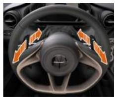
To upshift, pull the right-hand paddle towards you. To downshift pull the left-hand paddle towards you. The current gear position appears on the gear position display, see Gear position indicator, page 3.14.
