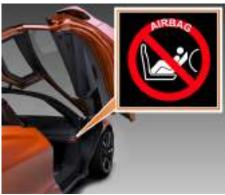
MARNING: If the PASSENGER AIR BAG OFF indicator does not illuminate, do not use a rearward facing child restraint system on the passenger seat. You may use a forward-facing child restraint system on the passenger's seat. The warning label on the passenger's side is there to remind you of this.
