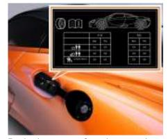
For the tire pressures for various operating conditions, see Tire pressures, page 7.8. They are also printed on a label attached to the fuel filler flap.
