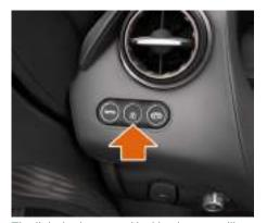
The light in the central locking button will illuminate for approximately 60 seconds after locking the vehicle, the light will continue to flash beyond this time.
