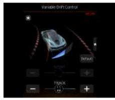
The amount of drift permitted by the ESC in Sport and Track Dynamic modes can be adjusted.
