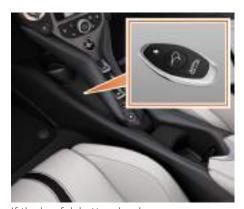
If the key fob battery has become discharged, and the engine will not start, place the key fob on the section of the cup holder housing immediately behind the switch panel.
