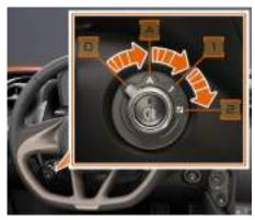
At position (0), the lights are off with the exception of daytime running lamps and tail lamps.
