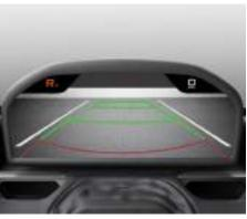
A colored grid is overlaid onto the live video feed as a guide to the proximity of visible objects to the rear of the vehicle.
