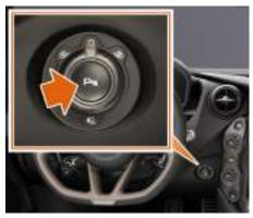
360 Park Assist will display a live video showing a 360 degree view around the vehicle in the Central Display.
