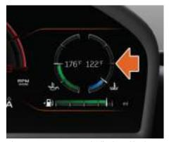
The water temperature is displayed in the form of a colored gauge on the right-hand side of the Driver Display.
