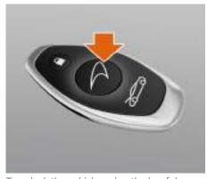
To unlock the vehicle, using the key fob, press the unlock button. The front, rear and side turn signals (market specific) flash twice and the anti-theft alarm system will be deactivated.
