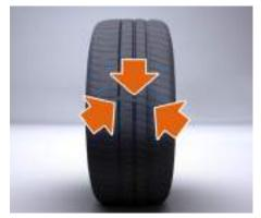
When the tread is worn to 1.6 mm, the wear indicators appear on the surface of the tread pattern, producing a continuous band of rubber across the width of the tire. Tires must be replaced as soon as the wear indicator becomes visible, or sooner if legislation dictates replacement at a greater tread depth.
