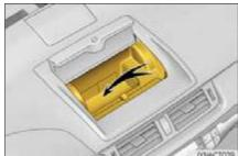
If an object has fallen down the back of the lid, the fallen object can be retrieved by removing the cover inside the auxiliary box.
