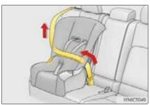
If the child restraint has a top tether strap, the top tether strap should be latched onto the top tether strap anchor.  $(\rightarrow P. 61)$
