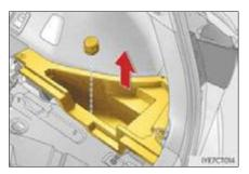
Remove the 12-volt battery maintenance cover.
