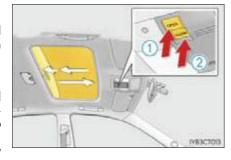
\*: Lightly press either end of the moon roof switch to stop the moon roof partway.
