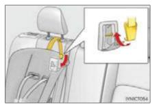
**3** Outboard only: Adjust the head restraint to the downmost position.
