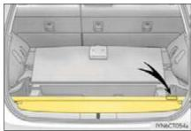
3 Fold the rear edge of the cover over, replace the side deck boards and close the center auxiliary box.
