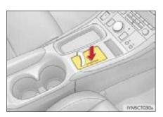
2 Open the cover and connect an iPod using an iPod cable.
