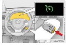
2 Accelerate or decelerate the vehicle to the desired speed, and push the lever down to set the speed.
