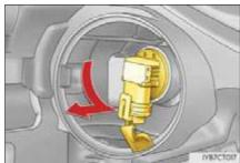
**3** Unplug the connector while pulling the lock release.
