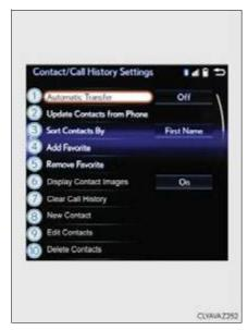
Add a new contact (PBAP incompatible Bluetooth<sup>®</sup> phones, or compatible phones with "Automatic Transfer" off)
