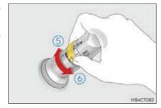
The wipers will automatically operate a couple of times after the washer squirts.
