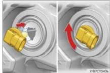
After installing the connector, shake the bulb base gently to check that it is not loose, turn the headlight high beams on once and visually confirm that no light is leaking through the mounting.
