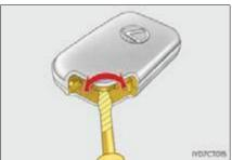
3 Remove the depleted battery.
