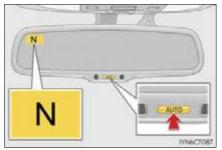
To turn the compass on or off, press the "AUTO" button for more than 3 sec-
