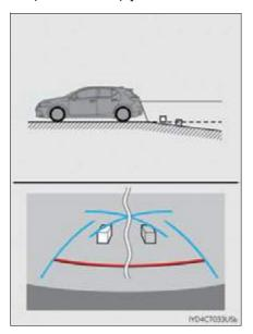
When any part of the vehicle sags due to the number of passengers or the distribution of the load, there is a margin of error between the guide lines on the screen and the actual distance/course on the road.
