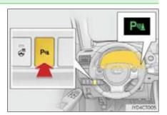
When the sensors detect an obstacle, the following displays inform the driver of the position and distance to the obstacle.
