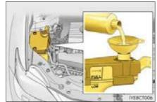
Start the hybrid system and turn the air conditioning system on to check that the radiator cooling fans operate and to check for coolant leaks from the radiator or hoses.
