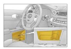
• The partition in the cup holder can also be used to store a small cup or can.
