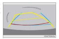
The steering wheel return points (parking assist guide lines) are displayed.
