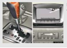
Rear view image is displayed when the shift lever is in "R".
