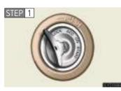
Remove the flat key from its case. Insert the key into the ignition switch.
