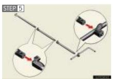
Assemble the jack handle extension as shown. Be sure to tighten each bolt securely.
