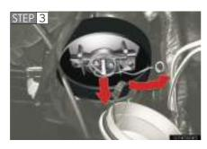
Release the wire clip and remove the light bulb.
