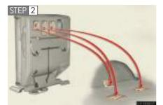
Returning third seats Reverse the steps above. Remove the lever cover and pull the lock release lever. Lift up the rear side of the seat and pull the whole seat backward.
