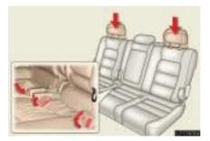
Stow the seat belt buckles and lower the head restraints to the lowest position.
