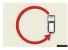
If "C" appears on the display, drive the vehicle at 5 mph (8 km/h) or less in a circle until a direction is displayed.
