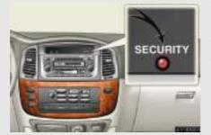
Close the doors and hood, and lock all doors. The system will be set automatically after 30 seconds.
