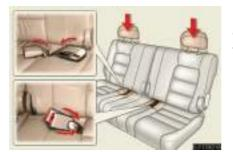
Stow the seat belts and buckles, and lower the head restraints to the lowest position.
