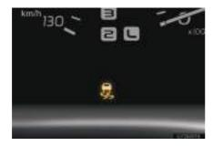
If the vehicle is in danger of slipping, the slip indicator light flashes and buzzer sounds to indicate that the VSC systems have been engaged.
