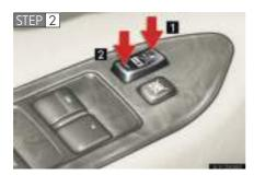
Shift the shift lever to "P" or "N", press and hold the driver's door lock switch (11 or 21) for 5 seconds then release.
