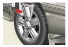
Remove the wheel ornament using the wheel nut wrench as shown.
