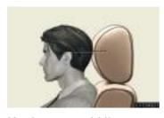
Make sure that the head restraints are adjusted so that the center of the head restraint is closest to the top of your ears.
