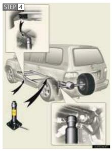
Slightly loosen the wheel nuts (one turn).
