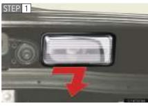
Open the back door and remove the license plate light unit.
