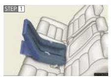
Place the child seat on the second or third outboard seat facing the rear of the vehicle.
