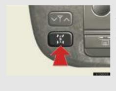
Lock the center differential when your vehicle's wheels get stuck in a ditch or when you are driving on a slippy or bumpy surface.
