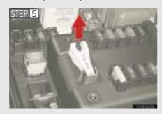
Remove the fuse with the pullout tool.
