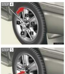
Firmly tighten each nut two or three times in the order shown in the illustration.
