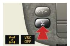
Push the center differential lock/ unlock switch to turn off VSC system.
