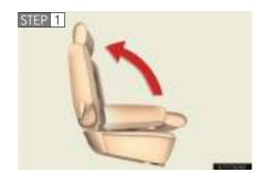
Fold the seatback forward and then back to the 1st lock position (most upright position) until it locks into place.
