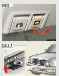
Release the lock from the inside of the vehicle to open the hood.
