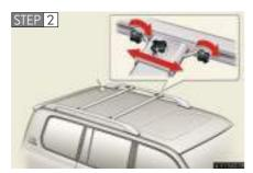
Slide the cross rails to the appropriate position for loading luggage and turn the side knobs clockwise to tighten the cross rails securely.
