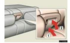
Hook the holding strap to the assist grip and secure the seat by pulling its free end.
