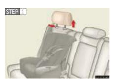
Secure the child restraint using a seat belt or lower anchors, and remove the head restraint.
