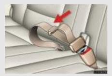
Remove excess length by pulling the free end of the belt.
