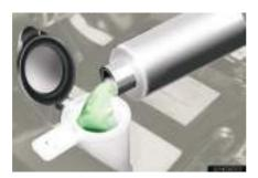
If any washer does not work or the low washer fluid warning light come on the washer tank may be empty. Add washer fluid.
