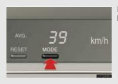
Display items can be switched by pushing the "MODE" switch.
