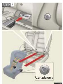
Latch the buckles onto the anchorages.
