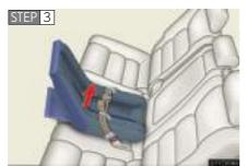
While pushing the child seat down into the seat, allow the belt to tight by pulling its free end until the child seat is securely in place.
