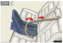
While pushing the child seat down into the seat, allow the shoulder belt to retract until the child seat is securely in place.
