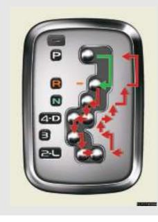
While the ignition key is in the "ON" position, depress the brake pedal and move the shift lever.
