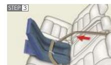
Fully extend the shoulder belt and then allow it to retract slightly in order to activate the ALR lock mode.
