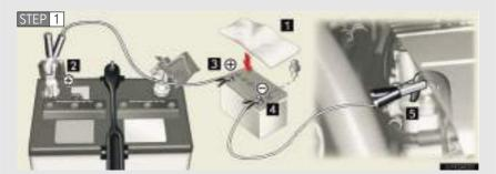
Connecting the jumper cables.
