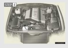
After the engine has cooled down sufficiently, check the coolant level and inspect the radiator core (radiator) for any leaks.
