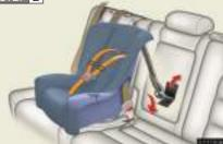
Take off the carpet, latch the hook onto the anchor bracket and tighten the top strap.
