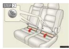
Take off the cover between the seat cushion and seatback and confirm the position of the lower anchorages below the symbol in the seatback.
