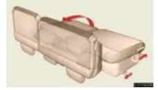
Pull the lever under the seat cushion or pull the strap on the rear end of the seat cushion and swing the whole seat forward.
