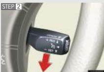
desired speed and press the lever down to set the cruise control speed.
