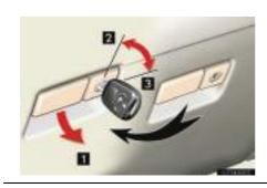
Open (pull lever)Unlock with the master keyLock with the master key
