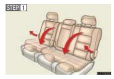
Pull the seatback angle levers and fold the second seats down.
