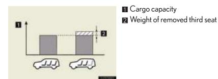
When removing the third seat, it is possible to load as much cargo as the weight of the removed seat.
