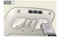
Point the remote control for the device 1 to 3 in. (25 to 75 mm) from the HomeLink $^{\textcircled{R}}$  control buttons.
