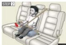
Sit the child in the child seat. Fit the seat belt to the child seat according to the manufacturer's instructions and insert the plate into the buckle. Make sure that the belt is not twisted.
