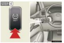
Push and hold the tire pressure warning reset switch until the tire pressure warning light blinks slowly three times.
