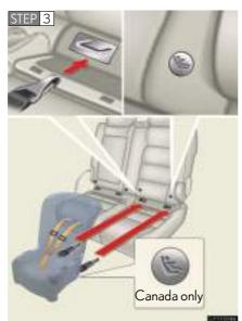
Latch the hooks of the lower straps onto the anchorages.
