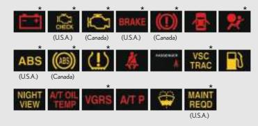
\*: These lights turn on when the ignition key is turned to the "ON" position to indicate that a system check is being performed. They will turn off after the engine is started, or after a few seconds. There may be a malfunction in a system if the lights do not come on, or if the lights do not turn off. Have the vehicle inspected by your Lexus dealer.
