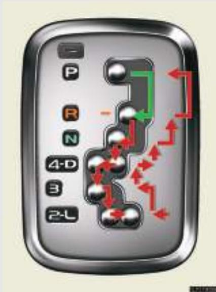
← While the ignition key is in the "ON" position, depress the brake pedal and move the shift lever.
