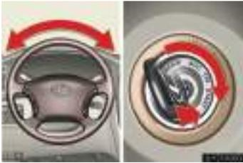
When starting the engine, the ignition switch may seem stuck in the "LOCK" position. To free it, turn the ignition key while turning the steering wheel slightly in either direction.
