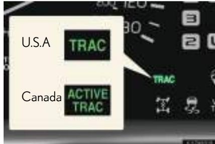
If the 4 wheels spin, the active traction control system indicator light flashes to indicate that the TRAC system have been engaged.
