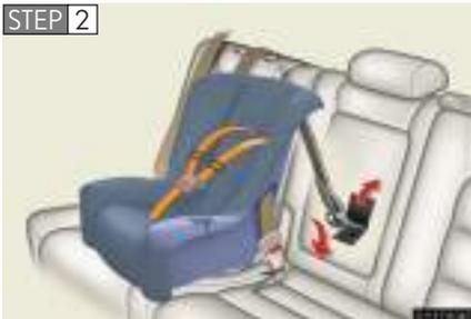
Take off the carpet, latch the hook onto the anchor bracket and tighten the top strap.
