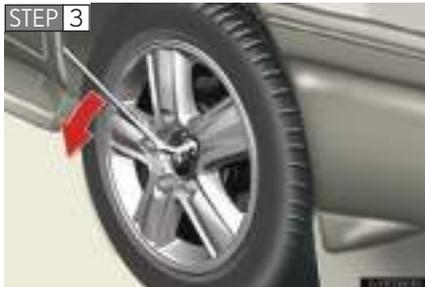
Slightly loosen the wheel nuts (one turn).
