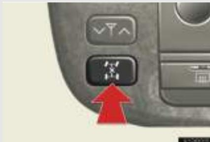
Lock the center differential when your vehicle's wheels get stuck in a ditch or when you are driving on a slippery or bumpy surface.
