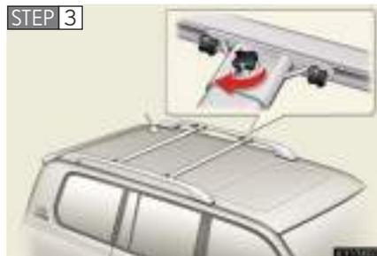
Turn the upper knobs clockwise to fix the cross rails to the appropriate length.
