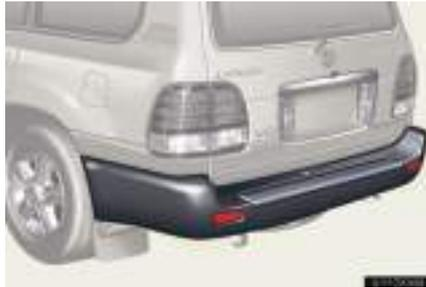
The rear step bumper is for rear end protection and easier step-up loading.
