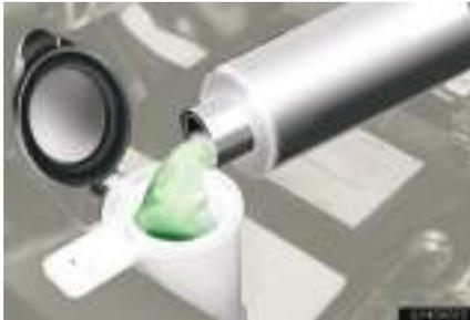
If any washer does not work or the low washer fluid warning light come on the washer tank may be empty. Add washer fluid.
