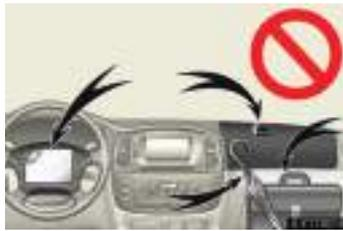
● Do not attach anything to or lean anything against areas such as the dashboard or steering wheel pad. These items can become projectiles when SRS driver and front passenger airbags deploy.
