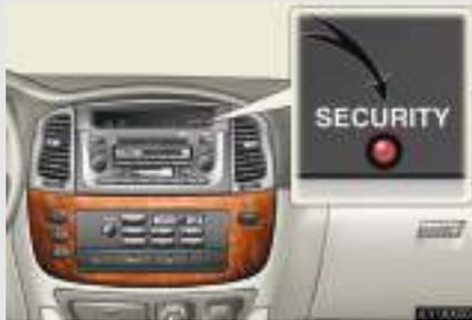
The indicator light flashes after the key has been removed from the ignition switch to indicate that the system is operating.
