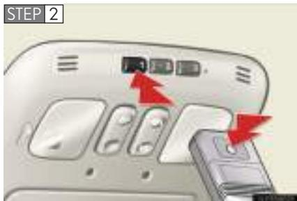
Press and hold down one of the buttons on the HomeLink<sup>®</sup> and the button on the transmitter. When the indicator light on the HomeLink<sup>®</sup> changes from a slow to a rapid flash after 20 seconds, you can release both buttons.
