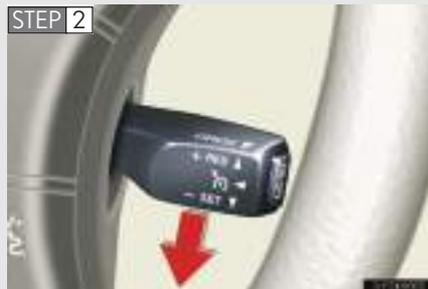
Accelerate or decelerate to the desired speed and press the lever down to set the cruise control speed.
