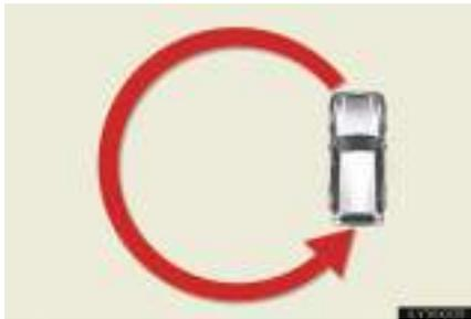
If “C” appears on the display, drive the vehicle at 5 mph (8 km/h) or less in a circle until a direction is displayed.
