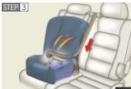
Fully extend the shoulder strap and then allow it to retract slightly into the ALR lock mode.
