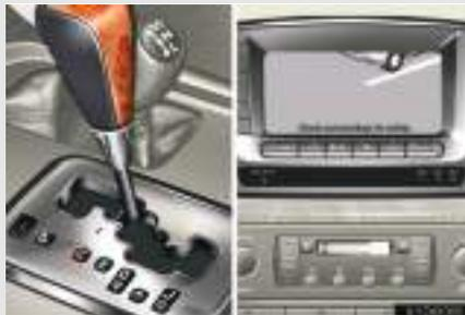
Rear view image is displayed when the shift lever is in "R".
