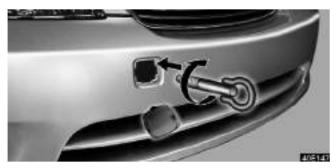
2. Use the front towing eyelet in the trunk. Secure it to the hole on the bumper by turning clockwise. (For the eyelet location, see page cccxi.)
