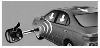
Push the "UNLOCK" button until the windows and moonroof start to move. When you release the button, the windows and moonroof stop operating.
