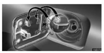
3. The removed cap can be stored on the back side of the fuel filler door.
