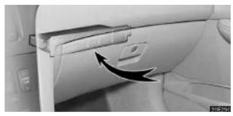
The air conditioning filter is behind the glove box.
