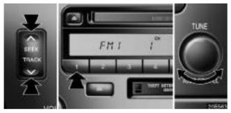
**Seek tuning:** Push the "SEEK" button. The radio will begin seeking up or down for a station of the nearest frequency and will stop on reception. Each time you push the button, the stations will be searched automatically one after another.
