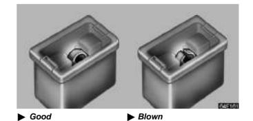
If the headlights or other electrical components do not work and the blade type fuses are O.K., check the cartridge type fuses. If any of the cartridge type fuses are blown, they must be replaced.
