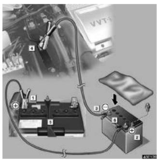
▶ 5 Discharged battery ▶ 6 Booster battery
