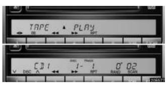
In the "TAPE" or "CD" mode, the applicable functions are shown in the lowest part of the display. Push the switch just below to turn on each function.
