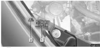
I Vertical movement adjusting bolt 1
