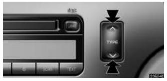
When you push the "TYPE" button while tuned to FM broadcasts, the current program type appears on the display.
