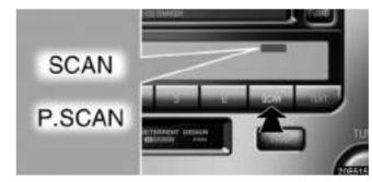
**To scan all the frequencies:** Push the "SCAN" button briefly. "SCAN" appears on the display. The radio will find the next station up the band, stay there for a few seconds, and then scan again. To select a station, push the "SCAN" button a second time.
