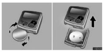
3. Open and remove the battery case cover using a coin.
