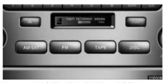
Push the "AM-SAT", "FM", "TAPE" or "DISC" button to turn on that mode. The selected mode turns on directly.
