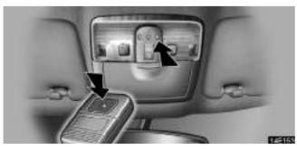
3. Simultaneously press and hold the hand-held garage transmitter button along with the selected HomeLink<sup>®</sup> button.
