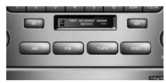
Push the "AM", "FM", "TAPE" or "DISC" button to turn on that mode. The selected mode turns on directly.
