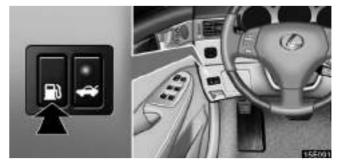
1. To open the fuel filler door, push the switch.
