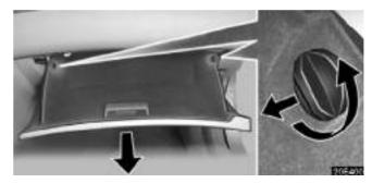
2. Remove the 2 pins installed on the upper part of the glove box and lower the glove box.
