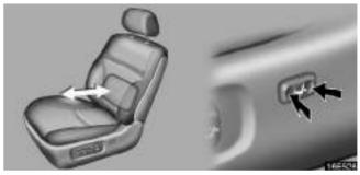
Push the control switch on either side.
