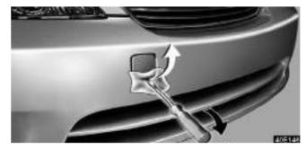
1. Remove the front towing eyelet cover on the front bumper using a flathead screwdriver. To protect the bodywork, place a piece of rag over the cover.
