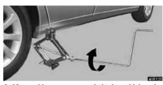
6. After making sure no one is in the vehicle, raise it high enough so that the spare tire can be installed.
