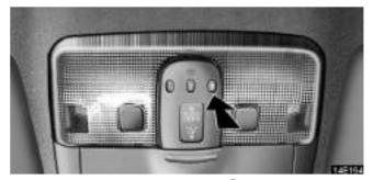
5. Test the operation of the HomeLink<sup>®</sup> by pressing the newly programmed button. If programming a garage door opener, check to see if the garage door opens and closes.
