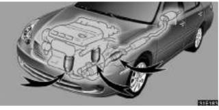
The three–way catalytic converters are emission control devices installed in the exhaust system.
