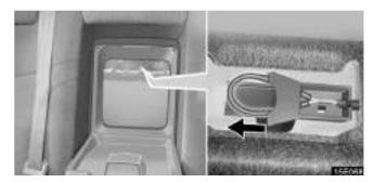
2. Pull the loop of wire to unlock the trunk lid.
