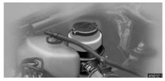
Check the fluid level through the reservoir. If necessary, add automatic transmission fluid DEXRON<sup>®</sup>II or III.
