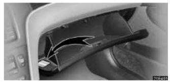
The air conditioning filter information label is placed in the glove box as shown and indicates that a filter has been installed.
