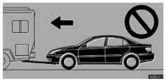
Your vehicle is not designed to be dinghy towed (with four wheels on the ground) behind a motorhome.
