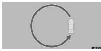
Drive the vehicle slowly (at 8 km/h [5 mph] or lower) in a circle until the direction is displayed. If there is not enough space to drive in a circle, drive around the block until the direction is displayed.
