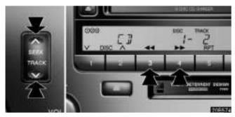
"TRACK" button: Use for direct access to a desired track.
