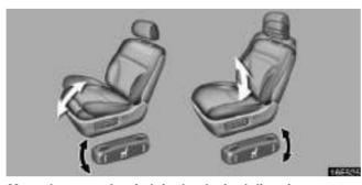
Move the control switch in the desired direction. Releasing the switch will stop the seat cushion in that position. Adjusting lumbar support (driver's seat only)
