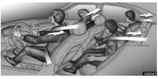
Both front seats and the two outboard rear seats are equipped with seat belt pretensioners and are designed to be activated in response to a severe frontal impact.
