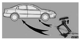
5. Position the jack at the jack points as shown. Rotate the load rest  $90^{\circ}$  from storage position to lifting position.
