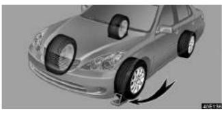
3. Block the wheel diagonally opposite the flat tire to keep the vehicle from rolling when it is jacked up.
