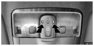
To erase all previously programmed codes at one time, press and hold down the 2 outside buttons for 20 seconds until the indicator light flashes.
