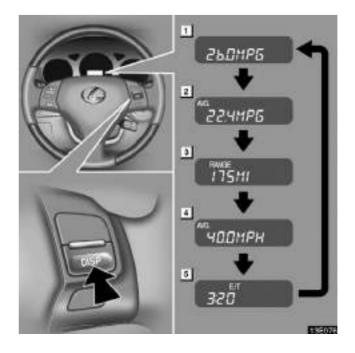
The following information is displayed in the instrument cluster when you push the "DISP" button with the ignition switch turned on.
