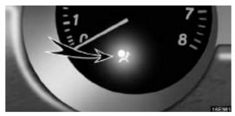
This indicator comes on when the ignition key is turned to the "ON" position. It goes off after about 6 seconds. This means the SRS front airbags are operating properly.
