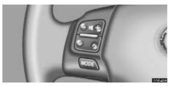
The switches are installed on the left side of the steering wheel.
