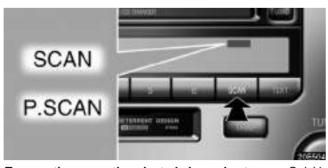
**To scan the currently selected channel category:** Quickly push and release the "SCAN" button. "SCAN" appears on the display. The radio will find the next channel in the same channel category up the band, stay there for 5 seconds, and then scan again. To stop scanning, push this button again.
