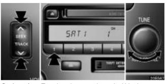
**Seek tuning:** To select the next channel within the current channel category, push the " $\Lambda$ " or " $\vee$ " side of the "SEEK/TRACK" button. Repeat until a desired channel is found.
