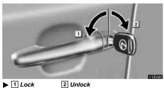
Turn the key towards the front of the vehicle to lock and towards the back to unlock.
