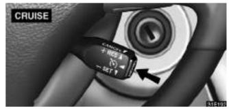
To turn the cruise control on, press the "ON–OFF" button. The "CRUISE" indicator light in the instrument cluster will come on to indicate that the cruise control is operational. Pressing the "ON–OFF" button again turns the system off.
