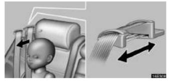
The seat belt comfort guides are installed on the outboard rear seats to relieve uncomfortableness from the shoulder belt when it is applied closer to a child's neck (at the age of 10 or so), by pulling the shoulder belt a little forward.
