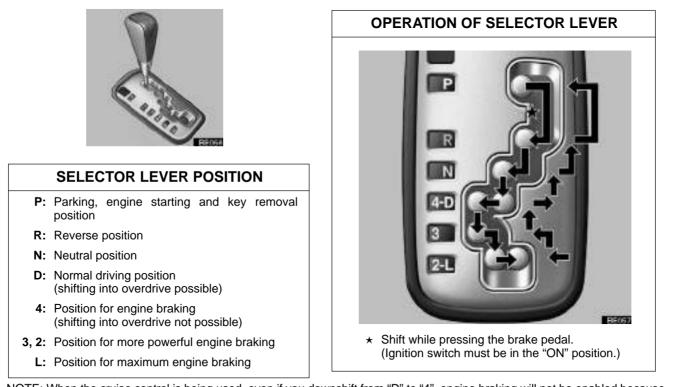
NOTE: When the cruise control is being used, even if you downshift from "D" to "4", engine braking will not be enabled because the cruise control is not cancelled. For the operation to decrease the vehicle speed, see page cclxxi.
