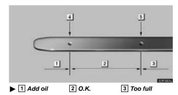
4. Pull the dipstick out and look at the oil level while holding a rag under the end. If it is between the low level mark ( $\boxed{4}$ ) and the full level mark ( $\boxed{5}$ ), it is O.K.
