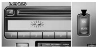
When the audio sound becomes difficult to be heard due to road noise, wind noise, etc. during driving, the system adjusts to the optimum volume and tone quality according to the noise level. While the Automatic Sound Levelizer is on, "ASL" appears on the display.
