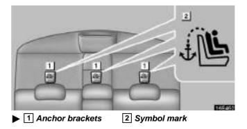
Use the anchor bracket on the package tray behind the rear seat to attach the top strap.
