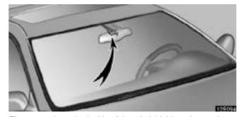
The sensor is on the inside of the windshield as shown above.
