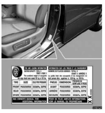
The recommended cold tire inflation pressures, tire sizes and the combined weight of occupants and cargo (vehicle capacity weight) are described on pageccclxv, ccclxvi and cdxiii. They are also described on the tire and loading information label as shown.
