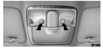
To turn on the personal light, push the switch. To turn it off, push the switch again.
