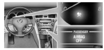
The SRS warning light and "AIRBAG OFF" indicator light will be illuminated if there is a malfunction in the front passenger occupant classification system.
