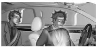
The SRS (Supplemental Restraint System) side airbags and curtain shield airbags are designed to provide further protection for the driver, front passenger and rear outboard passengers in addition to the primary safety protection provided by the seat belts.
