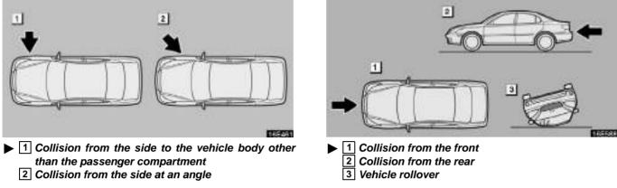
The SRS side airbag and curtain shield airbag system may not activate if the vehicle is subjected to a collision from the side at certain angles, or a collision to the side of the vehicle body other than the passenger compartment as shown in the illustration.
