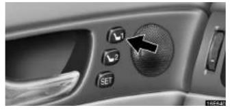
When you push button "1" or "2", the driving position will be automatically adjusted to the position recorded for that button.
