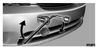
3. Tighten the front towing eyelet securely by a wheel nut wrench.
