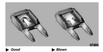
a. Look carefully at the fuse. If the thin wire is broken, the fuse has blown. If you are not sure or if it is too dark to see, try replacing the suspected fuse with one of the same value that you know is good.
