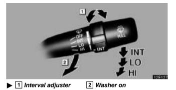
To turn the wipers on, move the lever down until you reach the desired speed setting.
