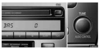
Each time you push the "AUDIO CONTROL" knob, the display changes as in the following. To adjust the tone and balance or turn on or off the Automatic Sound Levelizer, turn the knob.
