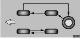
To equalize tire wear and help extend tire life, Lexus recommends that you rotate your tires according to the maintenance schedule. (For scheduled maintenance information, please refer to the "Owner's Manual Supplement/Scheduled Maintenance".) However, the most appropriate timing for tire rotation may vary according to your driving habits and road surface conditions.
