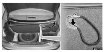
1. Lift up the deck board and hang the deck board hook on the right hinge of the trunk lid.
