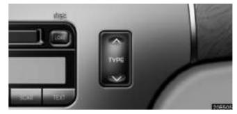
When you push the " $\Lambda$ " or " $\vee$ " side of the "TYPE" button while receiving a XM channel.
