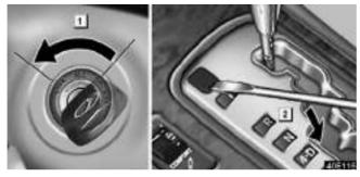
If you cannot shift the selector lever out of "P" position to other positions even though the brake pedal is depressed, use the shift lock override button as follows:
