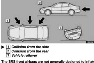
The SRS front airbags are not generally designed to inflate if the vehicle is involved in a side or rear collision, if it rolls over, or if it is involved in a low-speed frontal collision. But, whenever a collision of any type causes sufficient forward deceleration of the vehicle, deployment of the SRS front airbags may occur.
