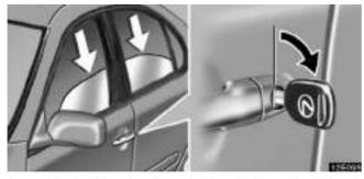
Insert the ignition key into the key hole on the driver's door.
