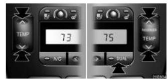
2. Use the "TEMP" or "PASSENGER TEMP" button to set the desired temperature.
