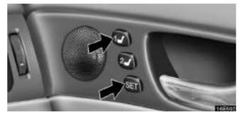
When you push button "1" or "2", the seat position will be automatically adjusted to the position recorded for that button.
