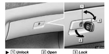
To open the glove box door, pull the lever. To lock the glove box door, insert the master key and turn it clockwise.
