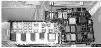
► Engine compartment 1 Pull-out tool 2 Spare fuses
