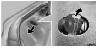
Remove the cover and pull up the manual lever in the trunk.
