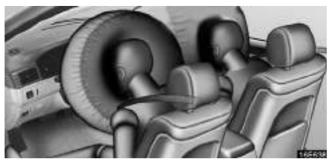
The SRS (Supplemental Restraint System) front airbags are designed to provide further protection for the driver and front passenger in addition to the primary safety protection provided by the seat belts.
