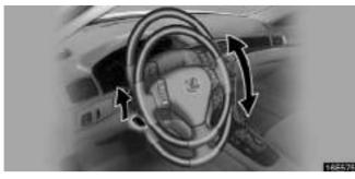
To change the steering wheel angle, hold the steering wheel, pull up the lock release lever, tilt the steering wheel to the desired angle and release the lever.
