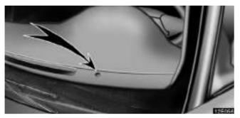
The automatic light control sensor is on the top of the driver's side instrument panel.
