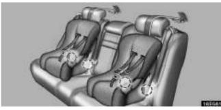
Lower anchorages for the child restraint systems complying with the FMVSS225 or CMVSS210.2 specifications are installed in the rear seat.
