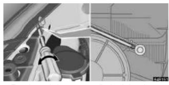
2. Turn the vertical movement adjusting bolt 2 the same number of turns and in the same direction as step 1 using a Phillips-head screwdriver.
