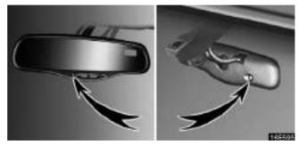
To ensure correct functioning of anti-glare mirror sensors located on both sides of the mirror, do not touch or cover the sensors with your finger or a piece of cloth, etc.
