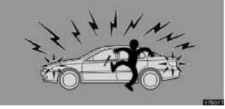
To deter theft of the vehicle, this system is designed to sound an alarm if any of the doors, trunk or hood is forcibly unlocked or the battery terminal is disconnected and then reconnected while the vehicle is locked.
