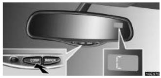
To rectify the compass, stop the vehicle and push and hold the "COMP" switch until "C" appears on the display.
