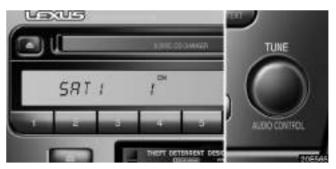
Turn the "TUNE" knob clockwise to step up the channel. Turn the knob counterclockwise to step down the channel.
