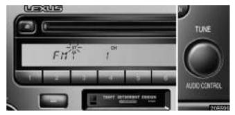
Turn this knob to the right to step up the station band or to the left to step down.
