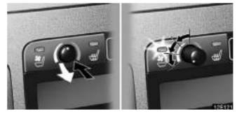
To turn on the seat ventilator, push the knob to pop it out and then turn the knob counterclockwise. The indicator light (green) comes on.
