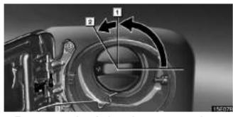
2. To remove the fuel tank cap, turn the cap counterclockwise by 90 degrees (to the pressure point
