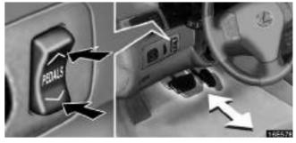
To adjust the position of the accelerator and brake pedals, push the switch.
