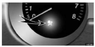
This indicator comes on when the ignition key is turned to the "ON" position. It goes off after about 6 seconds. This means the SRS side airbags and curtain shield airbags are operating properly.
