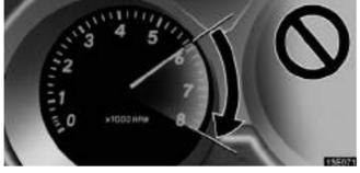
The tachometer indicates engine speed in thousands of rpm (revolutions per minute). Use it while driving to prevent engine over-revving.
