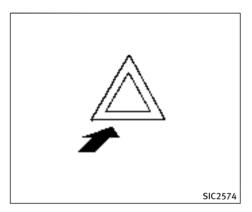
Push the switch on to warn other drivers when you must stop or park under emergency conditions. All turn signal lights will flash.
