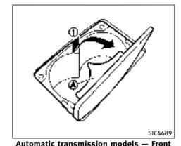
To open the cup holder, push the lid (1). The flap (A) will be folded down when inserting a large container.
