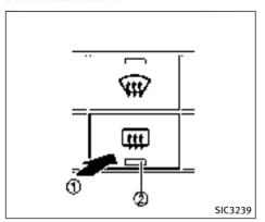
To defog/defrost the rear window glass and outside mirrors, start the engine and push the switch ① on. The indicator light ② will come on. Push the switch again to turn the defroster off.
