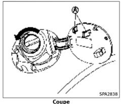
Turn the fuel-filler cap counterclockwise to remove. To tighten, turn the cap clockwise until a single click is heard. Put the fuelfiller cap on the cap holder (A) while refueling.
