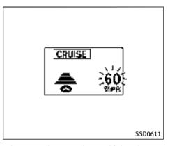
When passing another vehicle, the set speed indicator will flash when the vehicle speed exceeds the set speed. The vehicle detect indicator will turn off when the area ahead of the vehicle is open. When the pedal is released, the vehicle will return to the previously set speed.
