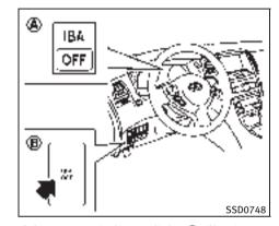
If the IBA OFF indicator light (A) illuminates with a beep sound, pull off the road to a safe location, stop the vehicle and turn the engine off. Check to see if the sensor window is dirty. If the sensor window is dirty, clean it with a soft cloth and restart the engine. If the sensor window is not dirty, restart the engine. If the IBA OFF indicator light continues to illuminate even if the IBA system is turned on with the IBA OFF switch (B), have the system checked by an INFINITI dealer.
