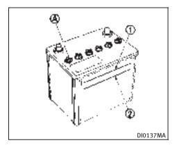
Check the fluid level in each cell (Remove the battery cover if it is necessary). It should be between the UPPER LEVEL (1) and LOWER LEVEL ② lines.
