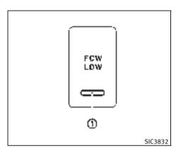
The Forward Collision Warning (FCW) system will sound a warning chime and blink the forward collision warning light (orange) to alert the driver if the vehicle is traveling close to a vehicle ahead.
