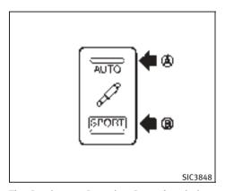
The Continuous Damping Control optimizes damping force and helps minimize the movement of the vehicle body. It helps stable driving when the vehicle moves up and down on large rolling roads or when the vehicle body leans during cornering with a high centrifugal force.
