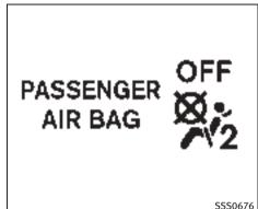
7. If the booster seat is installed in the front passenger seat, push the ignition switch to the ON position. The front passenger air bag status light == may or may not illuminate depending on the size of the child and the type of booster seat used. (See "Front passenger air bag and status light" later in this section.)
