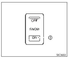
For driving or starting the vehicle on snowy roads or slippery areas, turn on the SNOW mode switch. The indicator light ① on the switch will illuminate. When the SNOW mode is activated, engine output is controlled to avoid wheel spin.
