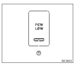
The Lane Departure Warning (LDW) system will sound a warning chime and blink the lane departure warning light (orange) to alert the driver if the vehicle is traveling close to either the left or the right of a traveling lane with detectable lane markers.
