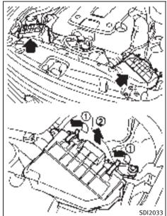
Remove the retainers  $\widehat{\mbox{\em 1}}$  as illustrated and pull out the filter element  $\widehat{\mbox{\em 2}}$ .
